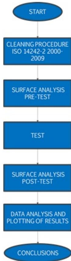
Figure 3.37: workflow of experimental procedures.
