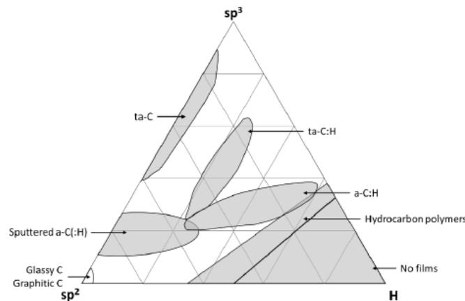
Figure 3.25: Ternary phase diagram for DLC formation with respect to  $sp^2$ ,  $sp^3$  and hydrogen content<sup>C</sup>
