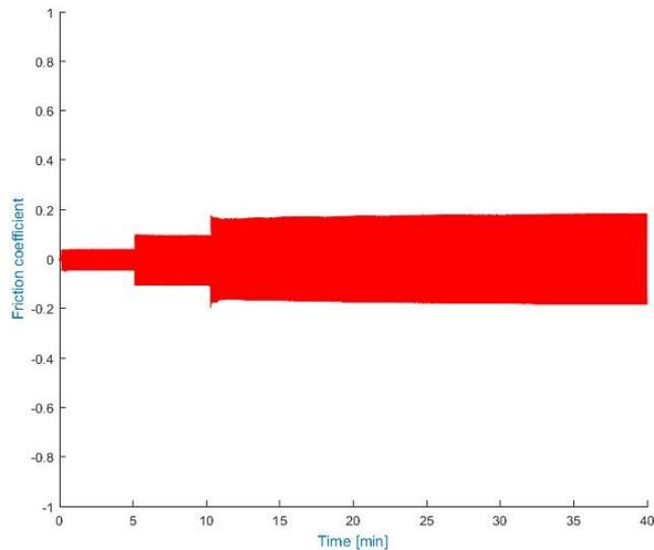
Figure 4.17: DLC(Ti-6Al-4V) coefficient of friction protocol 2
