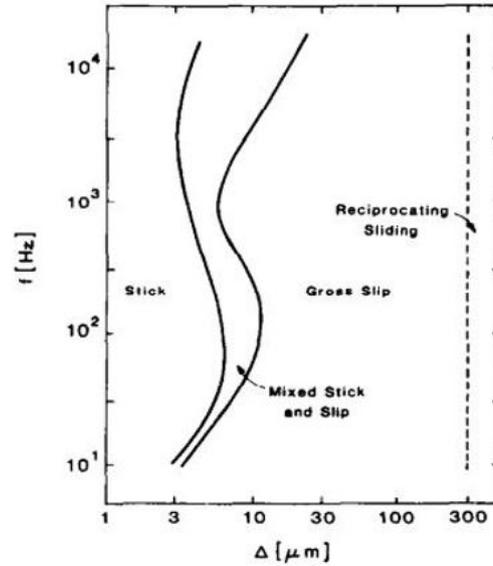
Figure 3.6: Fretting map  $f[\text{Hz}]$  &  $\Delta[\mu\text{m}]^x$
