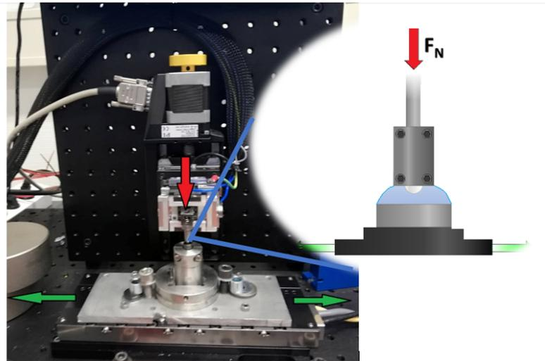
Figure 3.27: Ducom Microforce Biotribometer.
