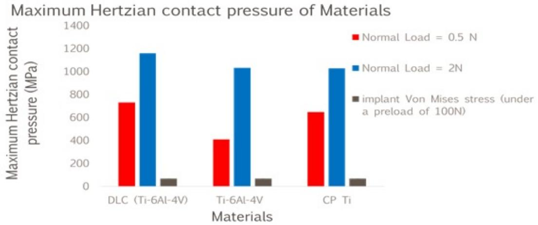
Figure 3.35: Hertzian contact pressure of the materials used
