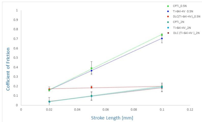
Figure 4.19: Comparison of all the coefficients of friction of both protocols
