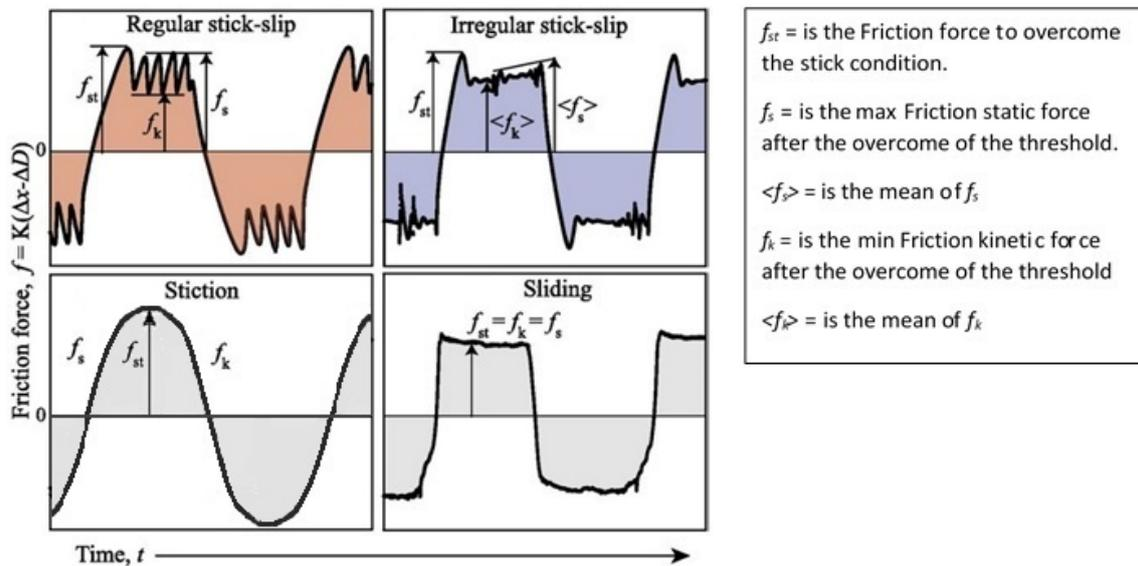
Figure 4.21: Comparison of different signal morphologies
