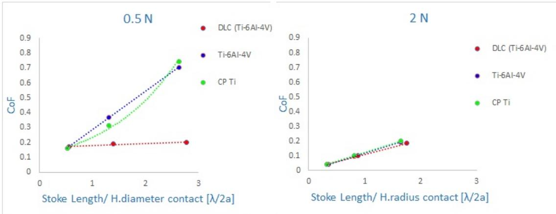
Figure 4.20: Comparison of different materials, putting in comparison coefficients of frictions vs stroke length/ hertzian contact diameter, of both the normal loads applied
