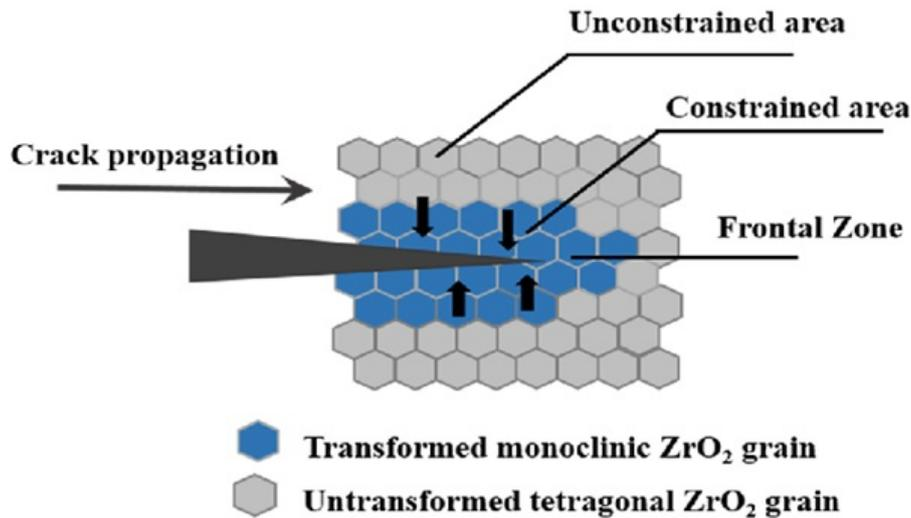
Figure 3.21: transformation t to m during a crack propagation.
