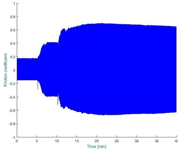
Figure 4.12: Ti-6Al-4V coefficient of friction protocol 1
