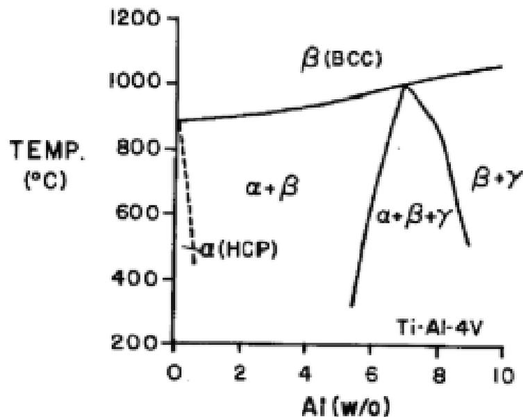
Figure 3.24: Ti-6Al-4V phase diagram.
