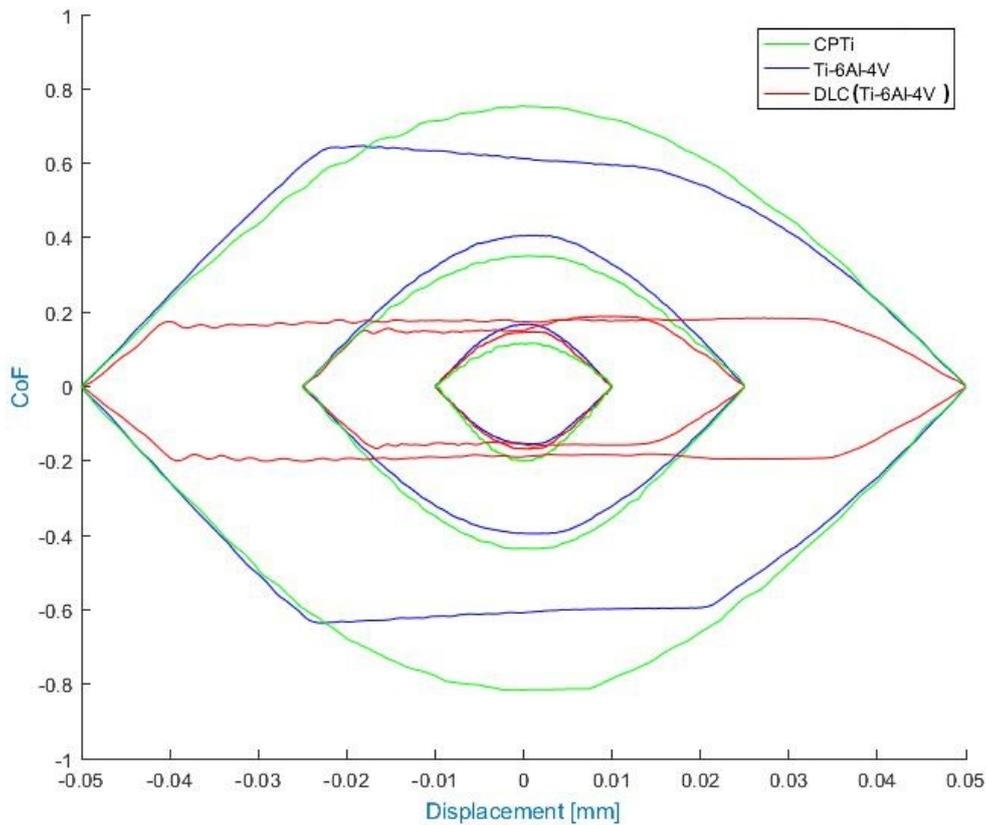
Figure 4.28: fretting loops of the different materials of the protocol 1 (5th cycle before the change from 0.02 to 0.05, 5th cycle before the change from 0.05 to 0.1, 5th cycle before the end of the test)
