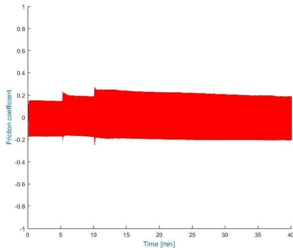
Figure 4.13: DLC(Ti-6Al-4V) coefficient of friction protocol 1
