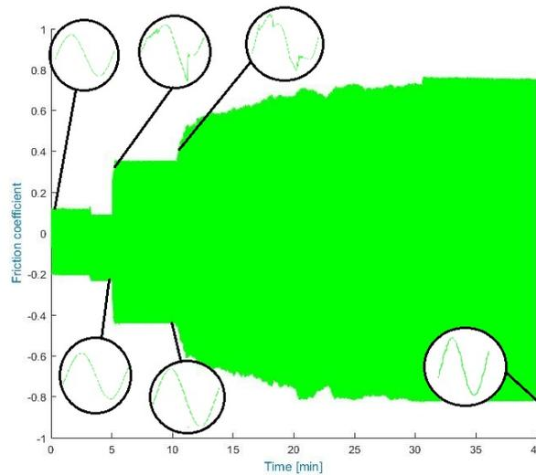
Figure 4.22: CPTi coefficient of friction signal morphology protocol 1
