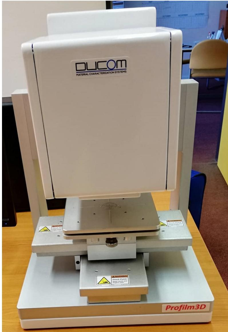
Figure 3.29: light profilometer (profilm 3D Filmetrics)
