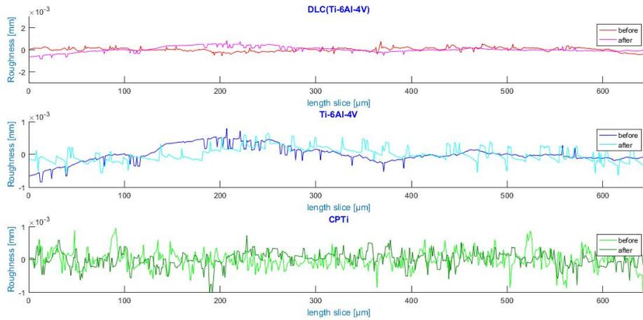
Figure 4.7: profile comparison between before and after the test 2
