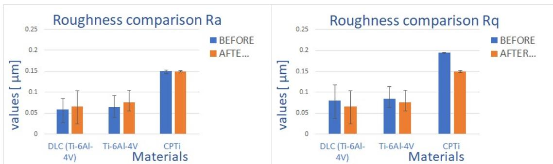
Figure 4.4: roughness values comparison between before and after the test 1, ISO 4287  $R_a$  and  $R_q$
