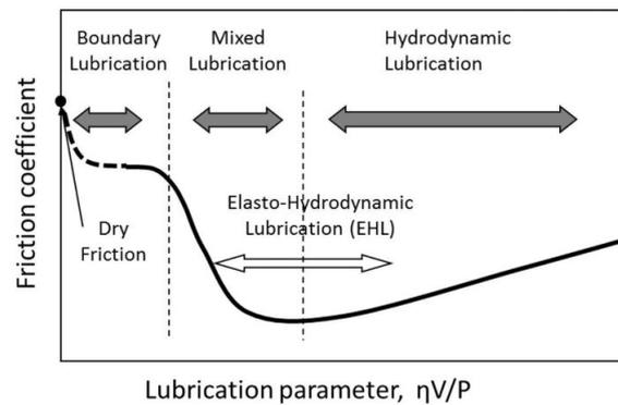
Figure 1.15: Representation of The Stribeck-curve of the different lubrication regimes
