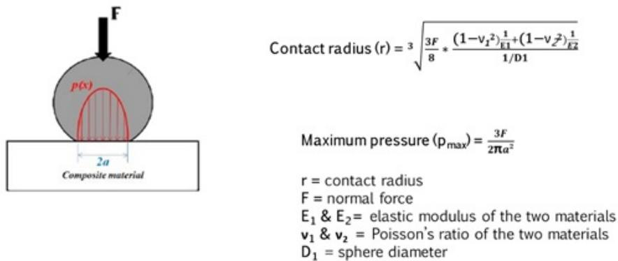
Figure 3.33: Hertzian contact model and formulas
