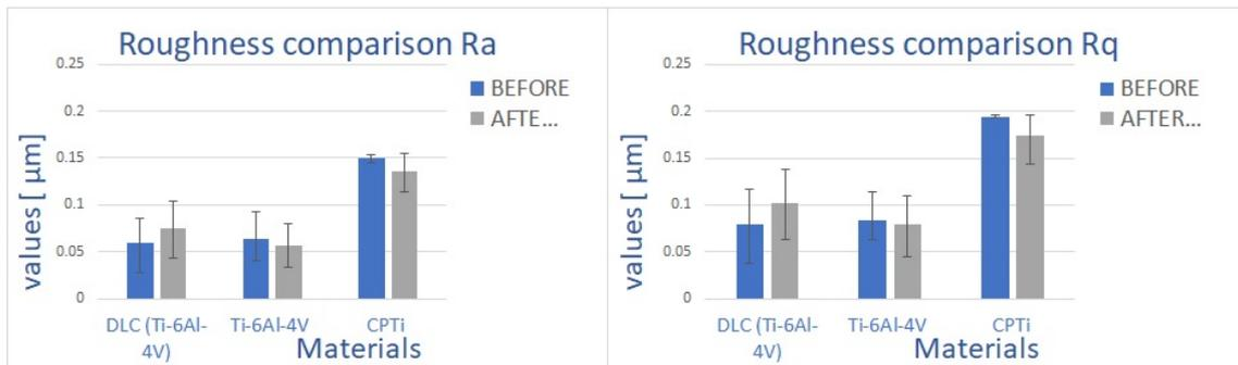
Figure 4.8: roughness values comparison between before and after the test 2, ISO 4287  $R_a$  and  $R_q$
