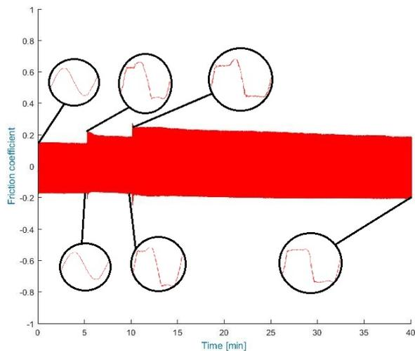
Figure 4.24: DLC (Ti-6Al-4V) coefficient of friction signal morphology protocol 1
