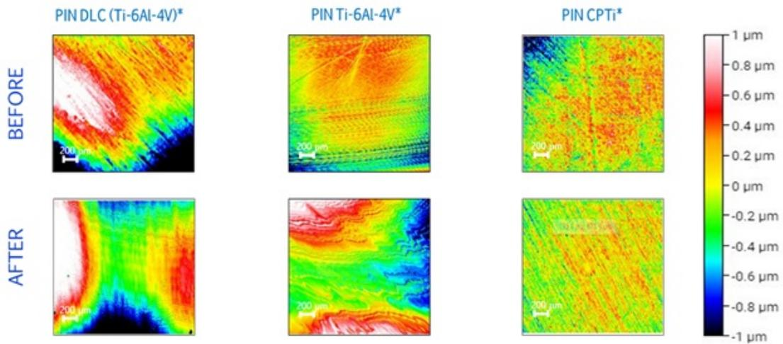
Figure 4.6: interferometer comparison between before and after the test 2
