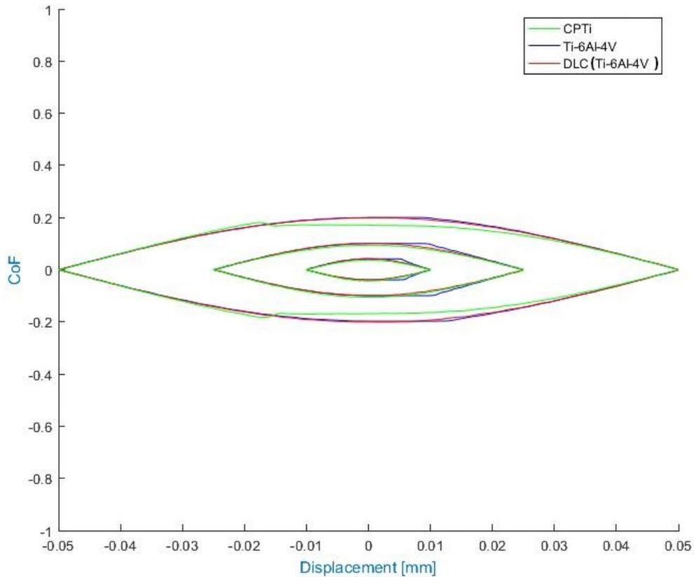
Figure 4.29: fretting loops of the different materials of the protocol 2 (5th cycle before the change from 0.02 to 0.05, 5th cycle before the change from 0.05 to 0.1, 5th cycle before the end of the test)
