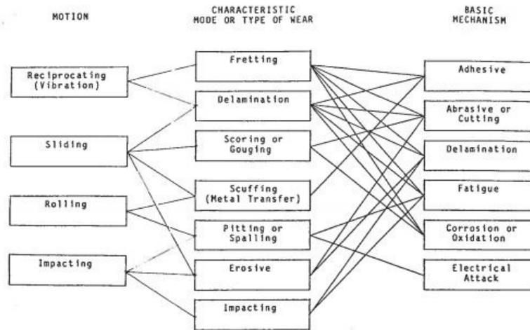
Figure 1.13: the relationship between motion, mode, and type of wear, and basic mechanism of wear by Ko
