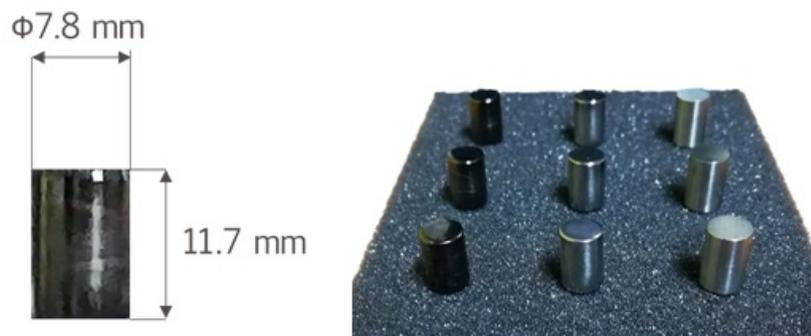
Figure 3.22: Ti-6Al-4V and DLC(Ti-6Al-4V) pins.
