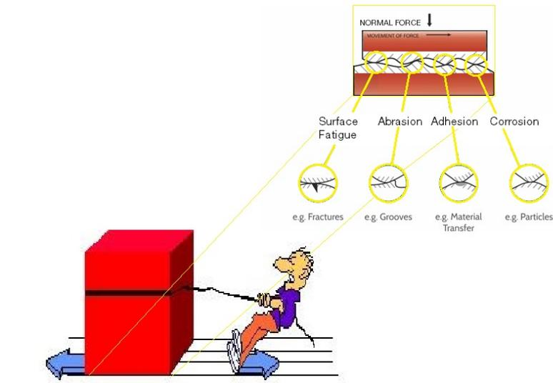
Figure 1.12: Representation of the different types of wear
