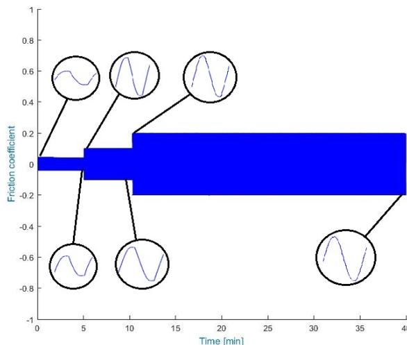
Figure 4.26: Ti-6Al-4V coefficient of friction signal morphology protocol 2
