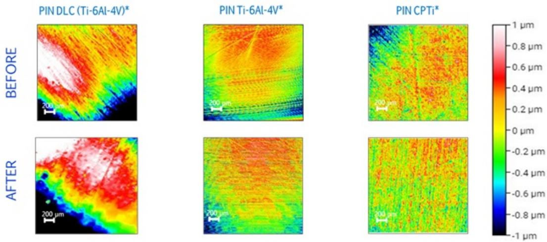
Figure 4.2: interferometer comparison between before and after the test 1
