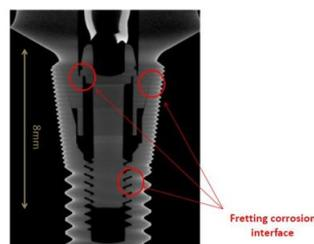
Figure 3.1: fretting corrosion in the fixture/abutment interface
