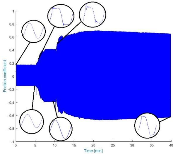
Figure 4.23: Ti-6Al-4V coefficient of friction signal morphology protocol 1
