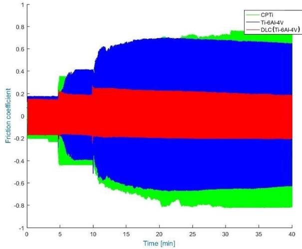
Figure 4.14: Comparison of the coefficients of friction protocol 1
