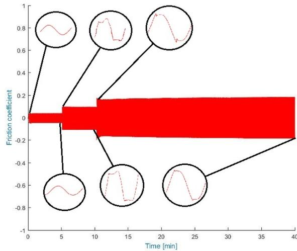
Figure 4.27: DLC (Ti-6Al-4V) coefficient of friction signal morphology protocol 2
