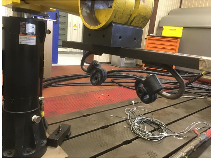
**Figure 5.4:** *The same disposition and shape of vehicle counter-brackets is cloned for the bench simulation. These features are rigidly connected to actuator arm tips through bolts*
