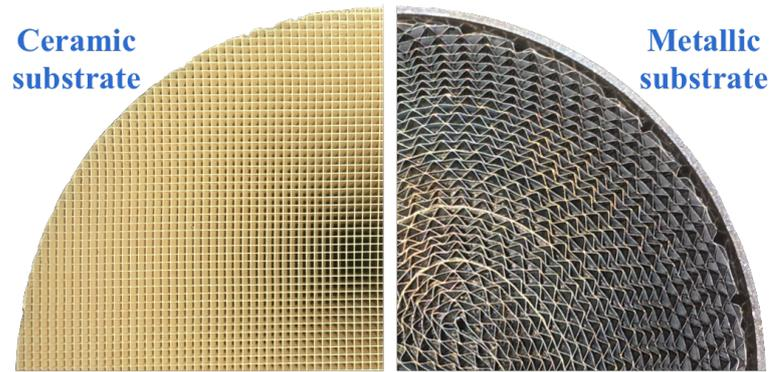
**Figure 2.4:** *Internal structure on converters substrates: the thin ceramic walls or metallic foil are not suitable to withstand mechanical stresses*
