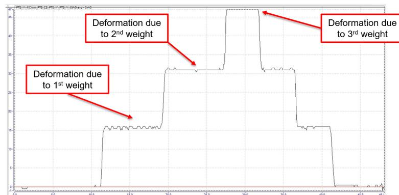
**Figure 3.10:** *Strain time history during the calibration: the symmetry between the loading and unloading phases indicates the correctness of the readings*
