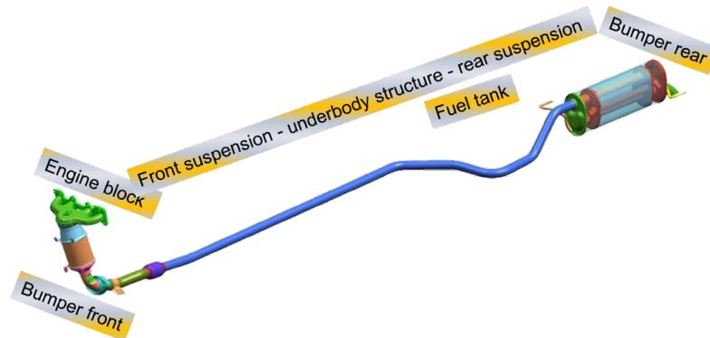
**Figure 1.4:** Scheme of the main constraints on the design of the exhaust line in a vehicle under-body
