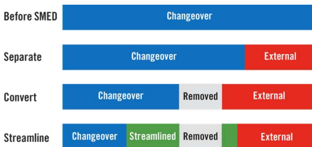
Figure 4.1- Graphical representation of the four steps proposed by the SMED methodology
