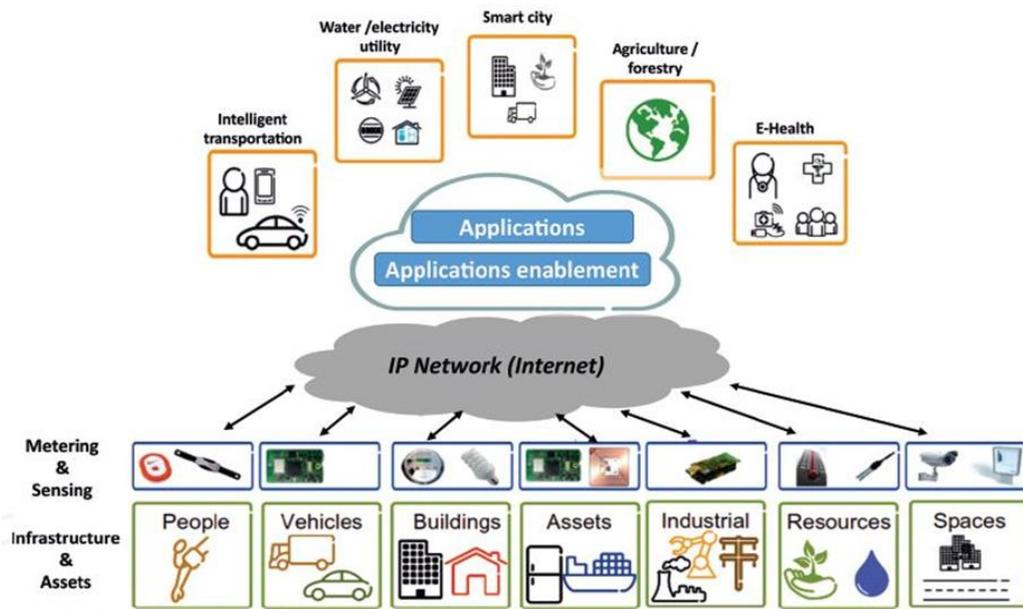
Figure 7: Overview on IoT architecture including different application areas by Haidine, Abdelfatteh, et al. (2016)
