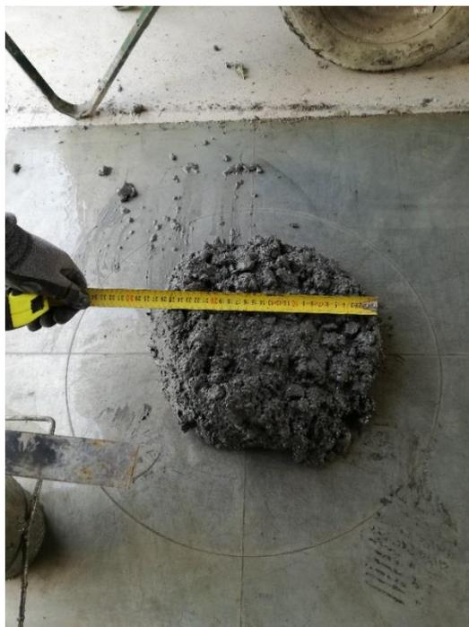
*Figura 103: “slump flow”*
