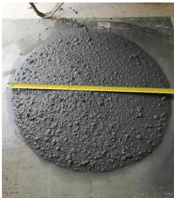
Figura 107: “slump flow”
