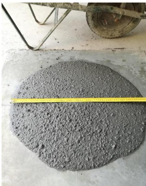
Figura 114: “slump flow”
