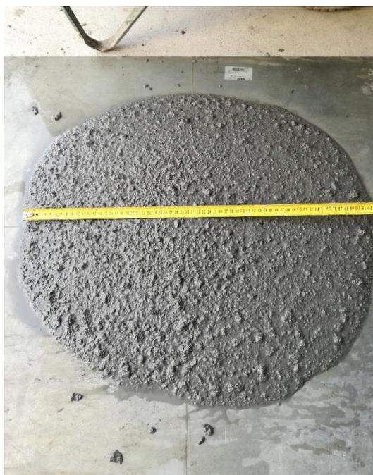
Figura 111: “slump flow”
