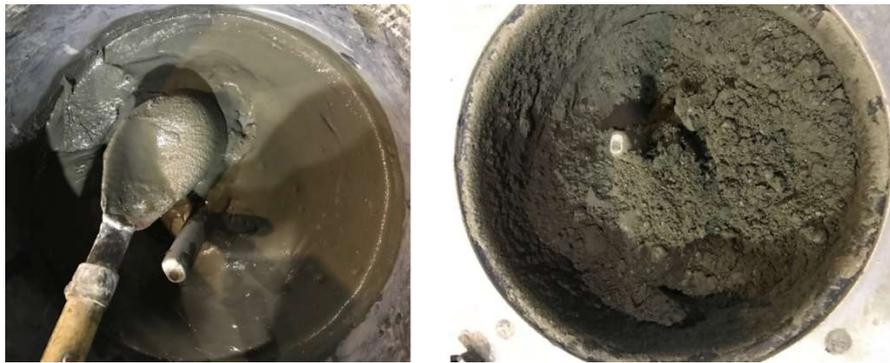
Figure 3.8 - Example of mixes with a not appropriate workability
