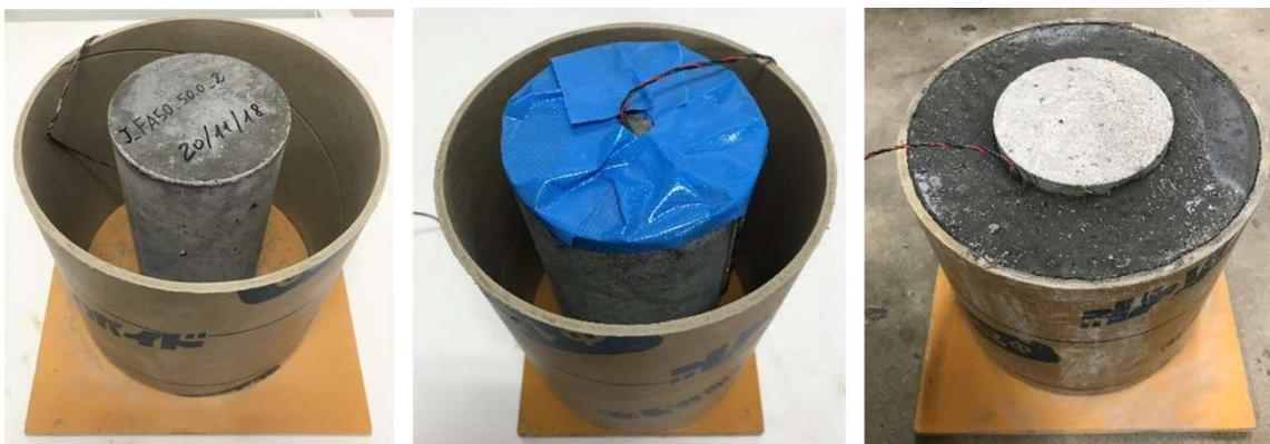
Figure 3.26 - Preparation and casting of jacket
