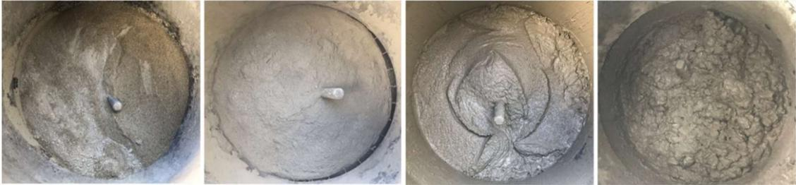
Figure 3.18 - Mixing phases for concrete cores
