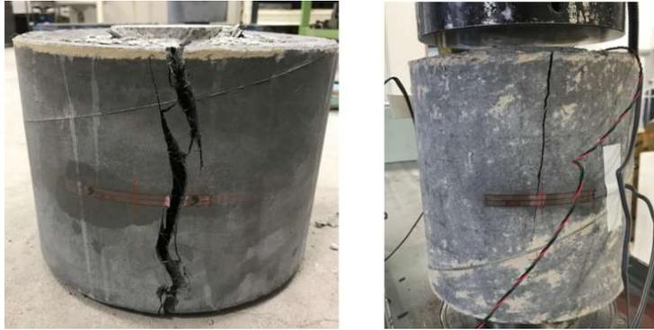
Figure 4.23 - Strain gauges breakage
