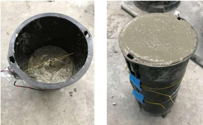
Figure 3.21 - Casting of concrete cores
