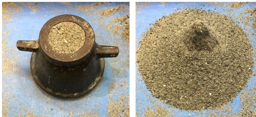
Figure 3.13 - Abram cone to determine the saturated surface dry (SSD)
