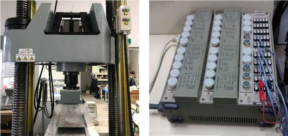
Figure 3.34 - Universal testing machine (UTM) used for the compressive test
