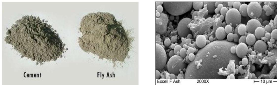
Figure 2.15 - (a) Cement and Fly Ash powders comparison; (b) Finer and more spherical Fly Ash particles than Cement
