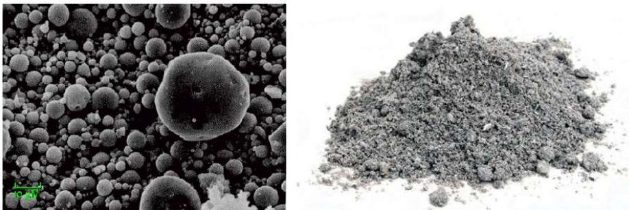
Figure 2.6 - Fly ash particles
