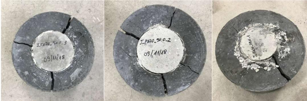
Figure 6.23 - Failure patterns: top view
