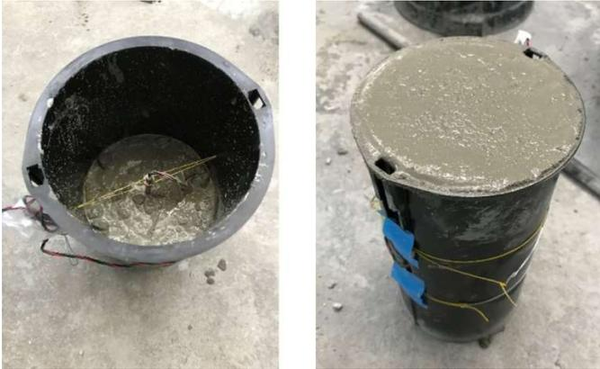
Figure 3.21 - Casting of concrete cores
