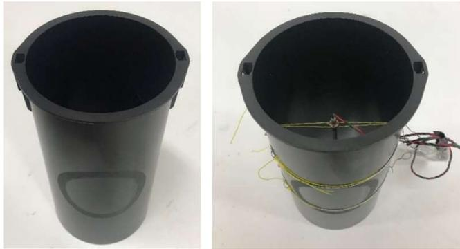
Figure 3.11 - Plastic molds used for core casting
