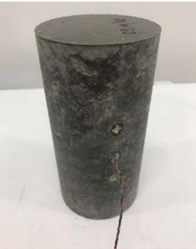
Figure 3.22 - Concrete core after removing the mold
