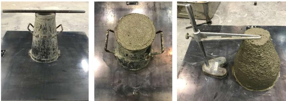
Figure 3.19 - Slump test: equipment and measurement
