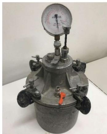
Figure 3.20 - Device for measurement of air content
