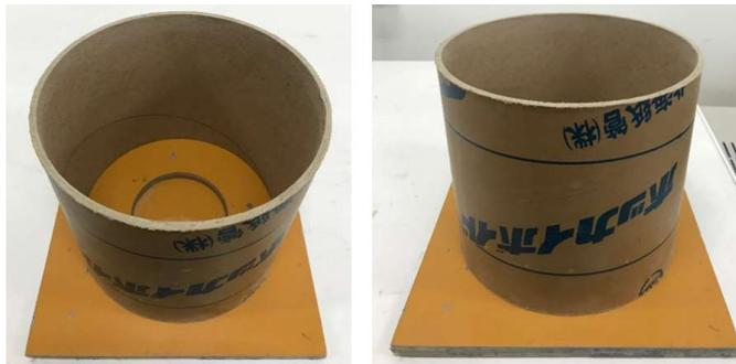
Figure 3.12 - Paper molds used for jacket casting
