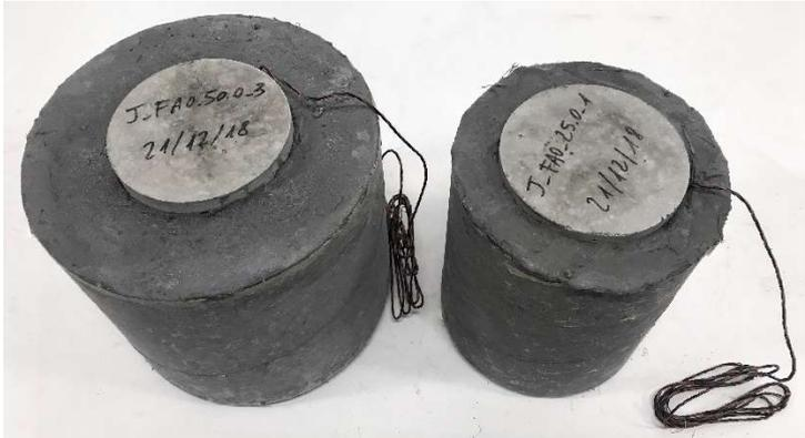
Figure 3.27 - Specimens after the steam curing
