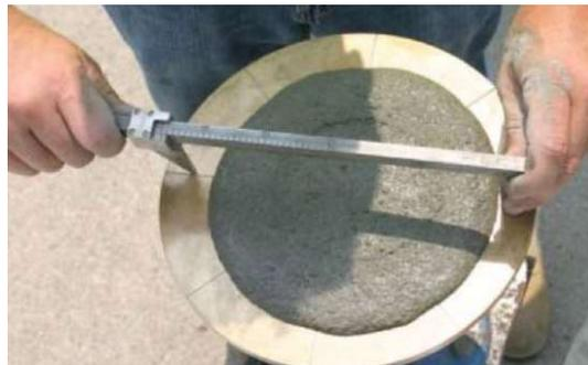
Figure 3.25 - Flow table test of UHP-FRCC
