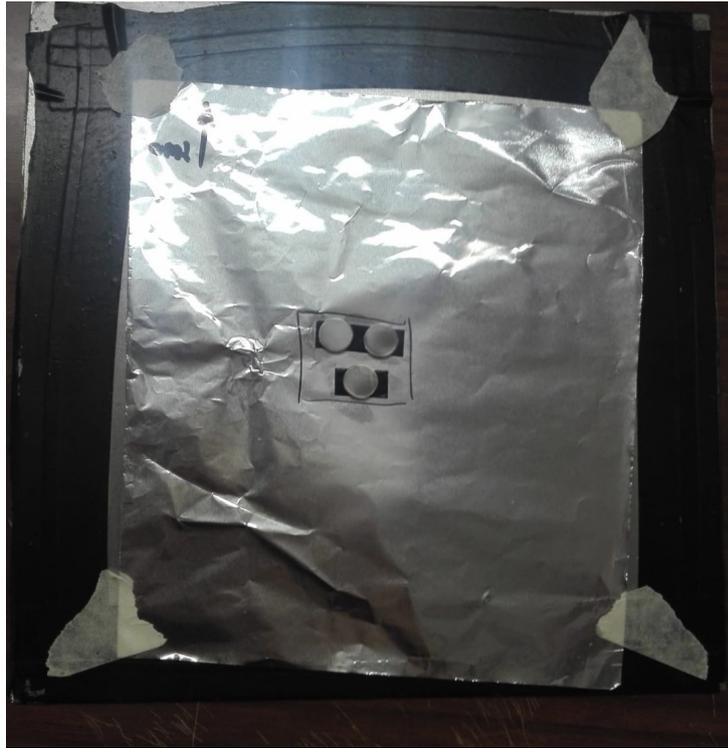
Figure 4.15: Samples placed on metal collector covered with aluminum foil
