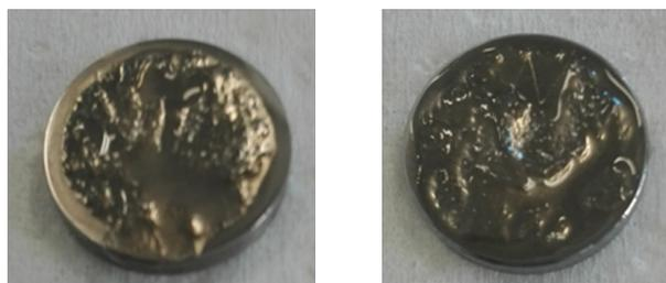
Figure 5.24: Samples 1 and 2 after 14 days of immersion
