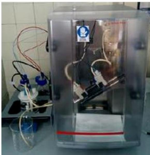
Figure 4.41: Electrokinetic analyzer for zeta potential measurement
