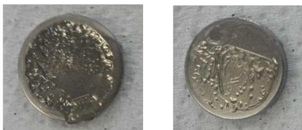
Figure 5.26: Samples 1 and 2 after 28 days of immersion
