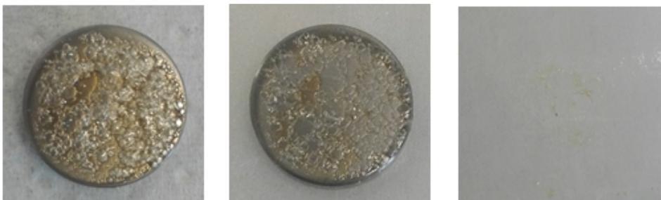
Figure 5.4: Tape test on Ti + UV + ker 7% wt
