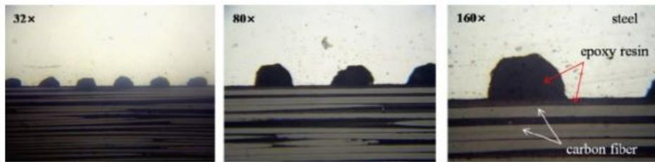
Figure 2.14: Cross section of a steel/composite bonded interface (F34)
