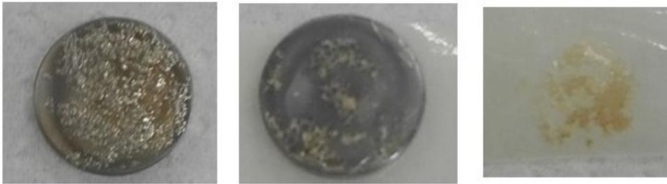
Figure 5.2: Tape test on Polished + ker 7% wt
