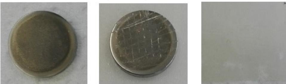
Figure 5.6: Tape test on Ti + plasma + ker 3% wt
