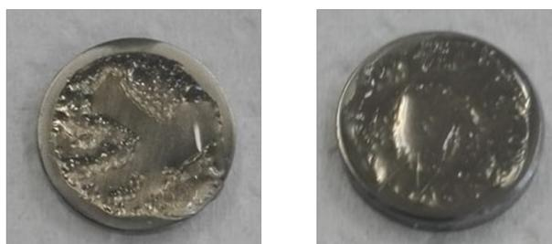
Figure 5.25: Samples 1 and 2 after 21 days of immersion
