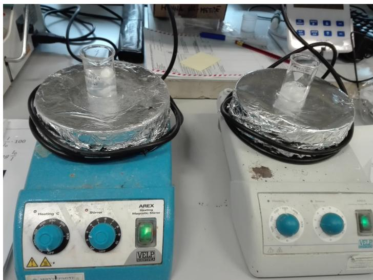
Figure 4.10: Keratin solutions in agitation on vibrating plates
