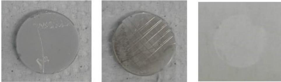
Figure 5.8: Tape test on Ti + plasma + keratin nanofibers
