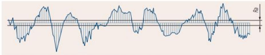
Figure 4.32: Arithmetical mean roughness value  $R_a$  (F92)
