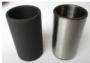
Figure 2.10: Phosphate coating (F30)
