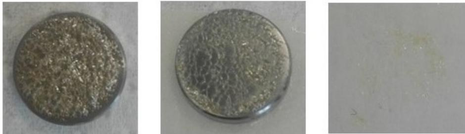
Figure 5.3: Tape test on Ti + plasma + ker 7% wt
