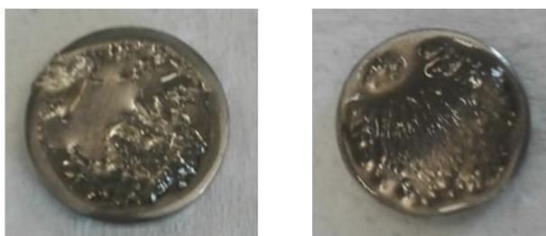
Figure 5.23: Samples 1 and 2 after 7 days of immersion
