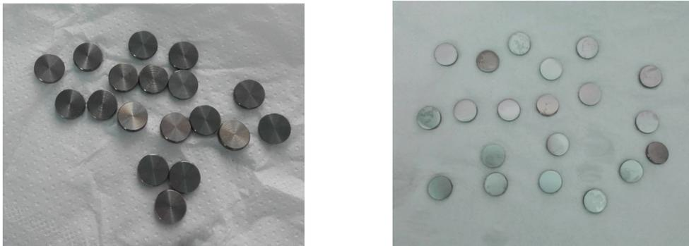
Figure 4.1: Samples before and after polishing
