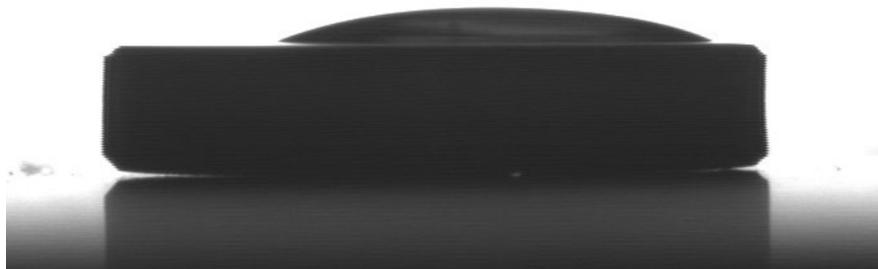
Figure 5.20: Keratin 3% wt drop on plasma-treated Ti
