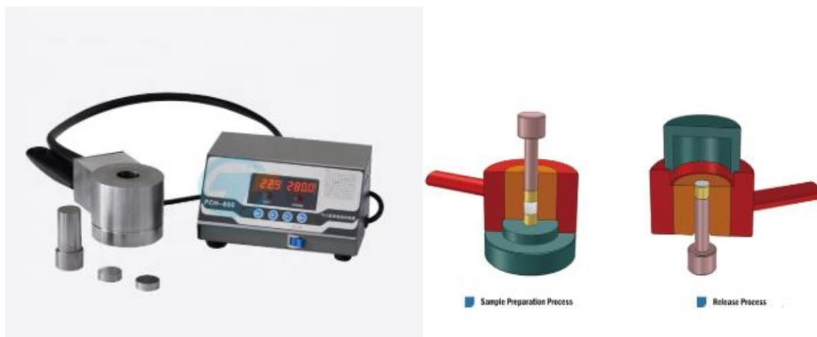
**Figure 5.10** On the left: all components of heatable pellet press die set. On the right: cross section of the piston-and-mold system that shows how the components are arranged together during the compression, the one on the left is showing the sample preparation process and the one on the right the pellet release process. The white cylinder is the compressed sample.
