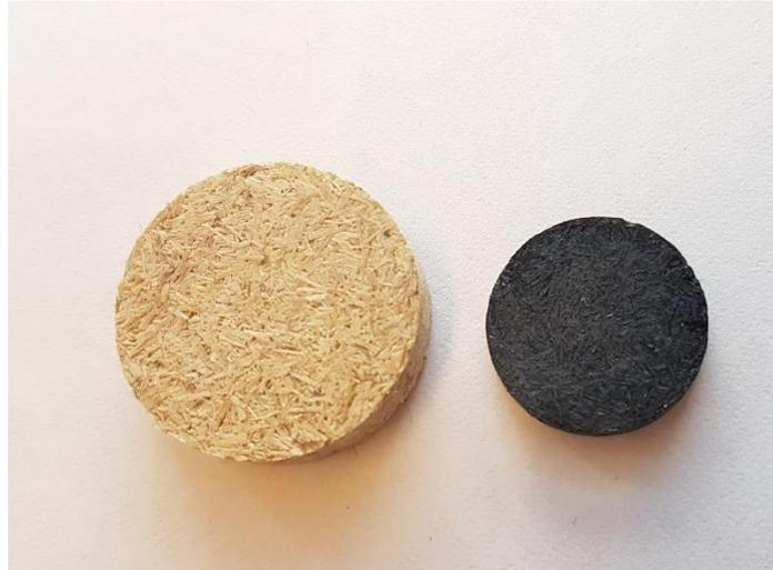
**Figure 5.16** Example of sample before and after pyrolysis. The shrinkage is axial and radial.
