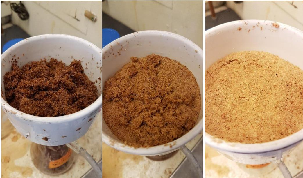
**Figure 5.6** Changing in colour of the sawdust during the immersion in boiling deionized water. On the left: sawdust after the alkali pre-treatment. In the middle: sawdust after some immersion in boiling deionized water. On the right: sawdust at the end of the pre-treatment process.
