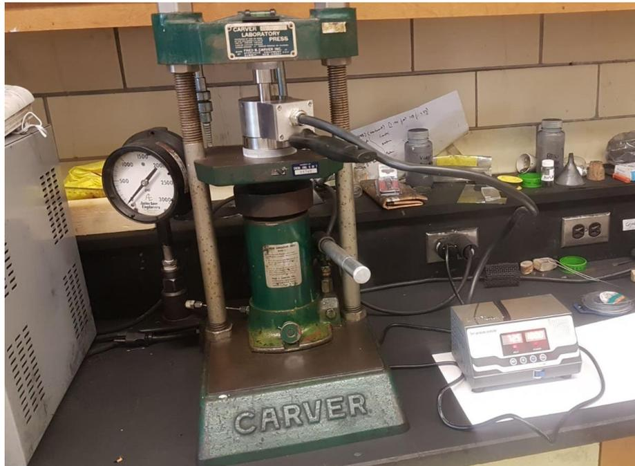
**Figure 5.9** Set-up for sawdust compression to produce pellets.
