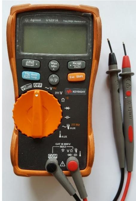
*Figura 2.9 Multimetro Agilent U1231A*
