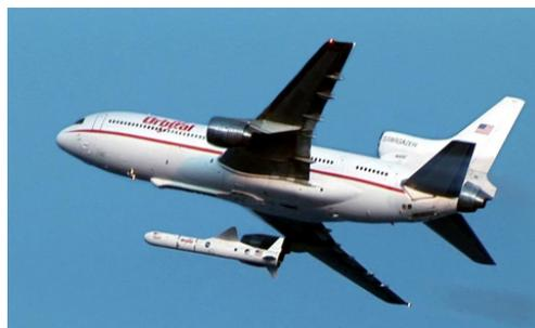
Figure 2.4: PegasusXL: captive on bottom vehicle [credits Northrop Grumman]
