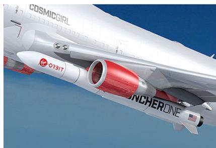
Figure 2.13: LauncherOne on wing bottom of CosmicGirl [credits Virgin Orbit]
