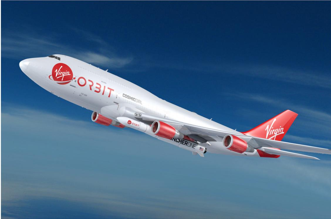
Figure 1.1: An example of air launched flight: Virgin Orbit's LauncherOne [credits Virgin Orbit]
