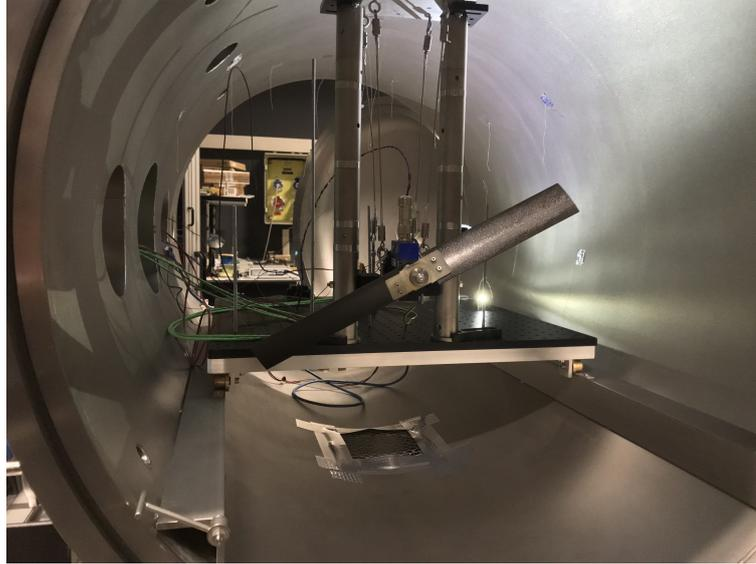
Figure B.3: *Suspended setup within the vacuum chamber.*[21]
