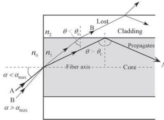
Figure 2.2 - Scheme of a fiber with the distinctive angles of the acceptance and propagation of the light [3]
