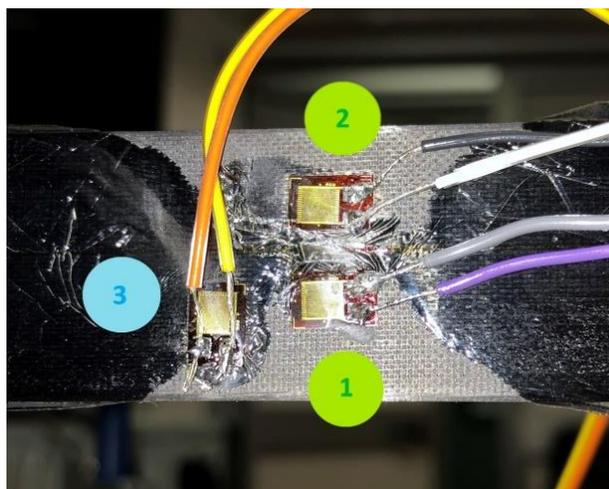
Figure 5.14 - Detail of the sample with the three strain gauges on it. The strain gauges 1 and 2 are for the strain in direction of the principal axis of the sample, and the strain gauge 3 is for the strain in the perpendicular direction
