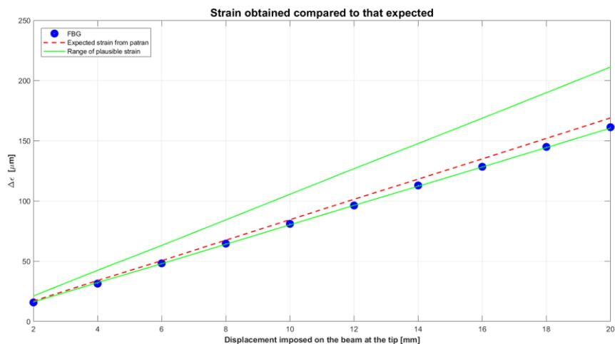
Figure 0.4 - Progress of microstrain, in the Bragg Gratings of the 1F\_1B sample, made on the 22<sup>nd</sup> February 2019. The red line is the expected value of microstrain in output from Nastran - Patran. Instead, the zone between the green lines, is the range of values plausible, it depends on the thickness of the glue used
