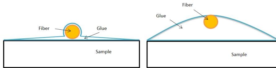
Figure 6.6 - Frontal section of fiber glued, in two cases: the first if you have put a very low layer of glue, and the second if you have put too much glue
