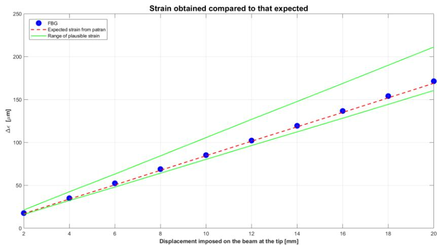
Figure 5.8 - Progress of microstrain, in the Bragg Gratings of the test of 1F\_1B sample, made on the 20<sup>th</sup> February 2019. The red line is the expected value of microstrain in output from Nastran - Patran. Instead, the zone between the green lines, is the range of values plausible, it depends on the thickness of the glue used
