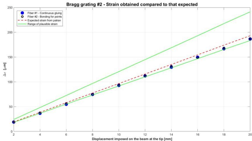
Figure 5.5 - Progress of micro strain, in the Bragg Gratings #2, of the two fibers, by the FBGs of 2F\_2B, made on the 14<sup>th</sup> January 2019. The red line is the expected value of microstrains in output from Nastran - Patran. Instead, the zone between the green lines, is the range of plausible values, it depends on the thickness of the glue used
