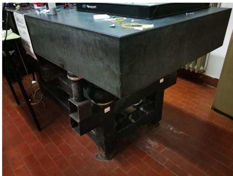
Figure 3.10 - First layer: it is a big and heavy table with dampers
