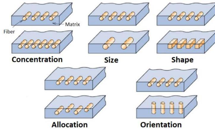
Figure 3.7 - The properties of the composite material are defined by a lot of variables about the coupling of the fibers and the matrix
