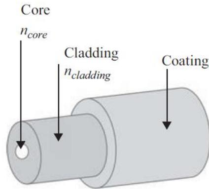
Figure 2.1 - Basic geometry of fiber optic [2]
