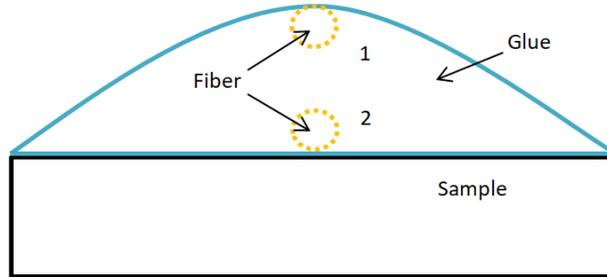
Figure 6.3 - Scheme of frontal section of the group sample and glue, with the possible positions, upper and downer, of the fiber
