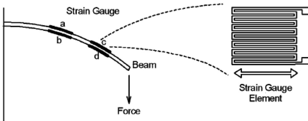
Figure 3.22 - Example of operation of the strain gauge [8]
