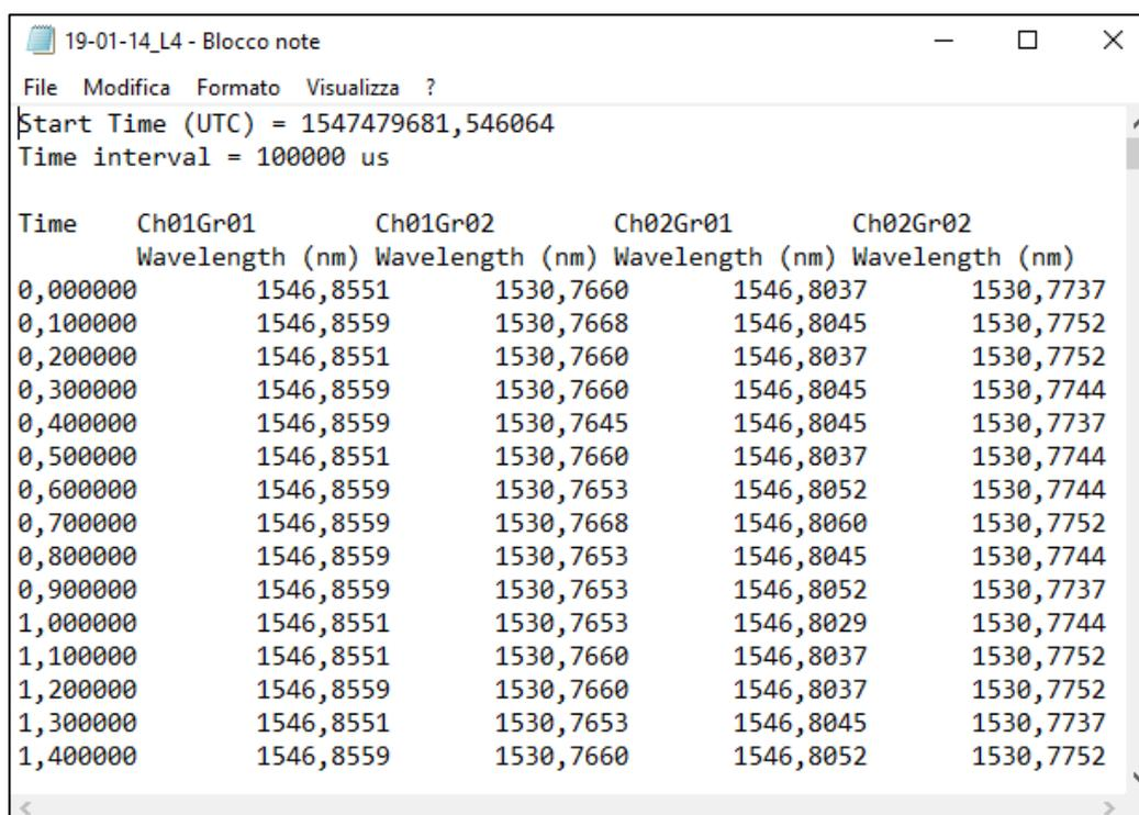
Figure 4.3 - An example of the output file of the SmartSoftSSI. This output presents the analyse of two fibers and each fiber has two Bragg Gratings (Ch = channel, Br = Bragg grating)
