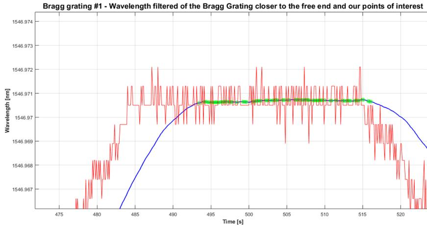
Figure 4.5 - Processing of the values of wavelength and extraction of the mean of the step
