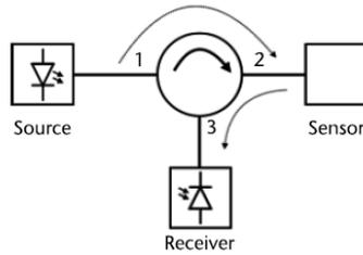
Figure 3.20 - Schematic representation of the use of a circulator to interrogate a sensor working in reflection [7]
