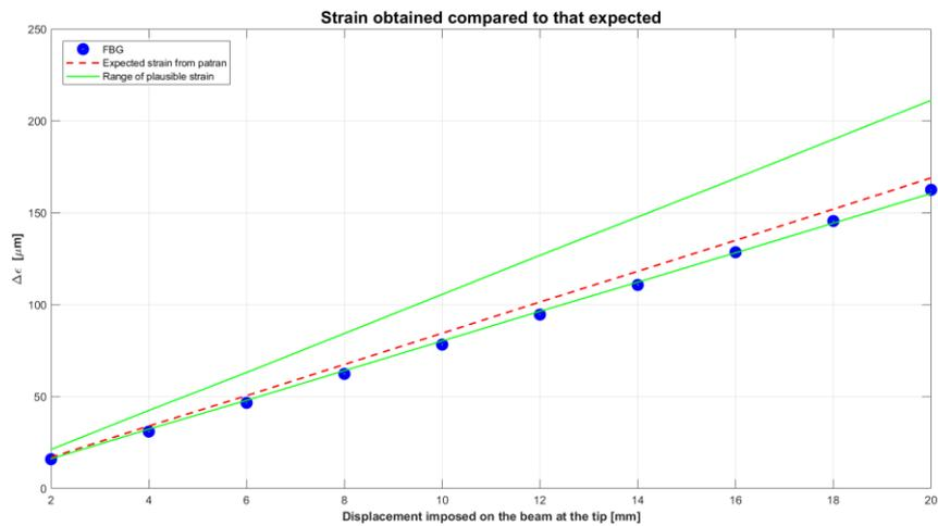
Figure 0.6 - Progress of microstrain, in the Bragg Gratings of the 1F\_1B sample, made on the 4<sup>th</sup> March 2019. The red line is the expected value of microstrain in output from Nastran - Patran. Instead, the zone between the green lines, is the range of values plausible, it depends on the thickness of the glue used
