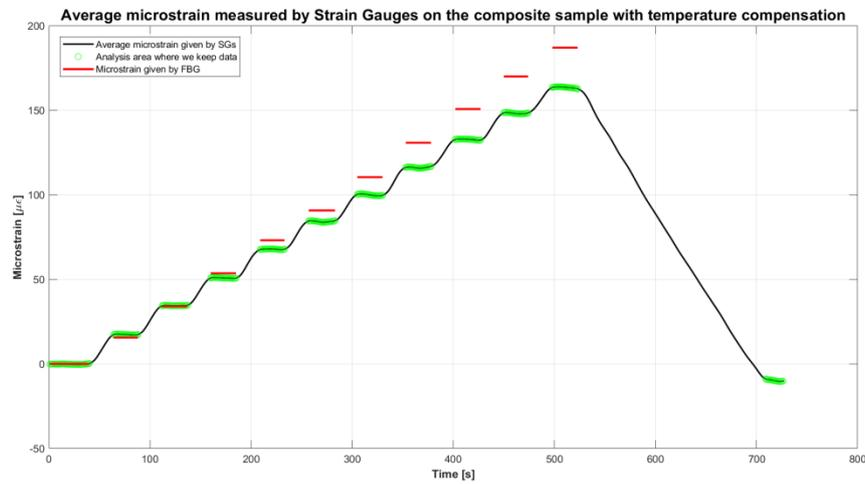
Figure 5.16 - In this picture it is possible to see the measure filtered of the average of the strain gauges, in black, and the point of interest with the green point. The averages of the steps of the FBG output are the red lines
