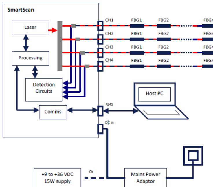
Figure 3.19 - SmartScan system diagram [6]
