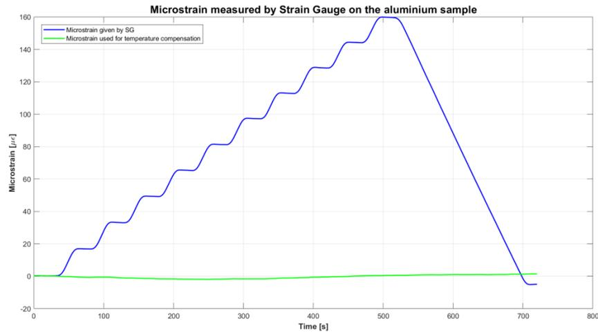
Figure 5.9 - In the graph it is possible to see the strains measured by the strain gauge, the blue line, and the measure of the free strain gauge, with the green line; this will use to do the thermal offset
