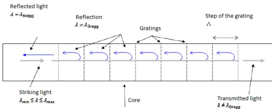
Figure 2.3 - Scheme of Bragg grating with the movements of the light [5]
