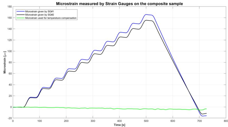
Figure 5.15 - In the graph it is possible to see the strains measured by the strain gauges, the blue line and the black line, and the measure of the free strain gauge; this will use to do the thermal offset
