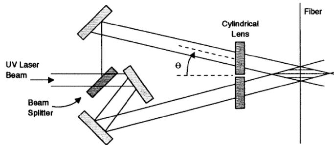
Figure 2.5 - Schematic illustration of the dual-beam holographic technique
