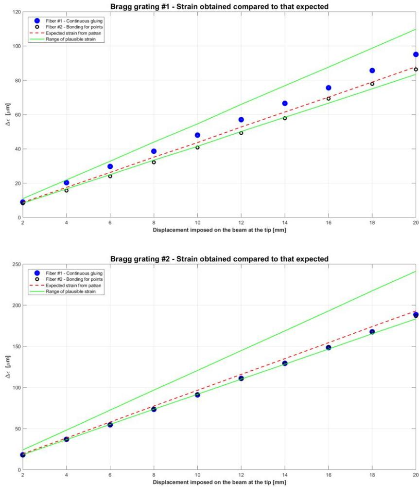
Figure 0.2 - Progress of microstrain, in the Bragg Gratings #1 and in the Bragg Gratings #2, of the two fibers of the 2F\_2B sample, made on the 12<sup>th</sup> February 2019. The red line is the expected value of microstrain in output from Nastran - Patran. Instead, the zone between the green lines, is the range of values plausible, it depends on the thickness of the glue used
