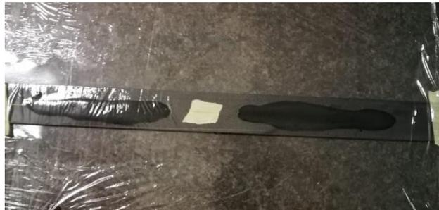
Figure 6.8 - Sample with FBG (in line with the piece of white paper), a layer of glue and the film in PE over all
