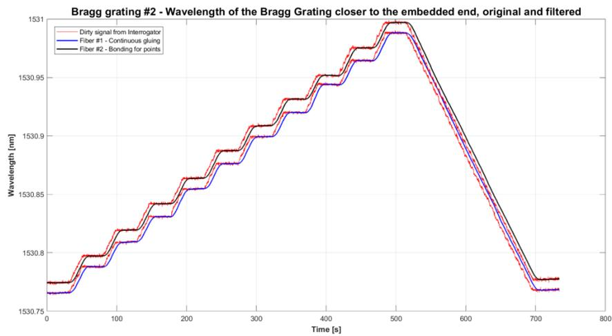
Figure 5.2 - In the two graphs above there are the signals of the FBGs original, from Bragg#1 the first and from Bragg#2 the second. Then there are also their filtered values
