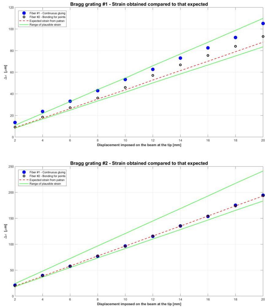
Figure 0.1 - Progress of microstrain, in the Bragg Gratings #1 and in the Bragg Gratings #2, of the two fibers of the 2F\_2B sample, made on the 08<sup>th</sup> February 2019. The red line is the expected value of microstrain in output from Nastran - Patran. Instead, the zone between the green lines, is the range of values plausible, it depends on the thickness of the glue used
