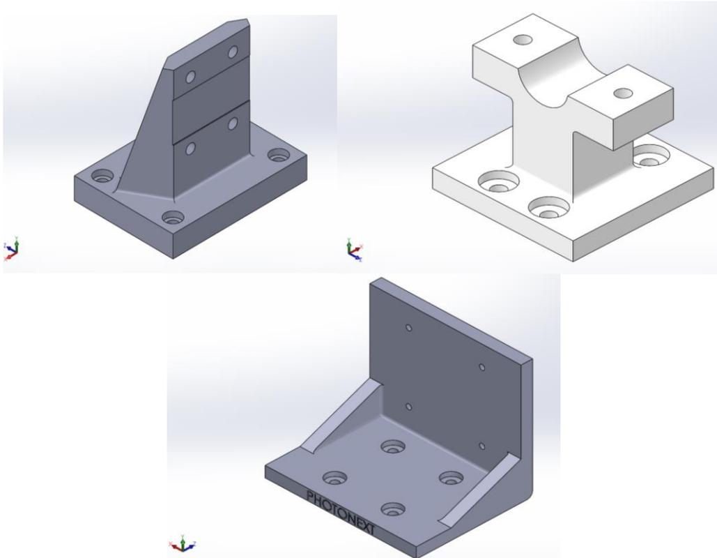
Figure 3.16 - The cad projects of our supports of sample, Faulhaber micromotor and micropositioner in order of time-of-day
