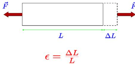
Figure 0.1 - Mechanical strain
