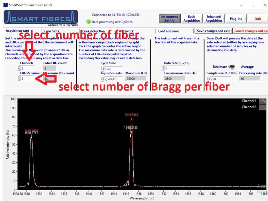
Figure 4.1 - Main screen of SmartSoftSSI. In this example there are two fibers with two Bragg Gratings for each fiber, Fiber #1 is the white curve and Fiber #2 is the red curve
