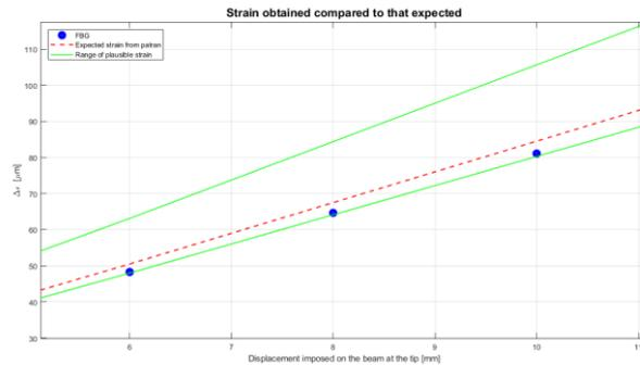
Figure 6.2 - Detail of a graph of the comparison between FBG and Patran-Nastran outputs
