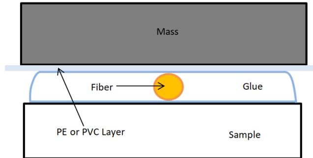
Figure 6.7 - Scheme of the elements and their application to make the new typology of gluing
