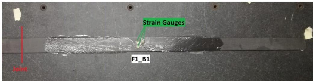
Figure 5.13 - The sample in composite; it is possible to see where the sample is fixed and where the sensors are
