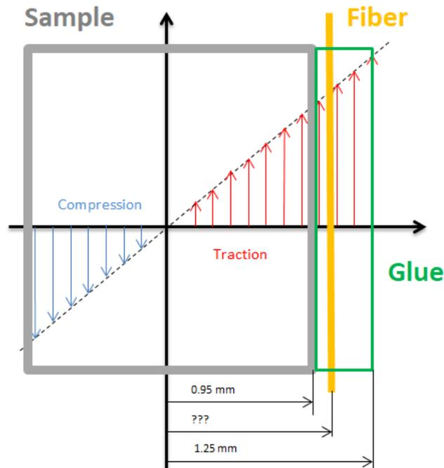
Figure 6.1 - Section of the group sample and fiber glued together
