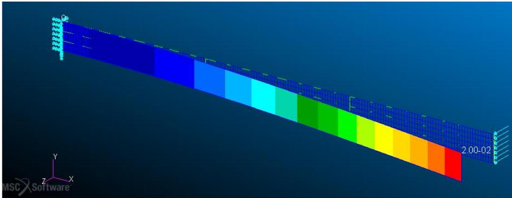
Figure 4.6 - Scheme on Patran of our sample with 20mm of deformation at the tip
