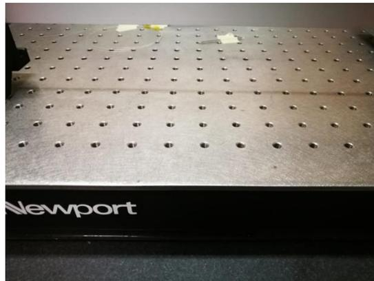
Figure 3.11 - Second layer, the smaller breadboard where samples and tools will be fixed
