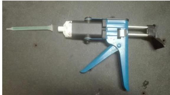
Figure 3.9 - Mixer and applicator of the adhesive
