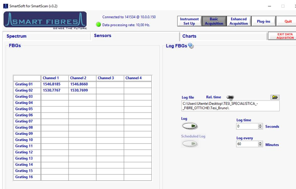
Figure 4.2 - The screen for the basic acquisition. It the same example with two fibers and two Bragg gratings
