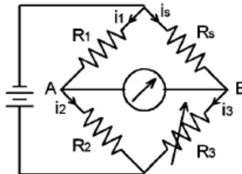
Figure 3.23 - Static balanced bridge circuit, with  $R_s$  that is the resistance of strain gauge
