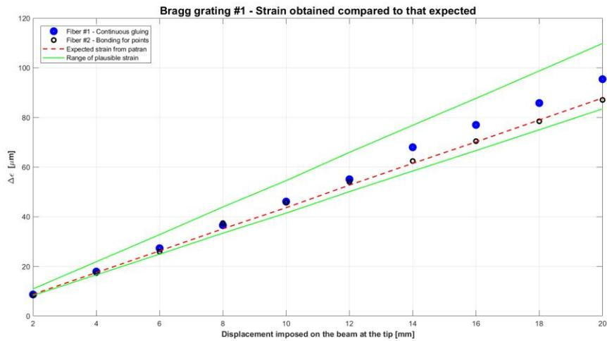
Figure 5.4 - Progress of microstrain, in the Bragg Gratings #1, of the two fibers, by the FBGs of 2F\_2B, made on the 14<sup>th</sup> January 2019. The red line is the expected value of microstrains in output from Nastran - Patran. Instead, the zone between the green lines, is the range of plausible values, it depends on the thickness of the glue used
