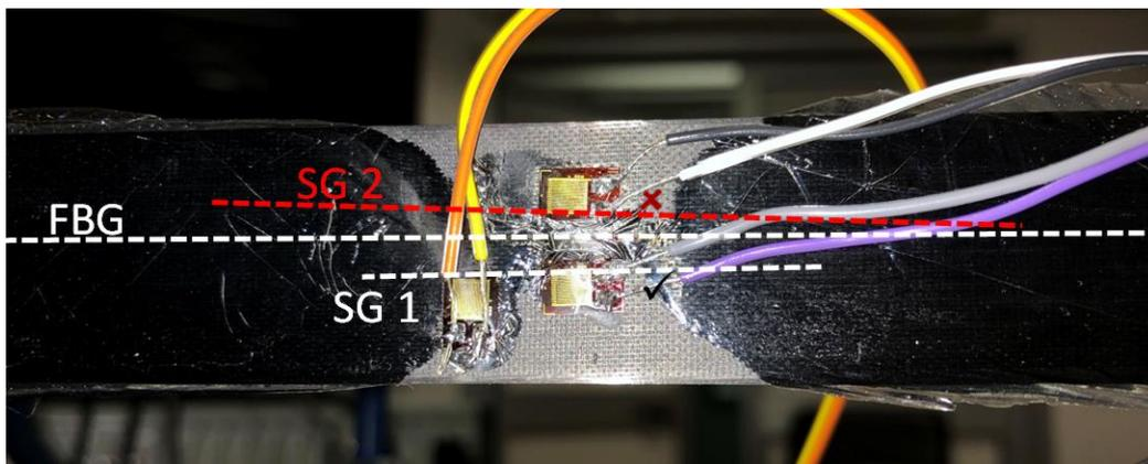
Figure 5.17 - In the picture it is possible to see that the strain gauge 2 is not well aligned with the FBG
