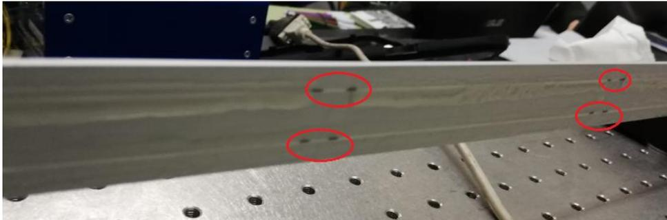
Figure 3.6 - In the picture there is an example of sample with two fibers, and each fiber has two Bragg Gratings
