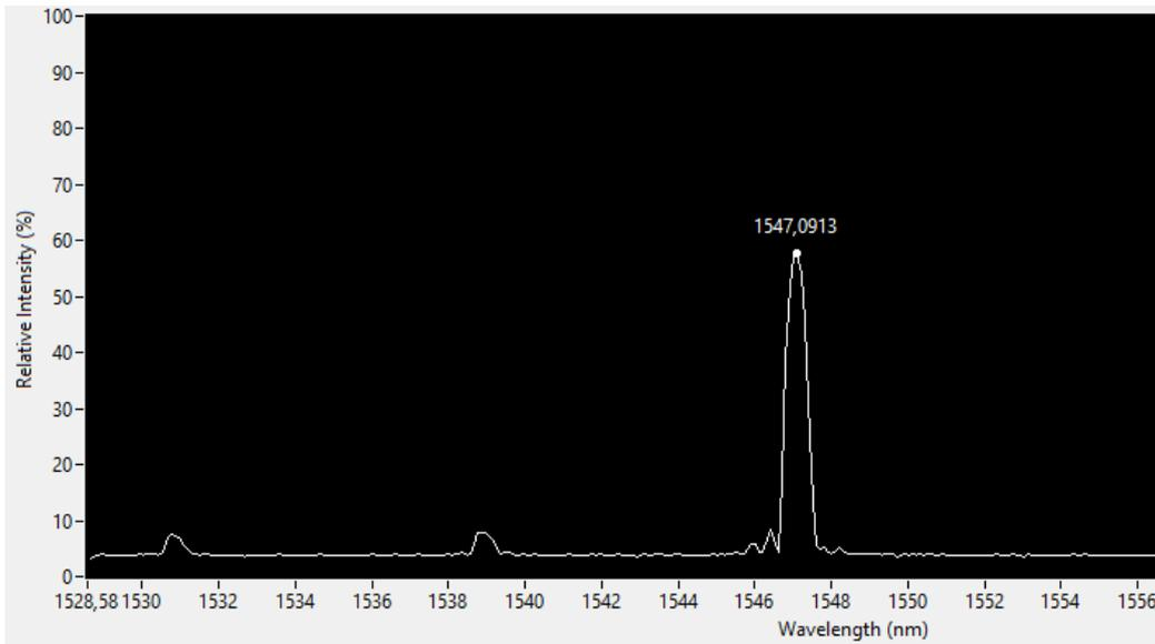
Figure 5.12 - The main screen of the interrogator, it is possible to see the signal of Bragg #1, but the Bragg #2 and #3 are too much low
