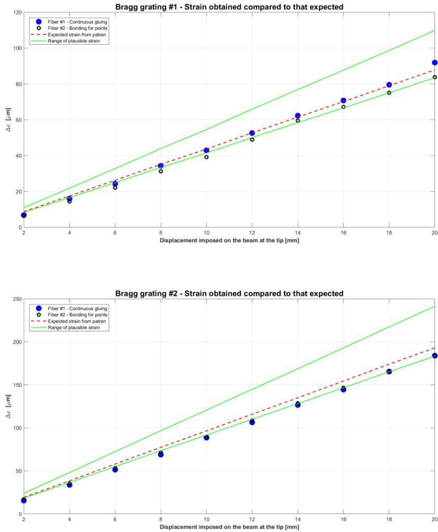
Figure 0.3 - Progress of microstrain, in the Bragg Gratings #1 and in the Bragg Gratings #2, of the two fibers of the 2F\_2B sample, made on the 15<sup>th</sup> February 2019. The red line is the expected value of microstrain in output from Nastran - Patran. Instead, the zone between the green lines, is the range of values plausible, it depends on the thickness of the glue used
