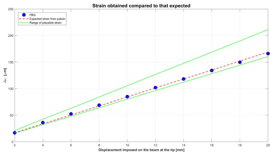
Figure 0.5 - Progress of microstrain, in the Bragg Gratings of the 1F\_1B sample, made on the 27<sup>nd</sup> February 2019. The red line is the expected value of microstrain in output from Nastran - Patran. Instead, the zone between the green lines, is the range of values plausible, it depends on the thickness of the glue used
