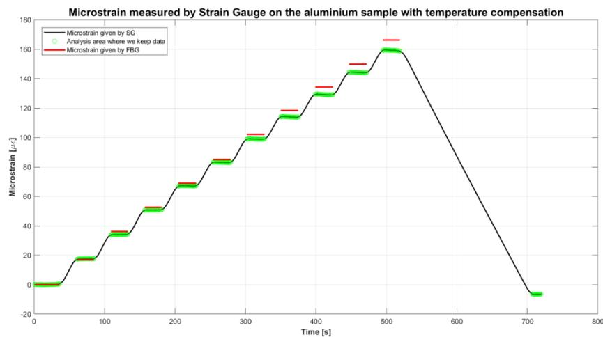
Figure 5.10 - In this picture it is possible to see the measure filtered of the strain gauge in black and the point of interest with the green point. There are also the averages of the steps of the FBG output in the red lines, they are of the test made on the 27<sup>th</sup> February 2019
