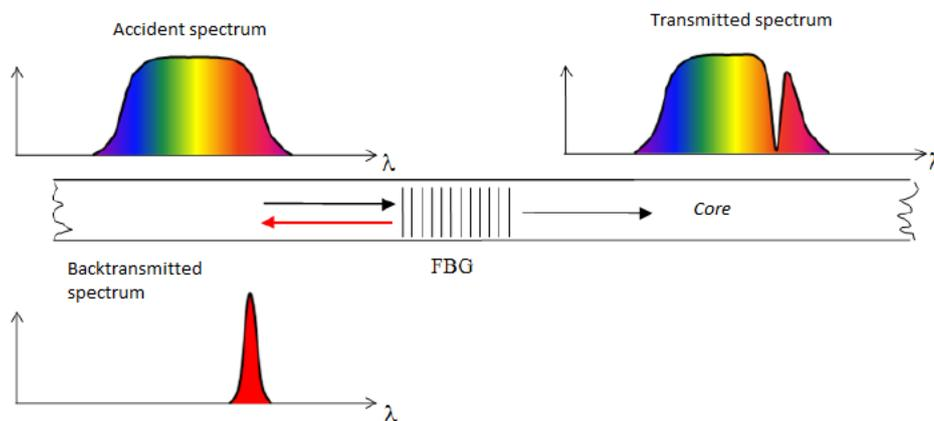
Figure 2.4 - Scheme of the behaviour of the light which strikes the FBG [5]
