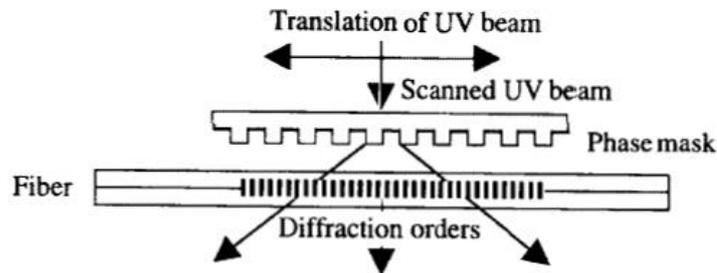
Figure 2.6 - - Schematic illustration of the phase mask technique
