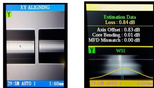
Figure 3.4 - The screen of the monitor of the splicer. In the first figure it is possible to see the profiles of two fibers to be bonded. In the second you can see the signal loss of the junction reported by the displacer
