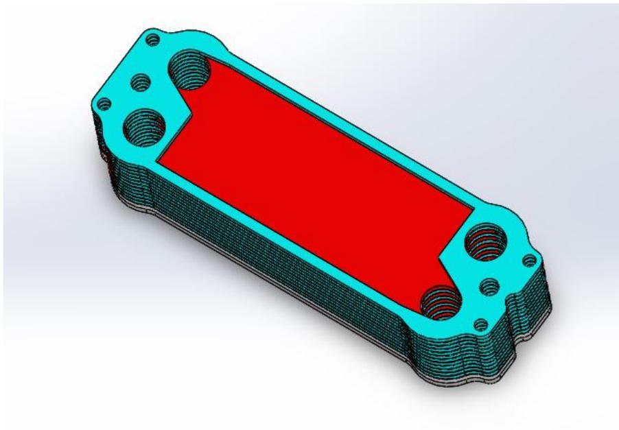
Figure 1.22: View of the inner channel of the heat exchanger, courtesy of *I.C.P.srl*
