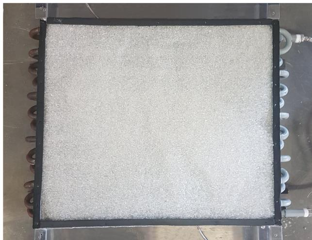
Figure 2.5: HX-ADS Finned heat exchanger filled with silica gel
