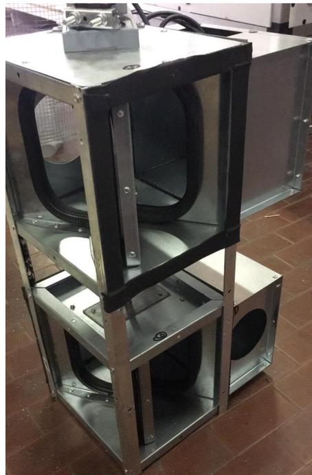
Figure 3.4: Double four-way valve before being installed
