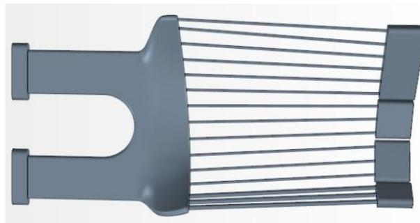
*Figure 6.1: Air domain in new cooling system CFD analysis.*
