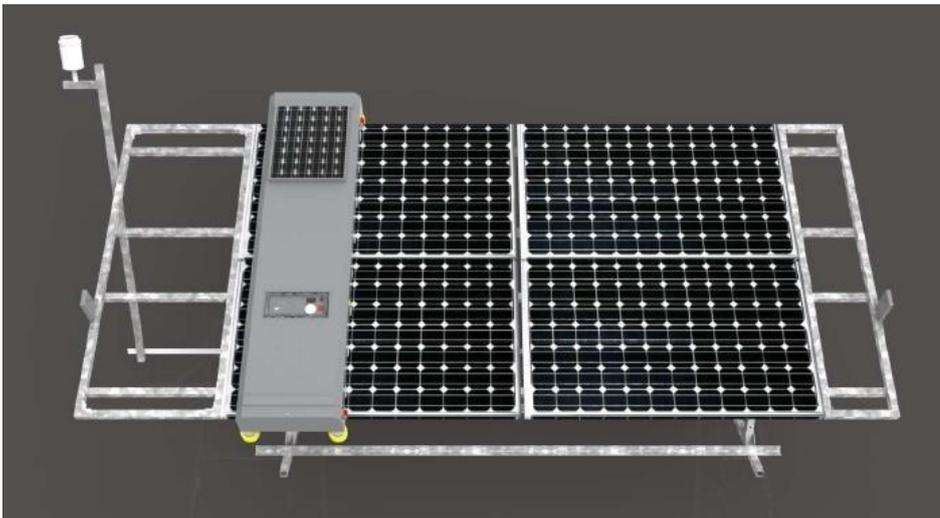
*Figure 3.7 Example of cleaning machine*
