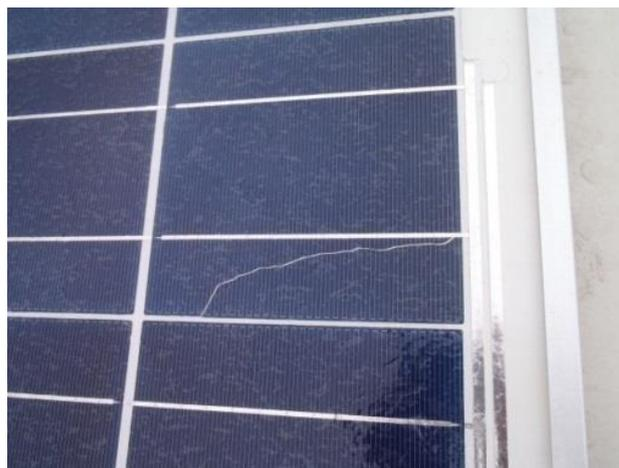
*Figure 4.3 Example of shattering*
