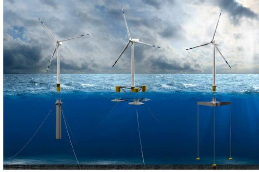
**Figure 1.6:** Archetypes of floating foundations adopted by the wind energy industry. From left to right: spar buoy, semi-submersible platform and tension-leg platform.
