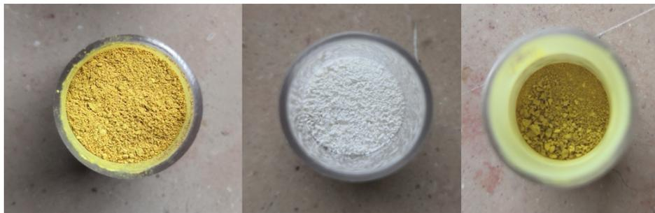
Figure 4.2. MIL-125-NH<sub>2</sub> sample 2 (left), anhydrous SrBr<sub>2</sub> (middle), MIL-125-NH<sub>2</sub>+(45%)SrBr<sub>2</sub> composite (right).
