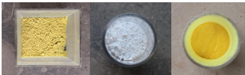
Figure 4.1. MIL-125-NH<sub>2</sub> sample 1 (left), anhydrous CaCl<sub>2</sub> (middle), MIL-125-NH<sub>2</sub>+(45%)CaCl<sub>2</sub> composite (right).
