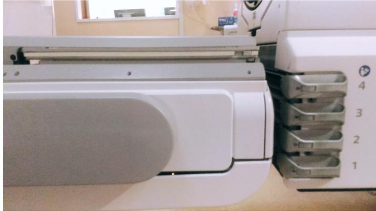
Fig. 2.3: All possible collimators which can be required and mounted on for any acquisition
