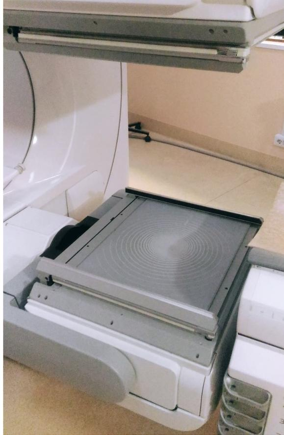
Fig. 2.7: HEAP collimators mounted up with detectors on gamma camera head
