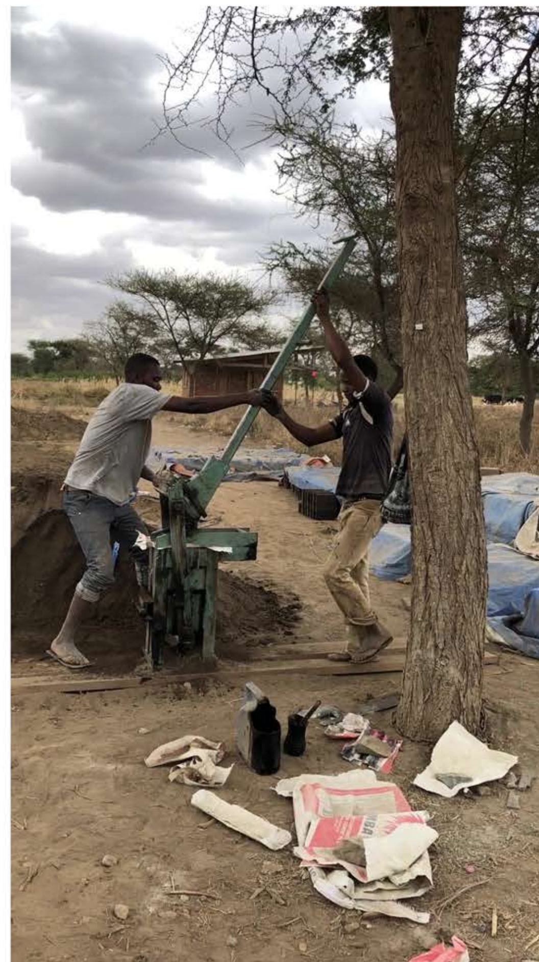
Picture 04. Tanzanian workers compressing earth blocks. Source: Photo by the Author.
