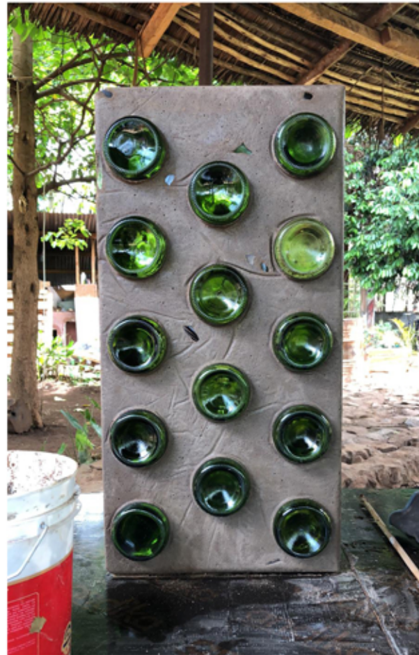
Picture 20. Back view of window prototype, developed with C-re-aid NGO, made from recycled wine bottles casted in concrete. Source: Photo by the Author.
