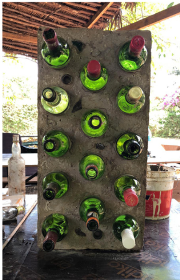
Picture 19. Front view of window prototype, developed with C-re-aid NGO, made from recycled wine bottles casted in concrete. Source: Photo by the Author.
