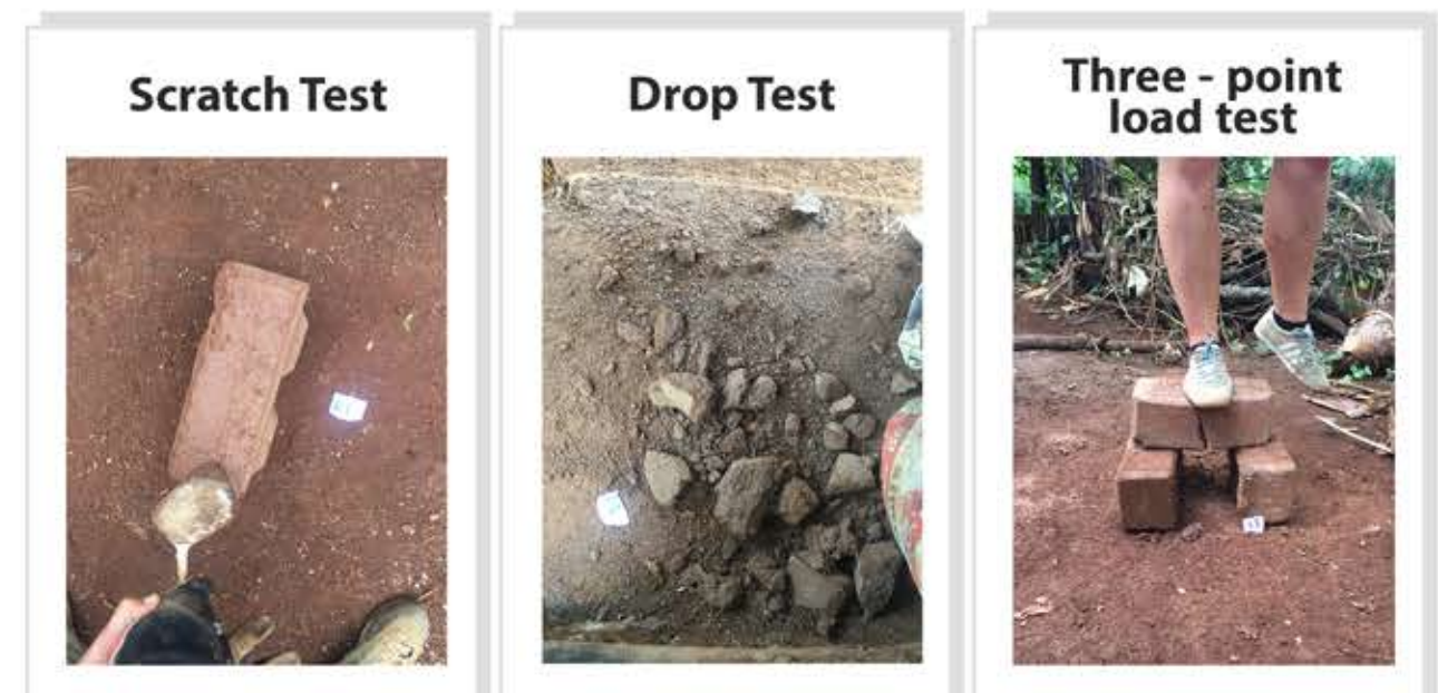
Picture 08. Strength tests in order to determine if the blocks are strong enough. Source: Photos by the Author.
