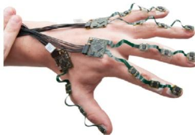
Figura 1.13: Glove, exible-PCB, [49]
