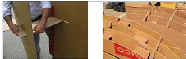
Figura 6.8: Assemblamento centine. Foto M. R..
