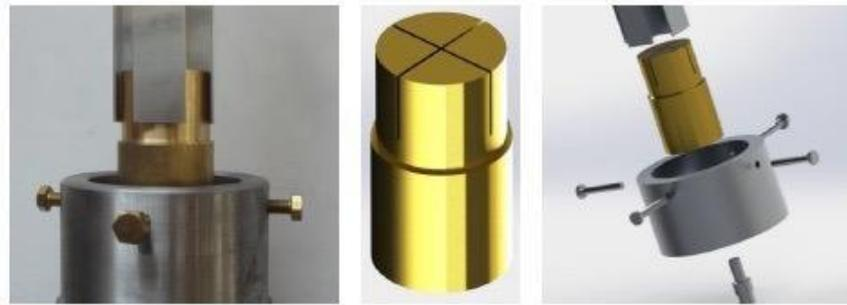
Figure 3.12 - Picture and rendering of lower end constraints
