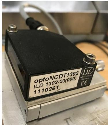
Figure 3.1 – Photo of laser opto NCDT 1302-20
