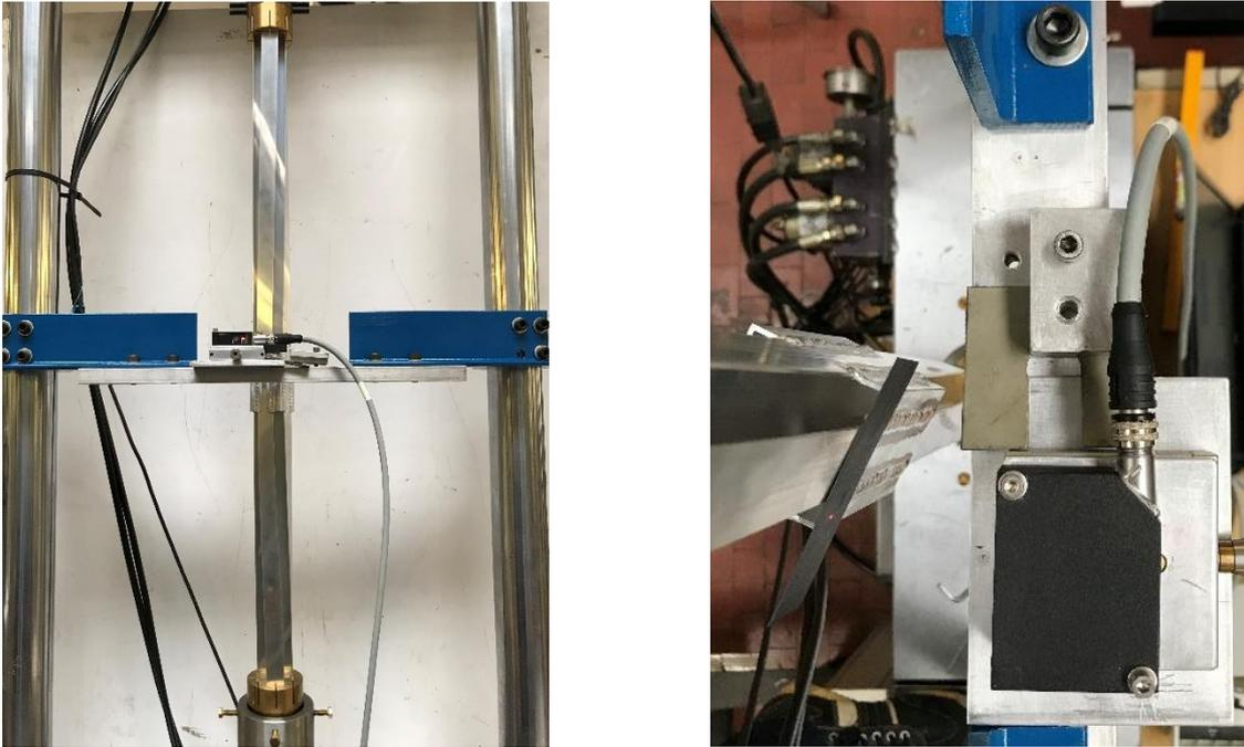
Figure 3.22 – Left: S8 specimen at the end of the test; Right: Top view of torsional instability.
