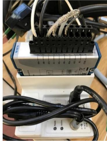
Figure 3.3 - Acquisition device NI 9215
