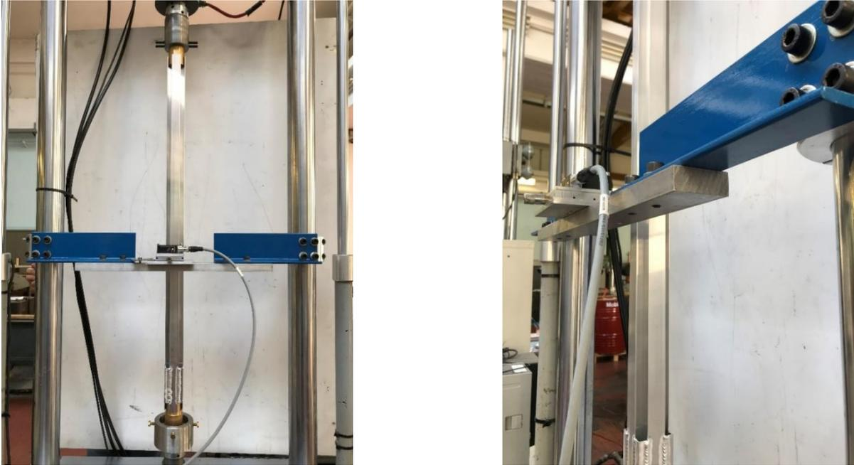
Figure 3.19 – Left: S5 specimen at the end of the test; Right: Zoom of torsion instability.
