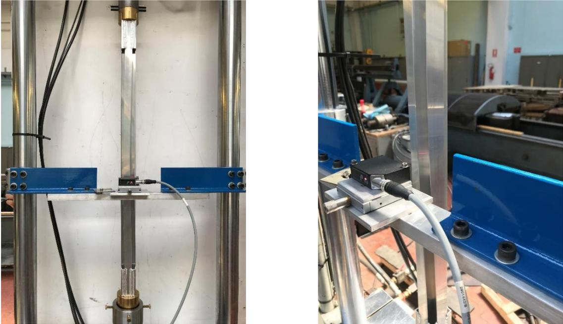
Figure 3.28 – Left : S12 specimen at the end of the test; Right: Zoom of torsion instability.
