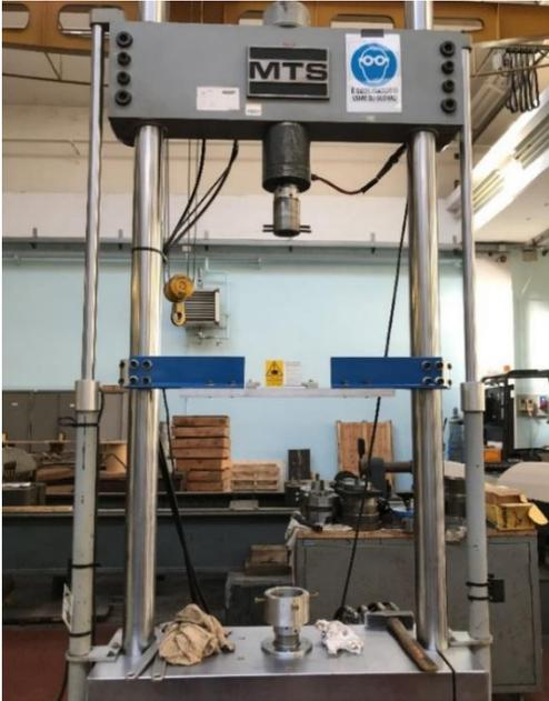
Figure 3.6 - Servo-hydraulic MTS testing machine
