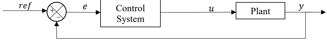
Figure 2.10 - Closed-loop control system
