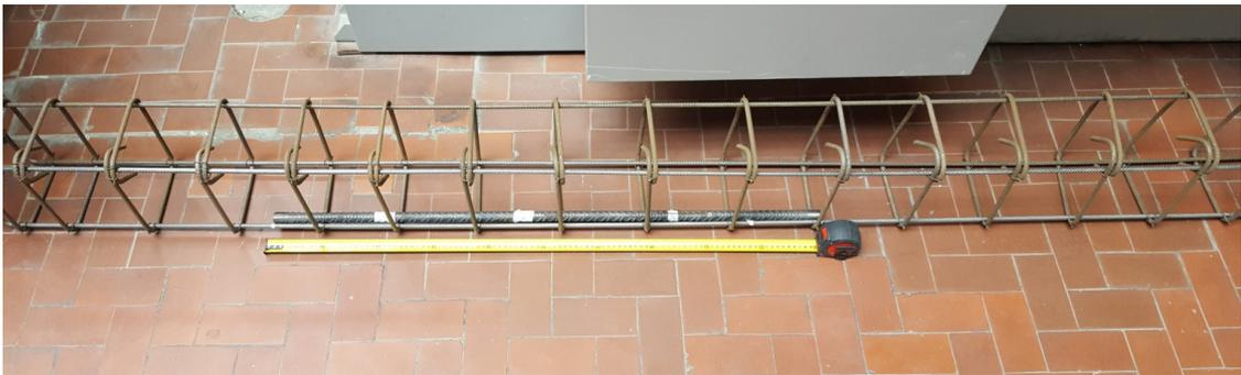
Fig. 86: Reinforcement cage
