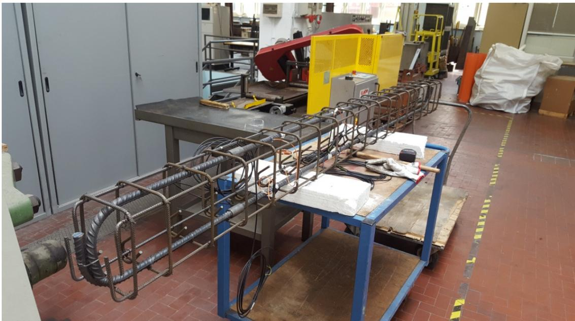
Fig. 89: Reinforcement cage assembled with instrumented reinforcement
