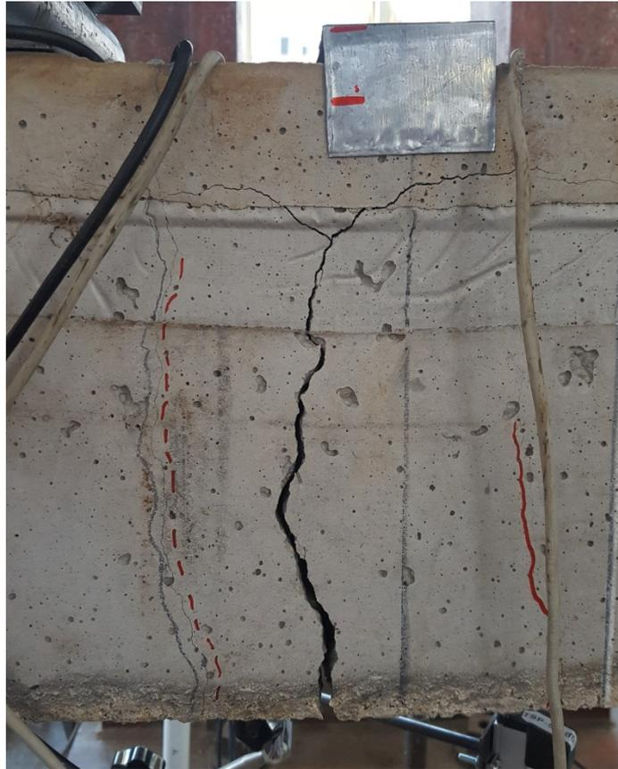
Fig. 106: Fracture detail - Test 18 - Collapse (Max. Load: 88.45 kN)
