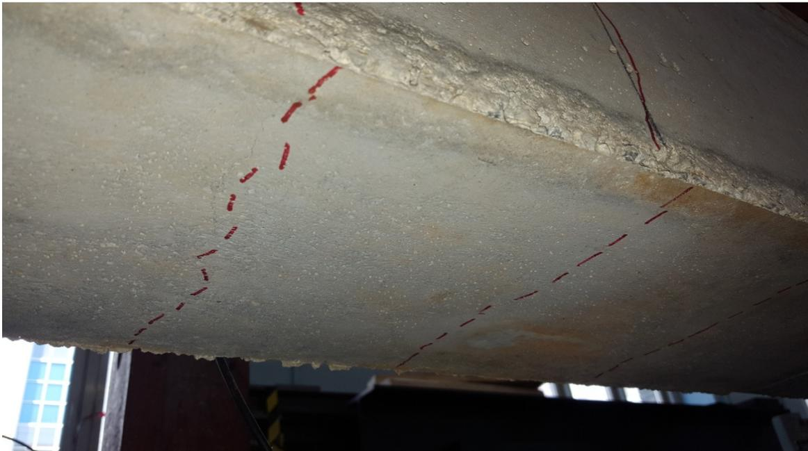
Fig. 115: Crack pattern picture - Test 9 (Max. Load: 25 kN)
