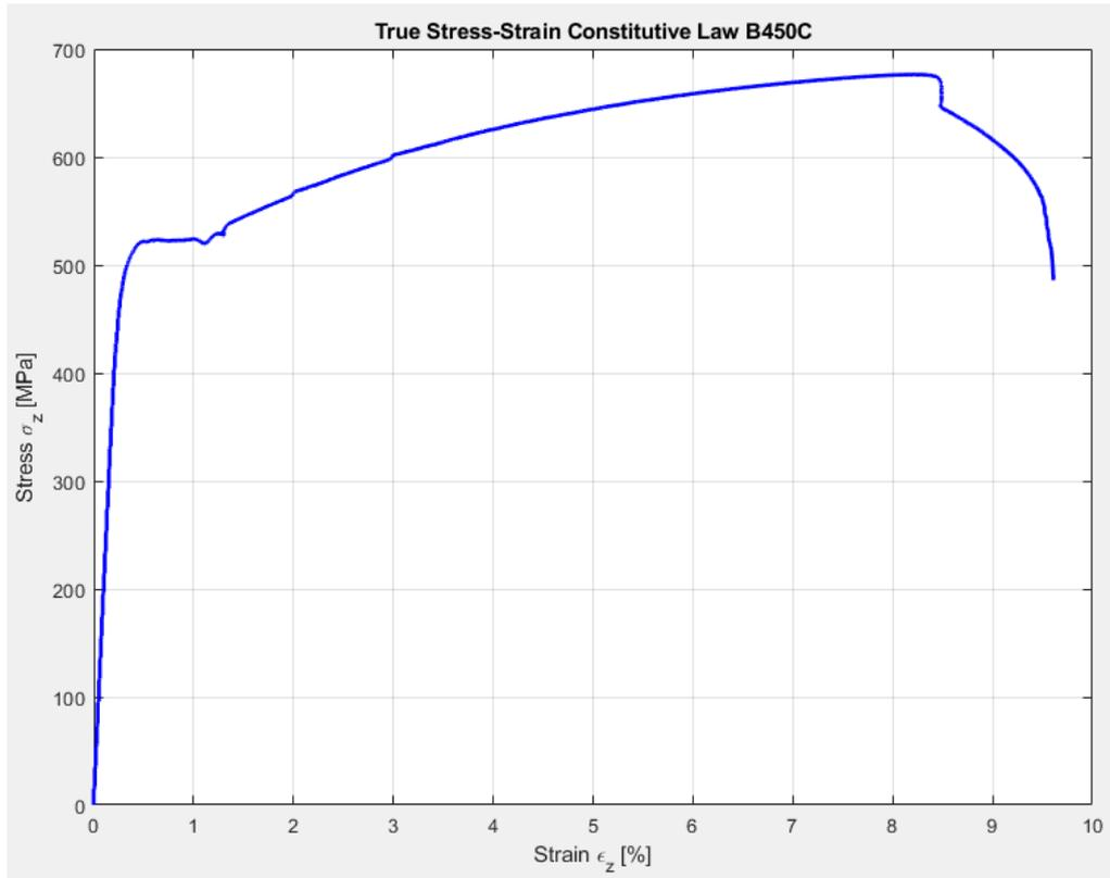
Fig. 26: True stress-strain B450C
