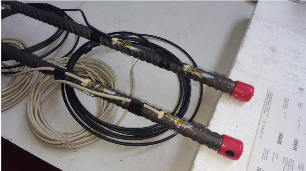
Fig. 83: Strain gauges final configuration
