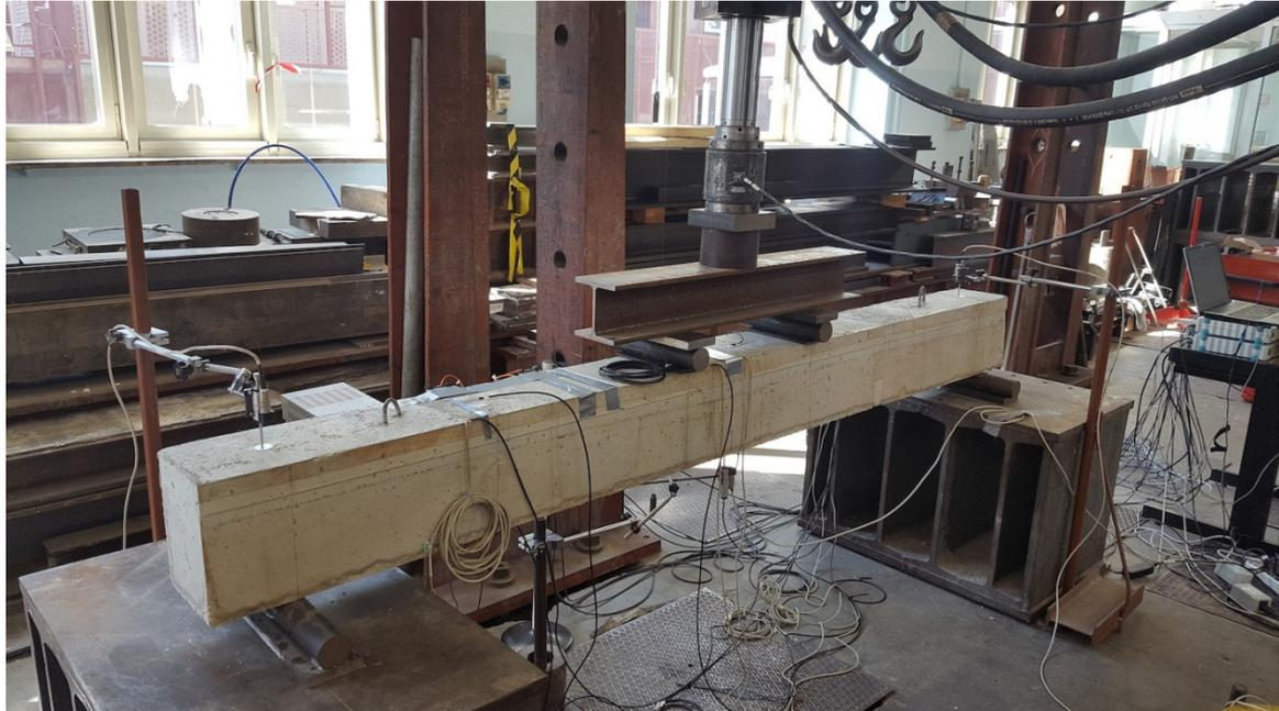
**Fig. 103: Bending test final configuration**
