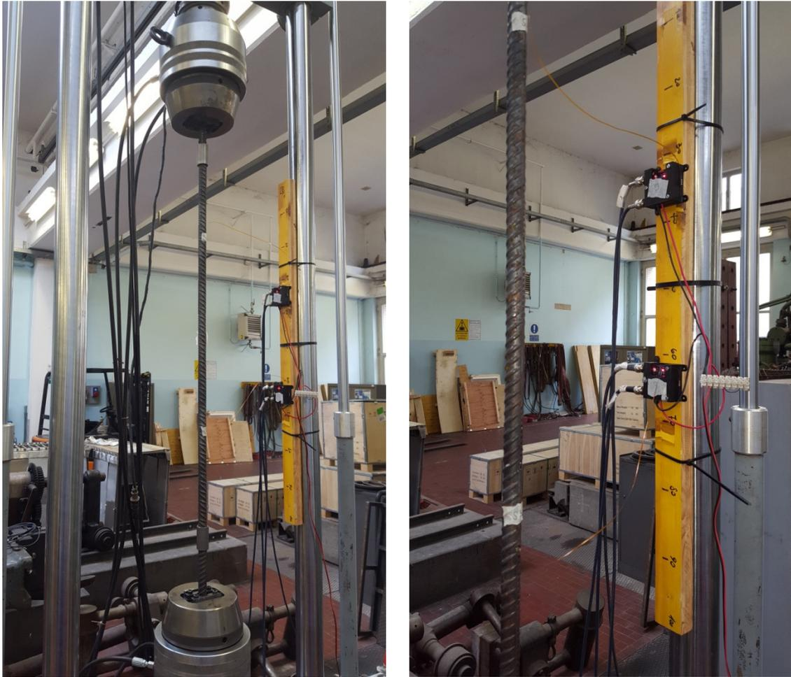
Fig. 74: Axial tensile test configuration (a) and a zoomed view (b)
