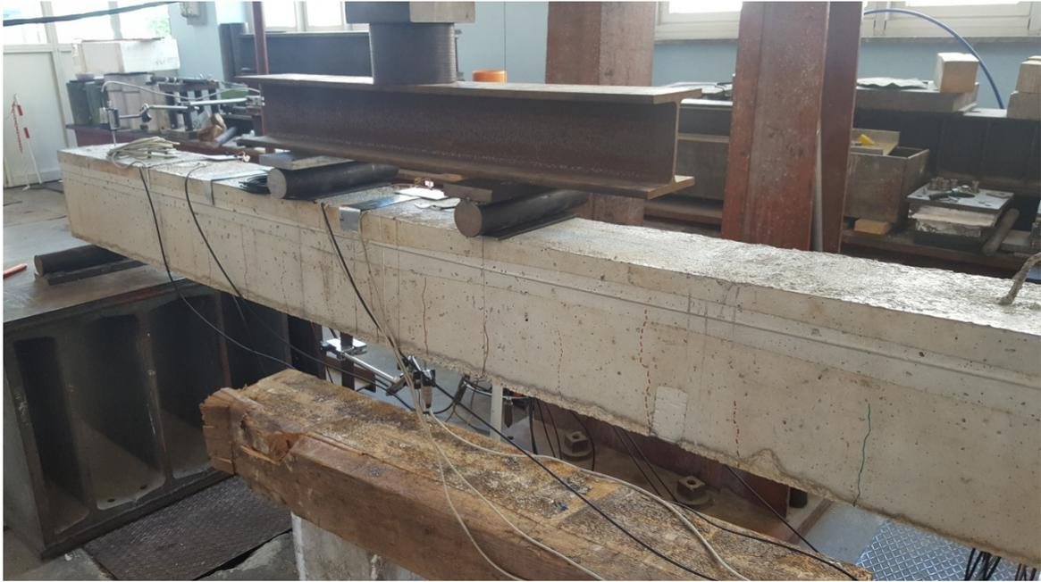
Fig. 116: Crack pattern picture - Test 15 (Max. Load: 55 kN)
