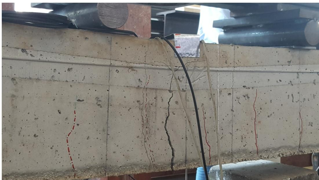
Fig. 105: Fracture - Test 18 - Collapse (Max. Load: 88.45 kN)
