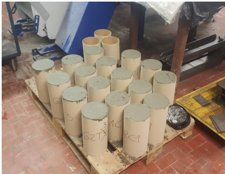
Fig. 96: Cylindrical concrete specimens
