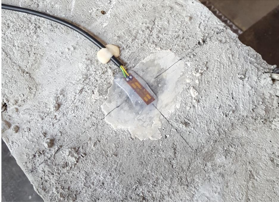
Fig. 99: Strain gauge installation (G01C)
