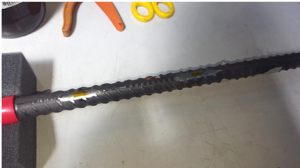
Fig. 82: Strain gauges glued to bar's surface
