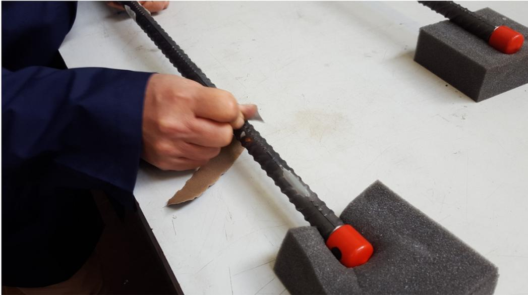
Fig. 81: Sanding off bar's surface
