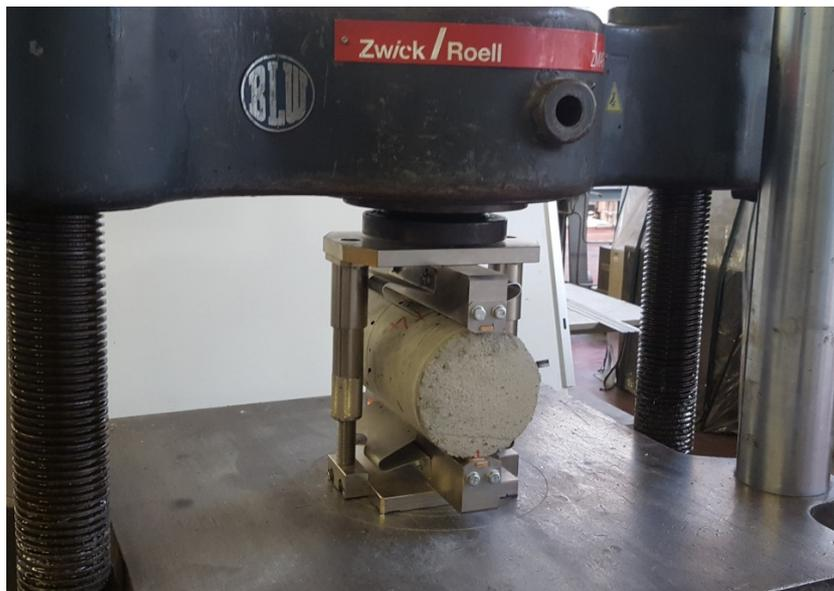
Fig. 98: Indirect tensile strength test
