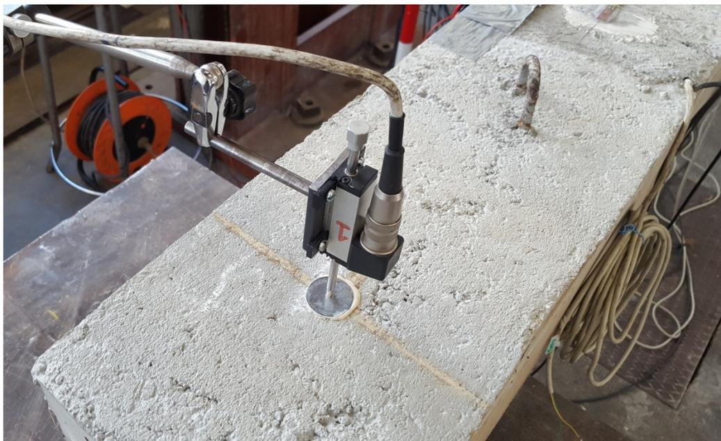
Fig. 101: LVDT installation (LVDT-left)
