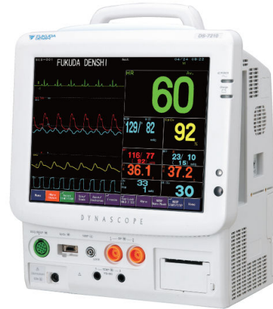
Figure 2.2.2: Dynascope Monitor DS-7100 (Fukuda Denshi Co.). Here the DS-7200 version is displayed as an example.
