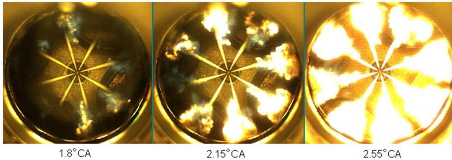
FIGURE 2.4. Combustion in an optically accessible Diesel engine. The fuel jet spray and the development of a diffusion flame can be seen. Reproduced from Cronhjort (2017).
