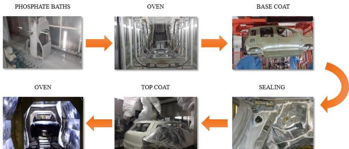
Figure 13 - Summarized scheme of the painting process
