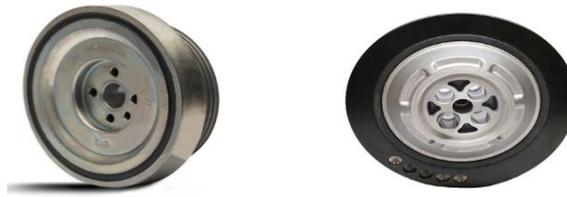
*Figure 2.11 Crankshaft decouplers*
