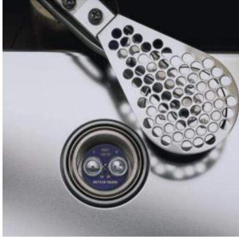
Figure 14 - Furnace detail of DSC.
