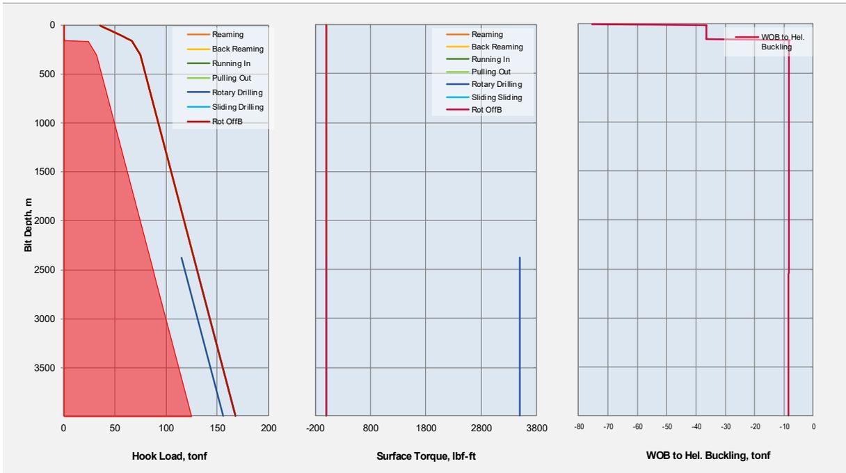
Hook load and surface torque distribution (12 ¼" section)
