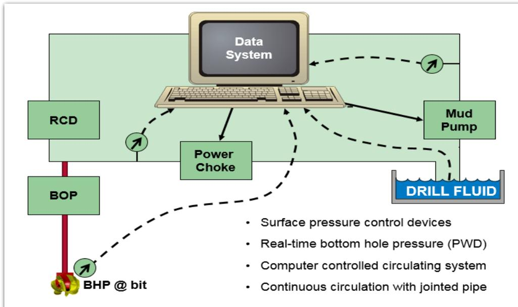
Figure 10- Data acquisition system
