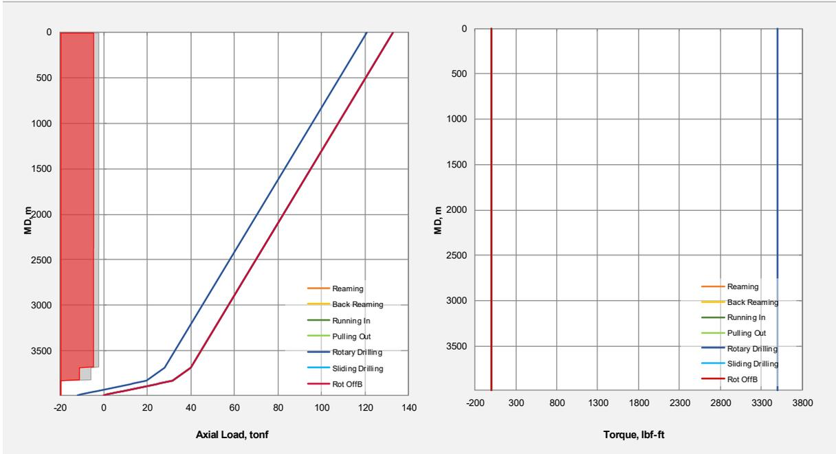
**Axial load and torque while drilling process (12 1/4" section)**
