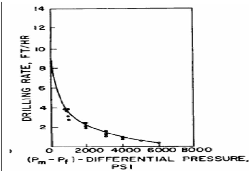
Figure 2 differential pressure impact on rate of penetration
