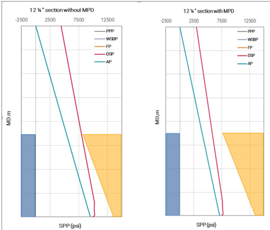
**Figure 21 - Standpipe pressure distribution through wellbore 12 1/4" section**
