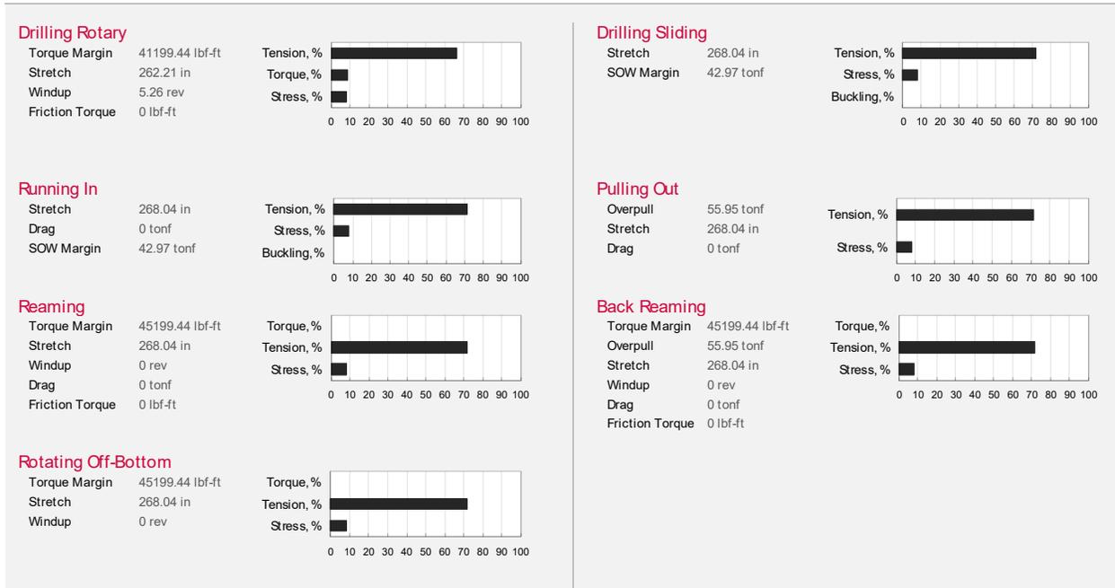
Tension, stress and buckling while tripping in and out (8 1/2" section)
