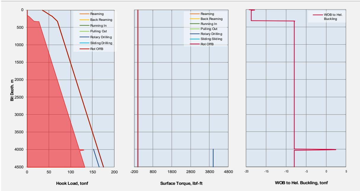
Hook load and surface torque distribution (8 1/2" section)
