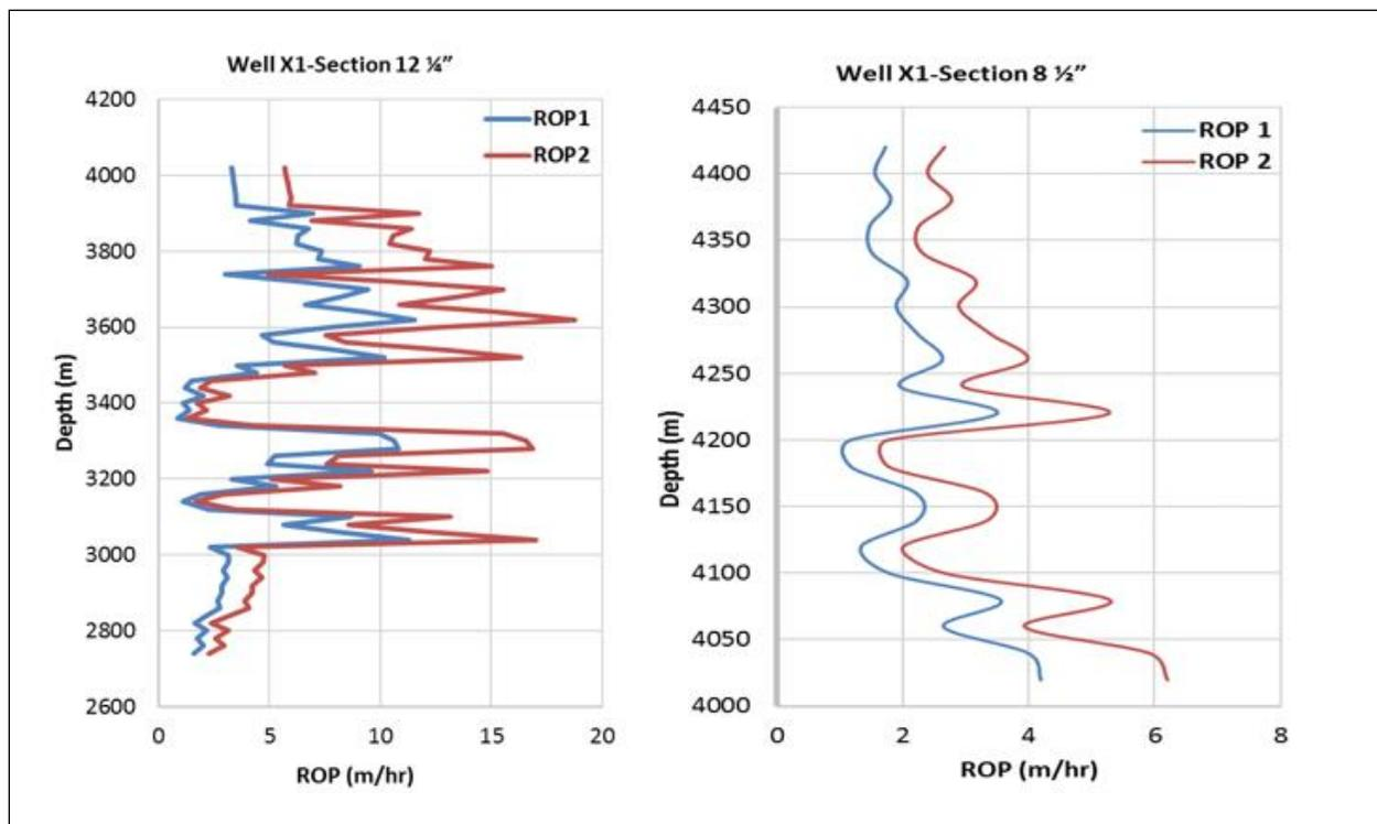
Figure 15- Increment of ROP in 12 ¼" and 8 ½" WELL X1
