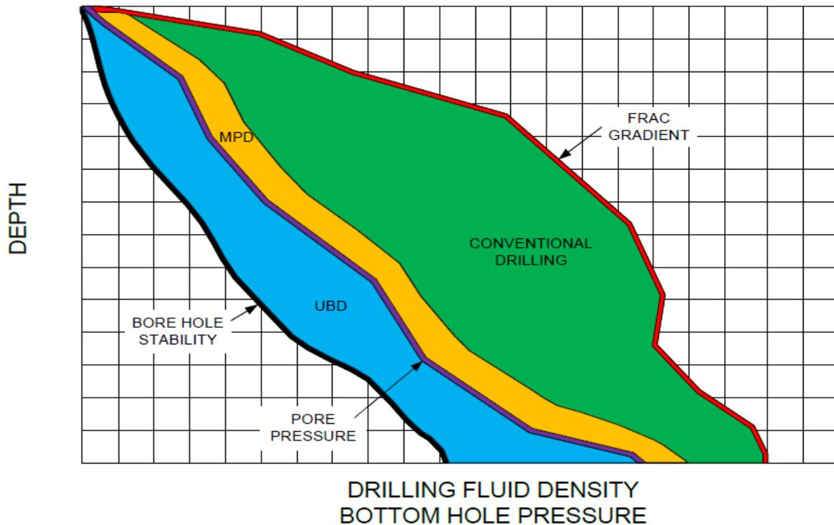
Figure 1- Drilling Window of different systems including MPD, UBD and Conventional Drilling.
