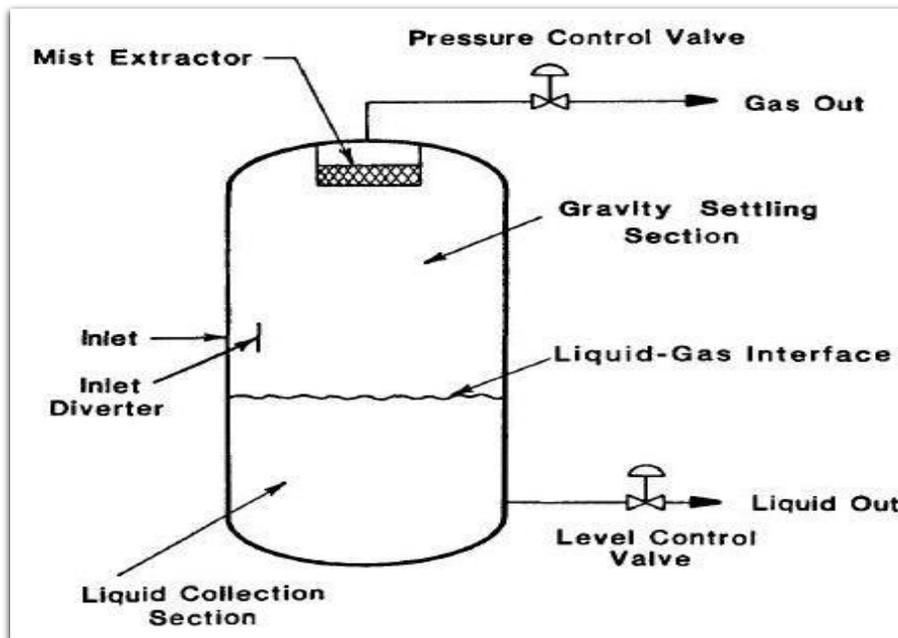
Figure 9- Two phase separator
