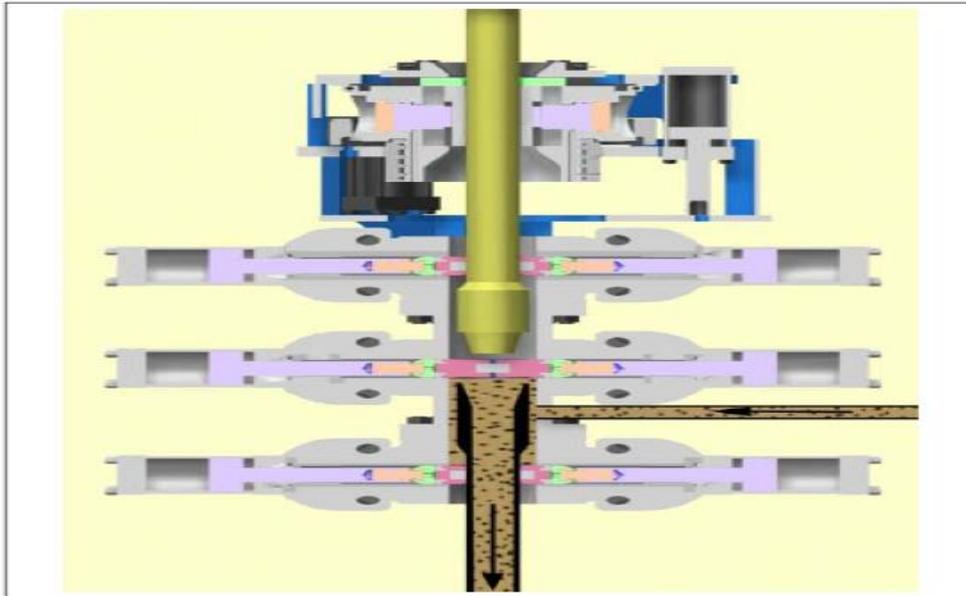
**Figure 5 - Continuous Circulation System method**
