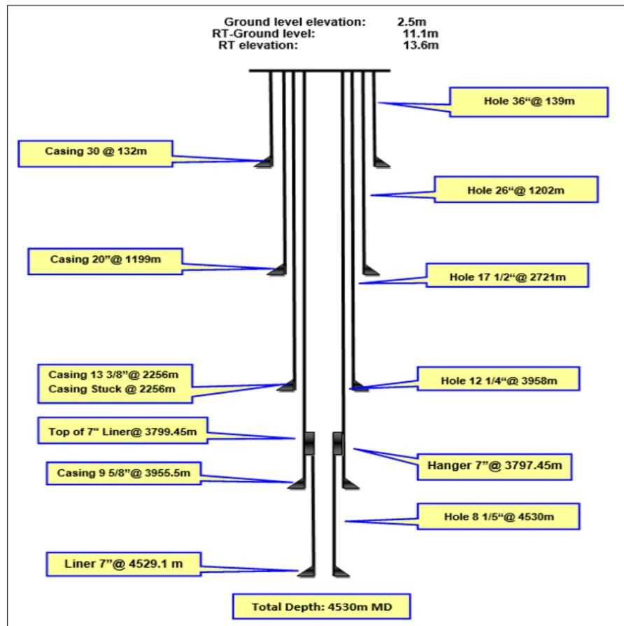
Figure 14 - Well Schematic
