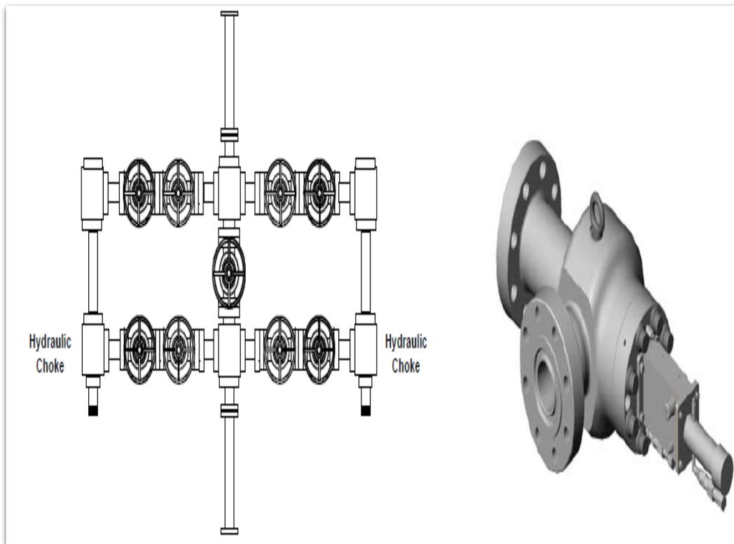
**Figure 8 - Choke manifold**
