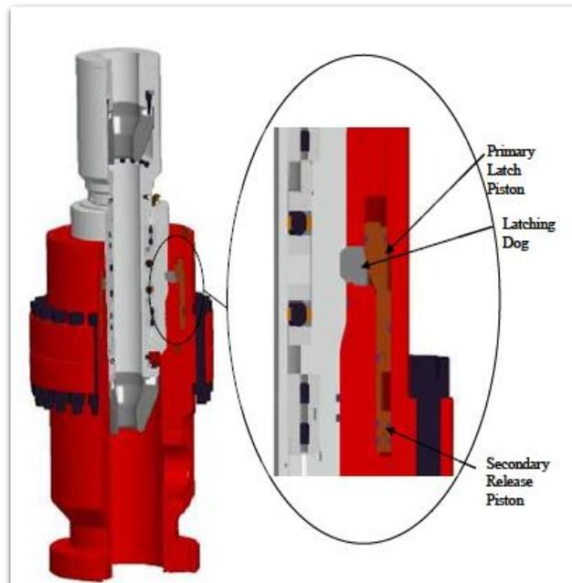
**Figure 7- Rotating Control Device**
