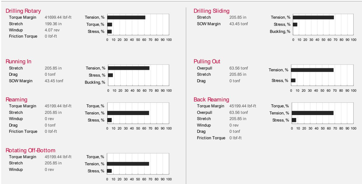
Tension, stress and buckling while tripping in and out (12 1/4" section)
