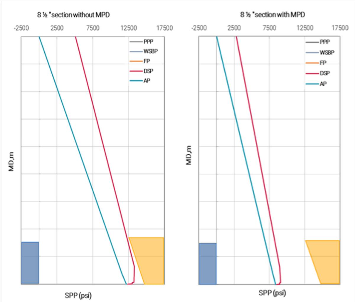
**Figure 23 - Standpipe pressure distribution through wellbore 8 1/2" section**
