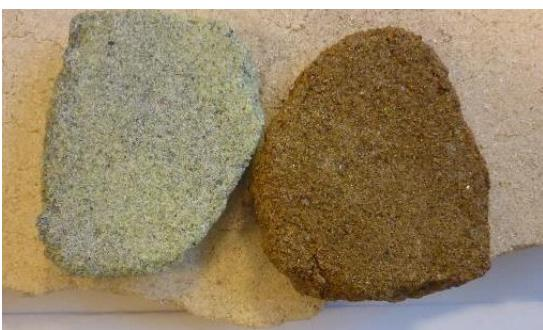
**FIGURE 8 SWEDISH DIABASE BEFORE AND AFTER THE THERMAL CYCLE**
