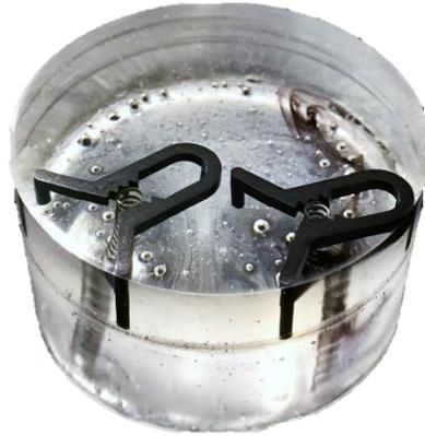
*Figure 3.5 – Embedded chip in epoxy resin to measure the thickness*
