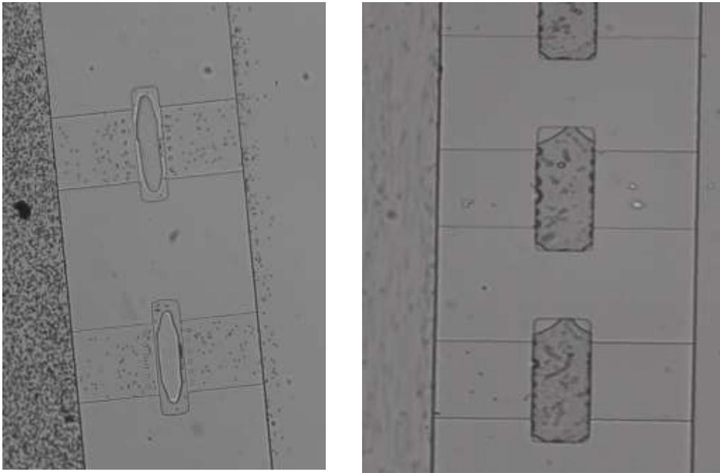
*Figure 22. optical micrograph of filter membranes. Flow rate of 0.2  $\mu\text{l}/\text{min}$  and 2 $\mu\text{m}$  polystyrene microbeads simulating E-coli cells. Left: PEG-DA, right: HEMA-EDMA*
