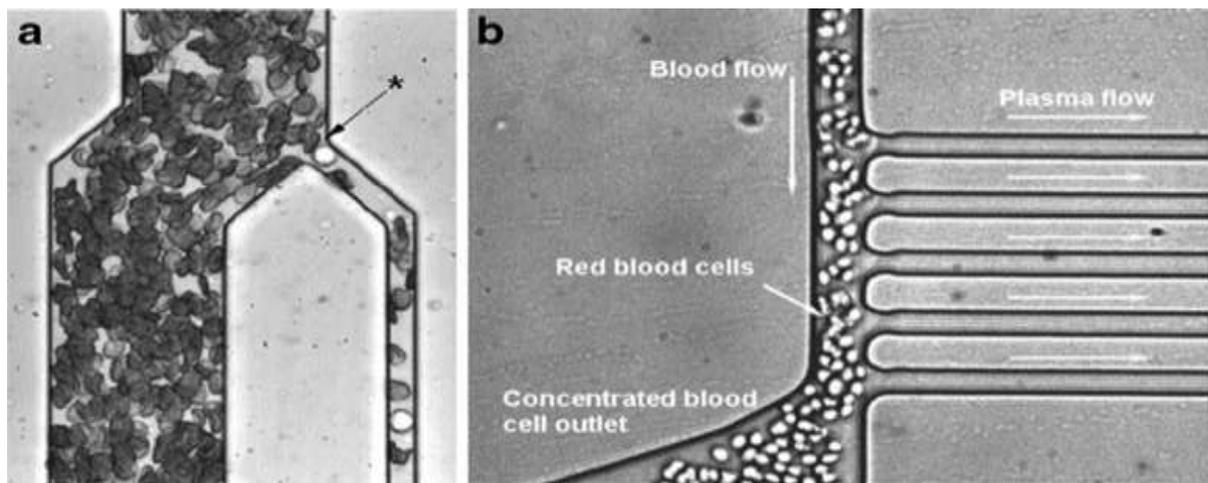
Figure 8. Example of two microfluidic devices that mimic the microvasculature. a) Leukocyte margination is used to isolate leukocytes (\*) as they are typically found in the near-wall regions of flow. From Shevkoplyas et al. *Anal Chem* 2005. b) Bifurcation law is manipulated to remove cell-free plasma from blood. From Yang et al. *Lab Chip* 2006.
