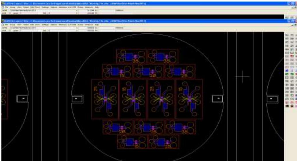
Figure 9. Wafer layout of 14 chips- 4 large chips for 4-way communication experiment and 10 small chips for 2-way communication experiment
