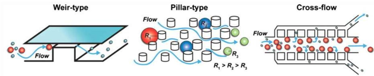
Figure 5. Schematic illustration for weir, pillar and cross-flow microfluidic filters. From Gossett et al. *Anal Bioanal Chem* 2010.
