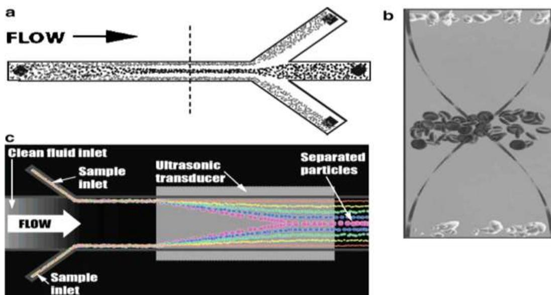
Figure 4. Acoustic separation. The acoustic radiation force may be manipulated for density-based, equilibrium separation (a, b) From Laurell et al. *Chem Soc Rev* 2007. or size-based kinetic separation (c). From Petersson et al. *Anal Chem* 2007.
