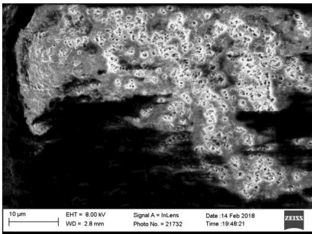
Figure 18. SEM image of nanoporous HEMA-EDMA. Scale bar 10  $\mu\text{m}$
