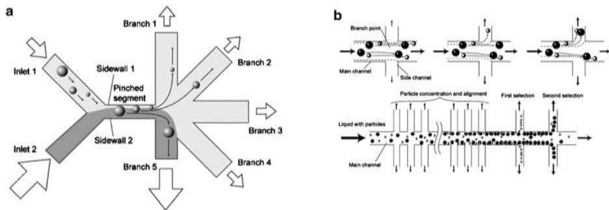
Figure 6. Hydrodynamic methods of separation. A) Pinched flow microfluidic fractionation. From Takagi et al. *Lab Chip* 2005. B) Hydrodynamic microfluidic filtration. From Yamada et al. *Lab Chip* 2005.
