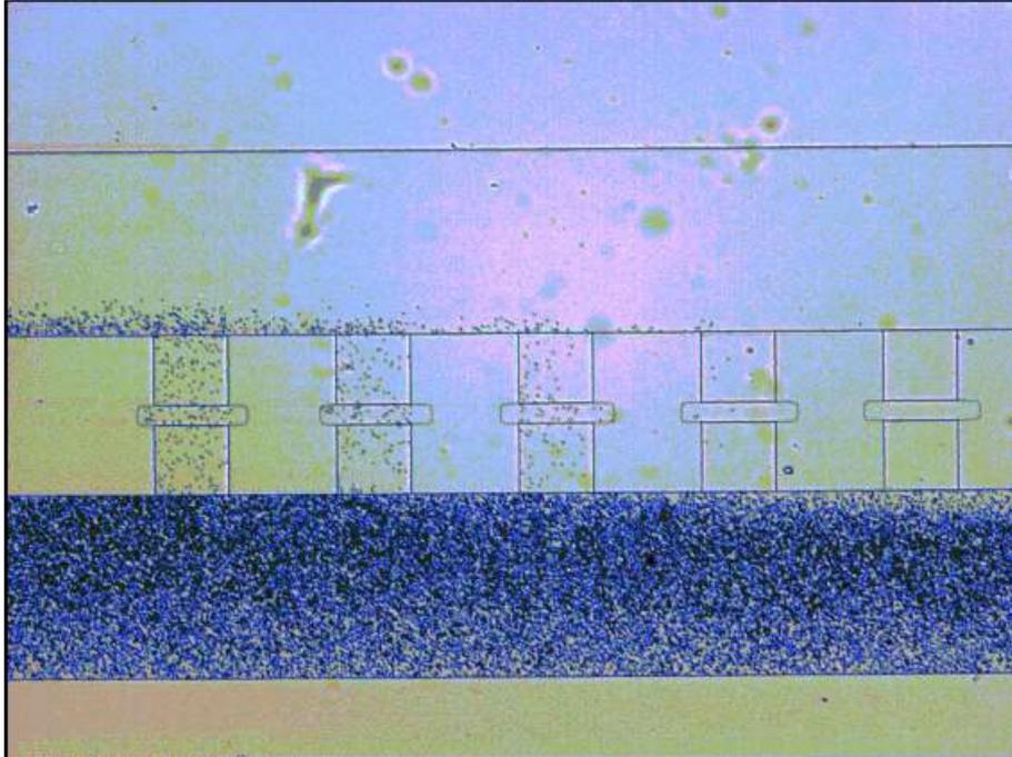
*Figure 20. filtering test in microfluidic device integrated with PEG-DA*
