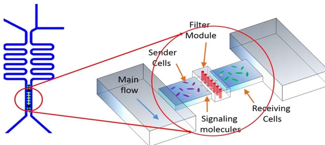
Figure 12. left: Fluidic circuit overall design, right: 3D rendering of three layers PDMS chip and functional components.
