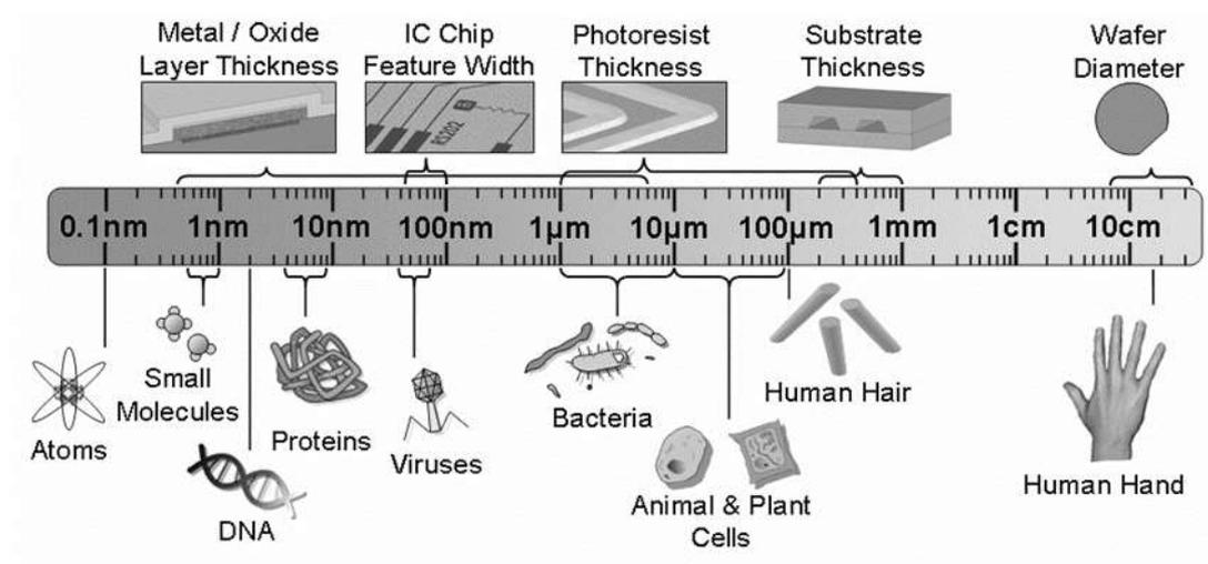
Figure 3. Approximate length scales for several biological and micro-fabrication structures.
