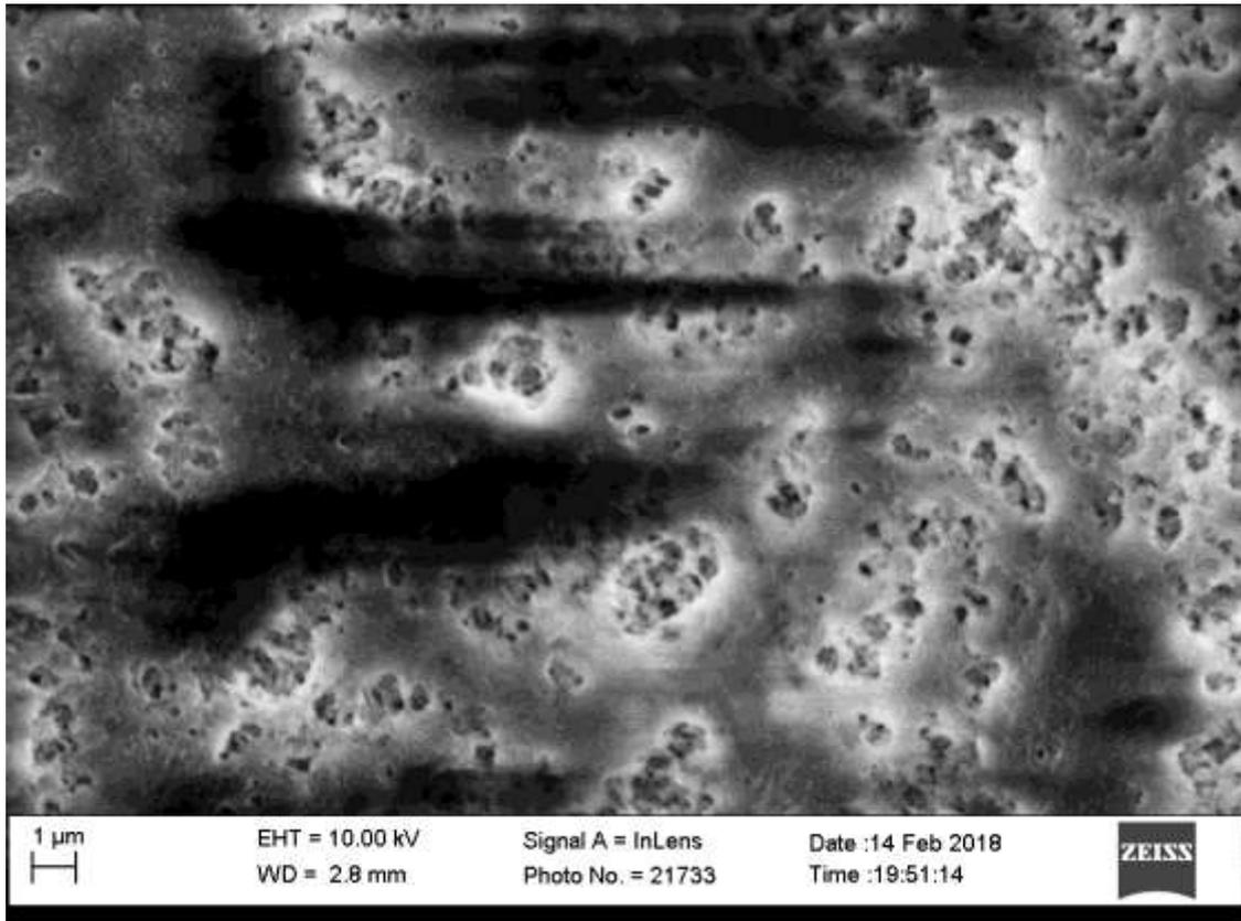
*Figure 19. SEM image of nanoporous HEMA-EDMA. Scale bar 1 μm*
