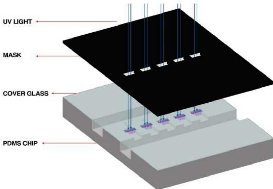
Figure 13. exposure arrangement via a dark photomask (focusing in the filtering area)
