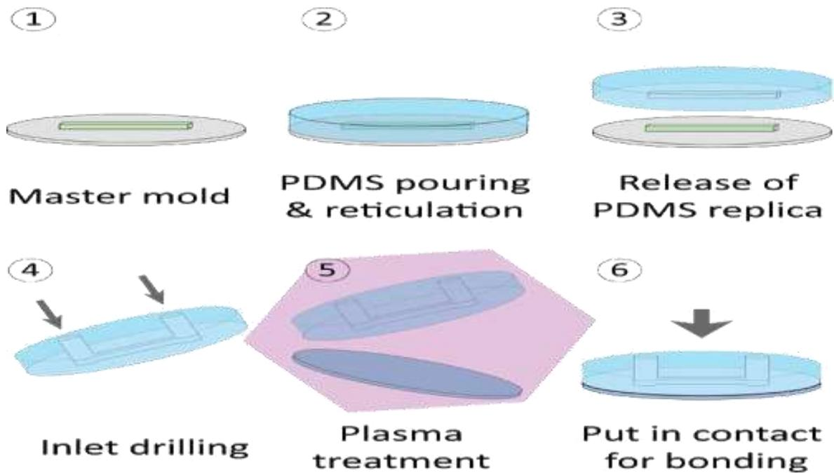
Figure 13. fabrication of a microfluidic chip by soft-lithography methods
