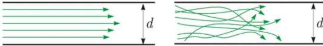
Figure 1: Microfluidics laminar (left) vs Turbulent flow (right)
