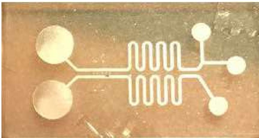
*Figure 14. Assembled PDMS-GLASS microfluidic chip*
