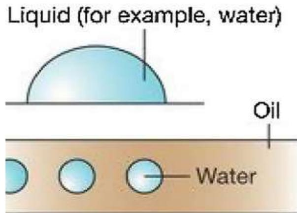
Figure 2. Surface and interfacial tension in microfluidics
