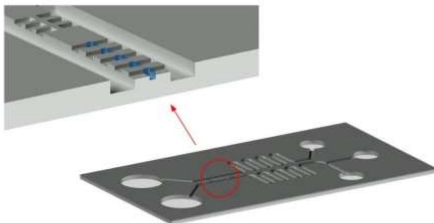
Figure 17. Microstructure filter membrane in the anchor region
