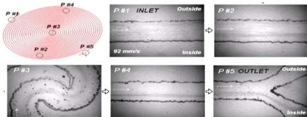
Figure 7. Example of an inertial microfluidic technique. From Seo et al. *Appl Phys Lett* 2007.
