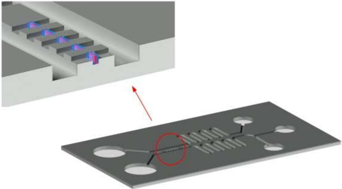
Figure 21. final layout of the microfluidic chip with Micro-pillar array in the anchor region
