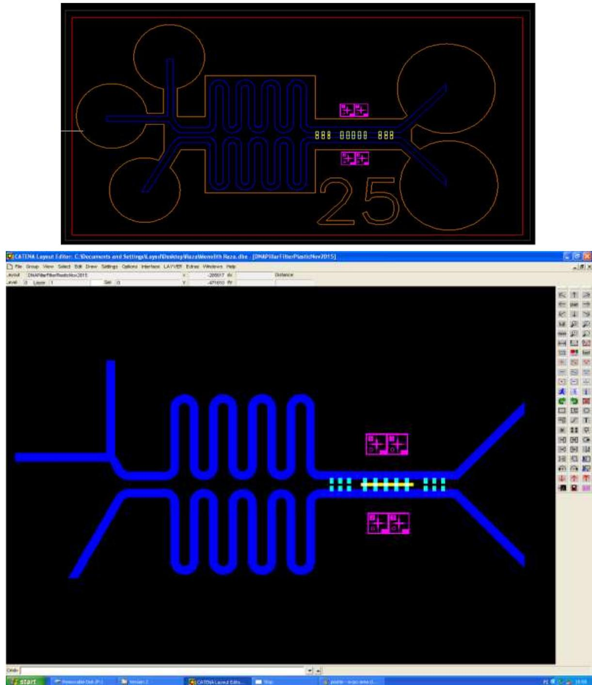
Figure 10. two-way communication microfluidic mask design (Top figure) and hydrogel layout (bottom figure, yellow part)
