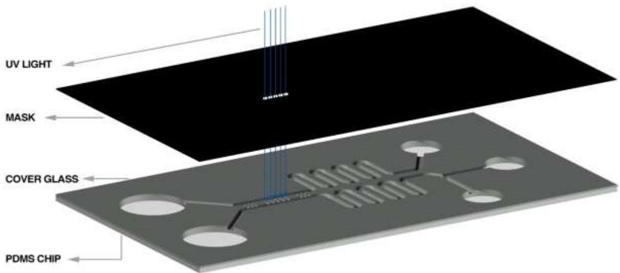
Figure XX. Figure 12. Exposure arrangement via a dark photomask patterning hydrogel blocks after hydrogel loaded
