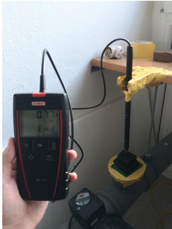
*Figure 25. Placement of the anemometer probe in the duct center.*
