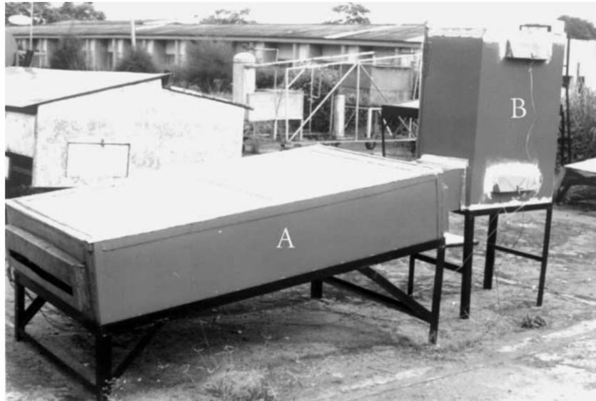
Figure 6. Photograph of the system. A, solar air collector and energy storage; B, heated space[21].
