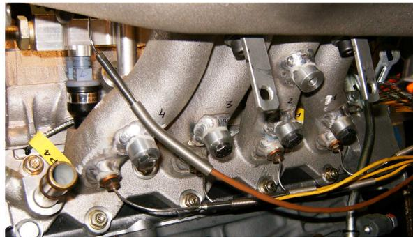
Figure 3.6: Intake pressure transducers location
