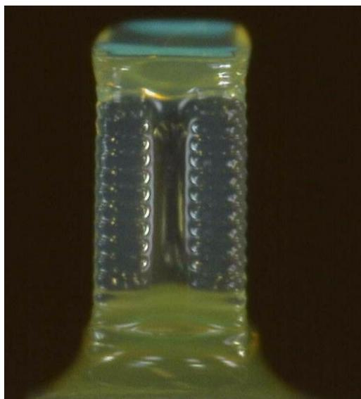
(a) Over hanging structure fabricated with HTM140-V2 resin.
