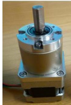
Figure 5.12 A geared stepper motor used in built P $\mu$ SLA.
