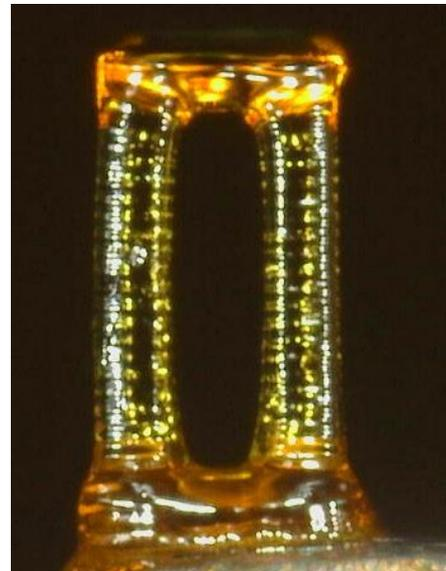
(b) Over hanging structure fabricated with laboratory made resin.
