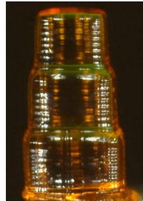
(b) Fabricated structure consisting 30  $\mu\text{m}$  thick layers followed by a base layer and squares of sizes 300x300, 250x250 and 200x200 pixels.
