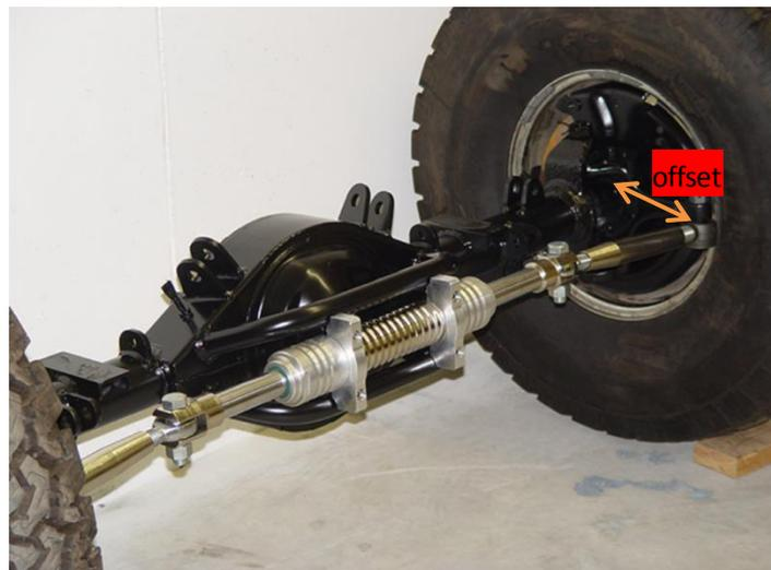
Figure 4.1.3.1 Double acting steering cylinder
