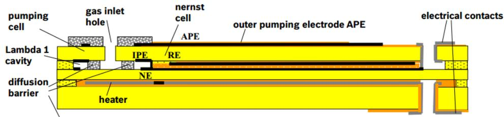
Fig. 44 – Sensing element detail
