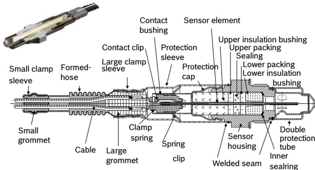
Fig. 43- Oxygen sensor section. Major components are evidenced.
