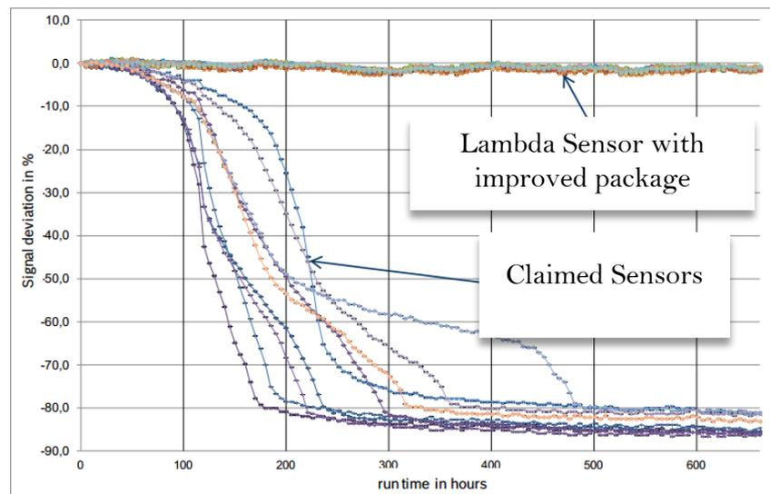
Fig. 60 – Signal deviation in component air test
