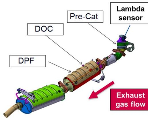
Fig. 42- Upstream Oxygen sensor
