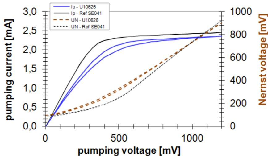
Fig. 47 – Pumping current drifting respect to pumping voltage
