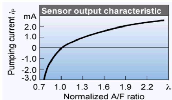
Fig. 45– Output pumping current characteristic
