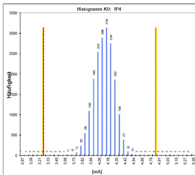
End of line test must be performed on 100% of the production lot for a certain amount of time. This test consists in verify the pumping current electrical characteristic of the sensing element. The Fig. 54 diagram, shows the distribution of the tested components.
