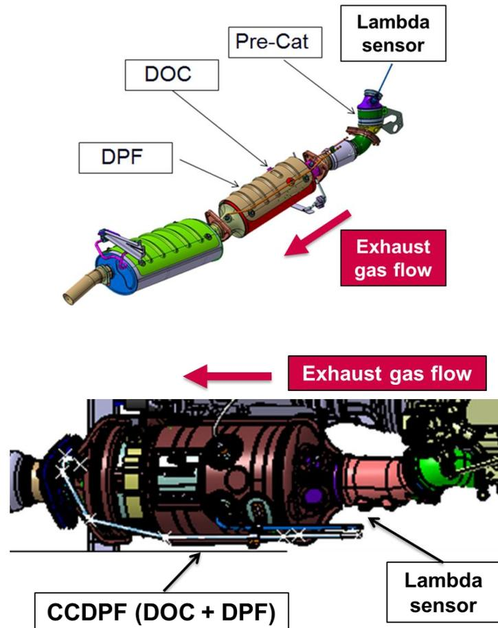
Fig. 32- ATS Layout – Oxygen sensor detail
