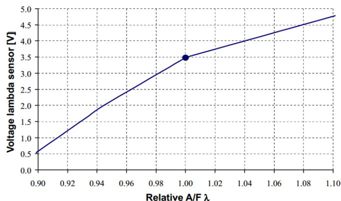
Fig. 34 - Output voltage trend respect to A/F ratio
