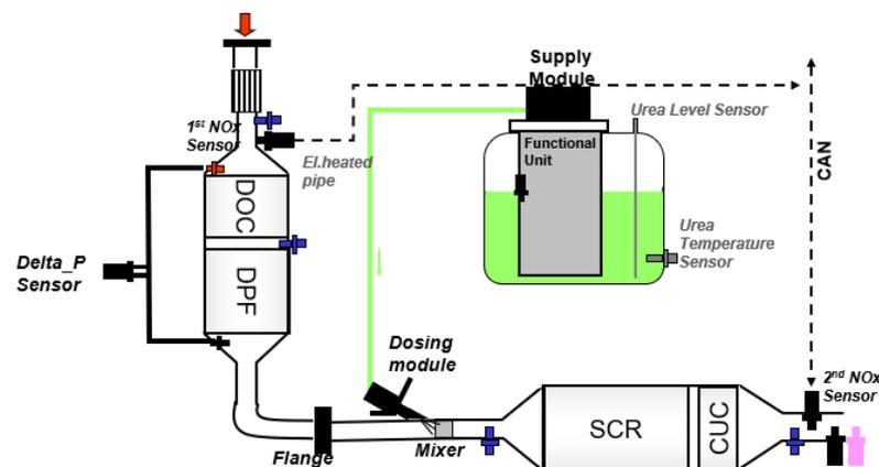
Fig. 31- Exhaust Gas ATS layout
