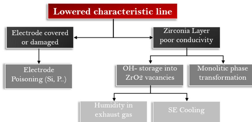
Fig. 49 – Failure tree flow chart
