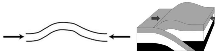
Figure 2.2: Buckling – Loading schema on the left and a tectonic-scale example.
