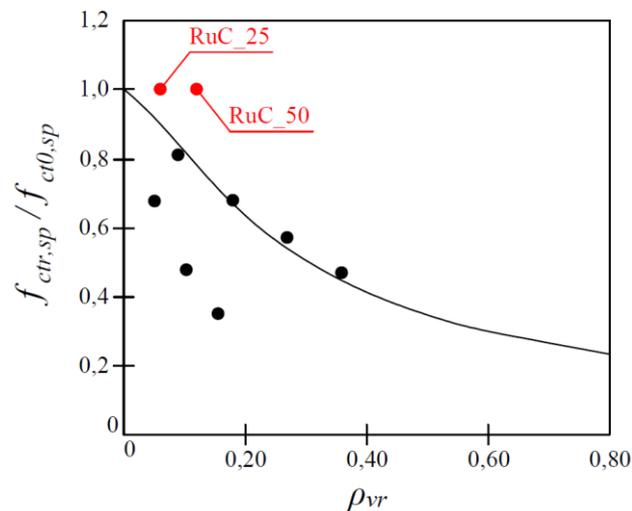
**Fig. 62** – Tensile strength degradation comparison between relationship obtained by Bompa *et al.* and results purposed in this work
