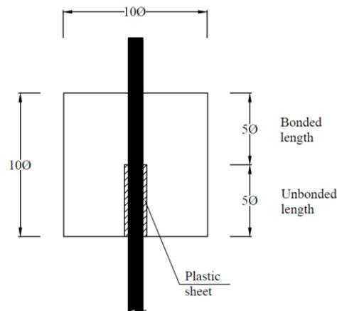
**Fig. 39** – Pull-out test specimen ( $\Phi$  is bar diameter)
