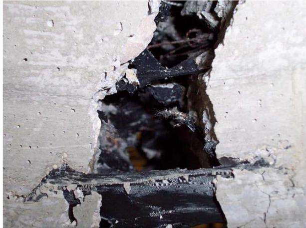
**Fig. 21** – Particular of the cracked section of a specimen after a flexural strength test (Aiello and Leuzzi, 2010)
