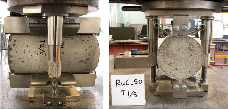
Fig. 44 – Splitting tensile strength test setup
