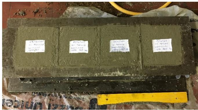
**Fig. 31** – Casting of trial concrete mixture cubic specimens
