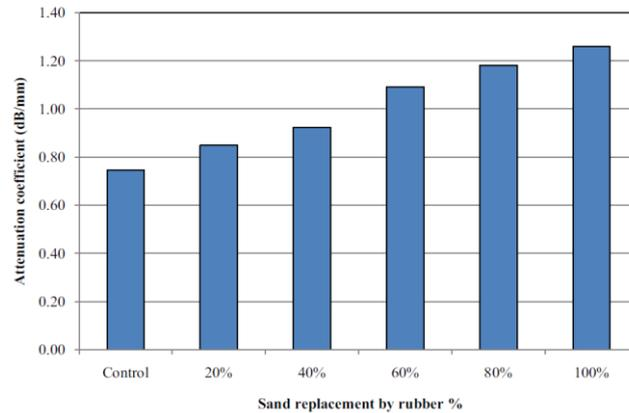
**Fig. 22** – Attenuation coefficient of conventional concrete and rubberized concrete at different percentages of sand replacement (Aliabdo, Abd Elmoaty and Abdelbaset, 2015)
