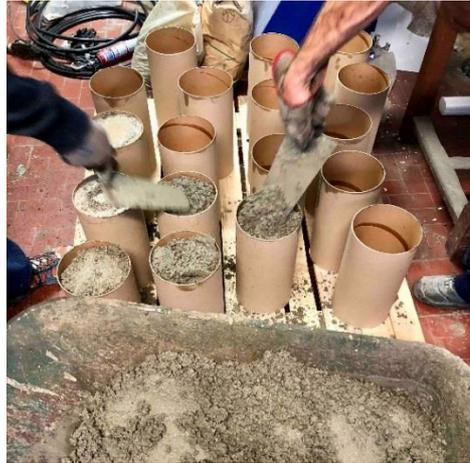
**Fig. 36** – Preparation of cylindrical samples in cardboard formworks
