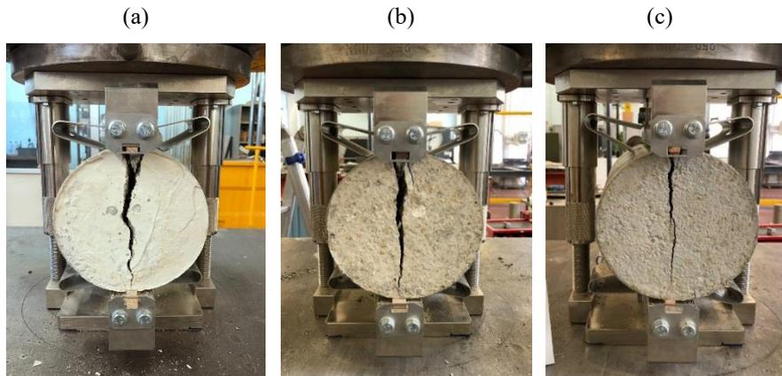
**Fig. 52** – Specimen after failure in splitting tensile test: a) RuC\_0, b) RuC\_25, c) RuC\_50
