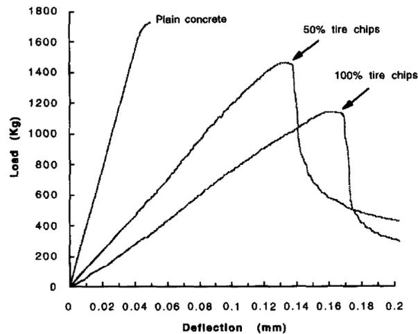
Fig. 20 – Load-deflection curves for plain and rubber tyre concrete beams (Toutanji, 1996)
