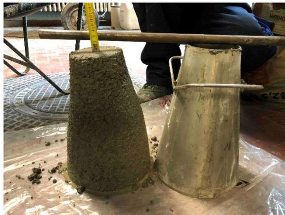
**Fig. 41** – Slump test on mixture RuC\_75
