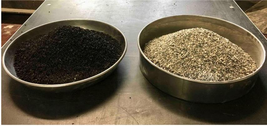
**Fig. 34** – Substitution between fraction 2-4mm of crumb rubber and river sand equivalent in volume
