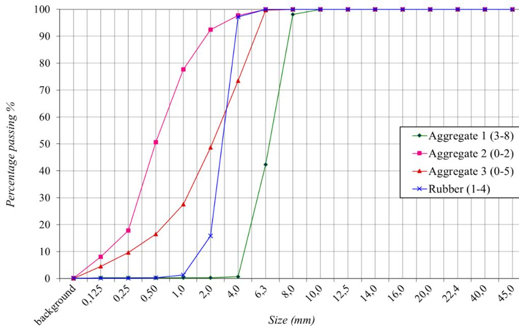
**Fig. 29** – Sieve analysis comparison between natural aggregates and waste rubber aggregate
