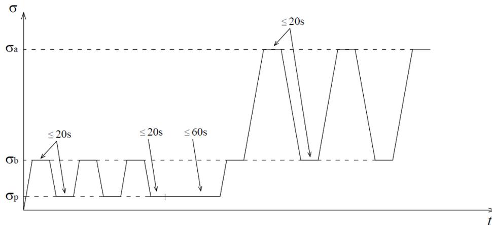
**Fig. 43** – Experimental determination of modulus of elasticity (UNI EN 12390-13, 2013)
