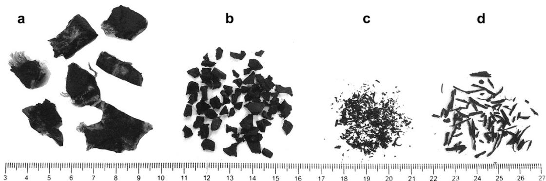
**Fig. 12** – Classification of rubber aggregates: (a) chipped, (b) crumb, (c) granular and (d) fibre (Najim and Hall, 2010).
