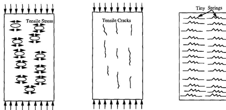
Fig. 17 – Modeling of rubberized concrete with chipped rubber as gravel replacement under compression (Eldin and Senouci, 1993)
