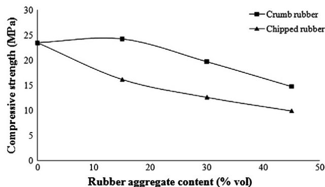
**Fig. 8** – Compressive strength loss in concrete with rubber particle (Najim and Hall, 2010)
