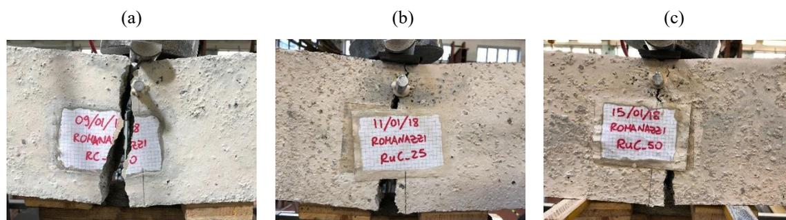
**Fig. 55** – Beams after failure three points bending tests: a) RuC\_0, b) RuC\_25, c) RuC\_50
