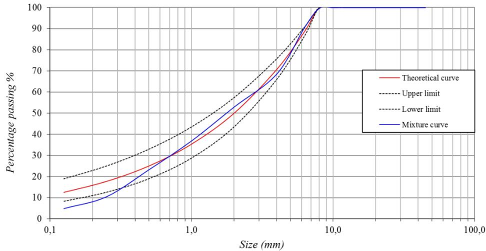
**Fig. 27** – Fuller mix optimization of the three natural aggregates
