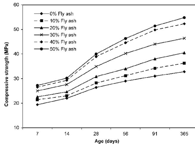
**Fig. 6** - Compressive strength versus age in fly ash concrete (Siddique, 2003)
