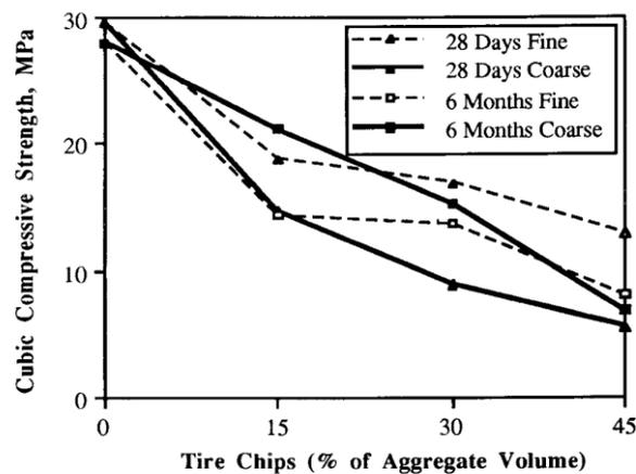
**Fig. 16** – Changes in cubic compressive strength with the amount of rubber content (Topçu, 1995)
