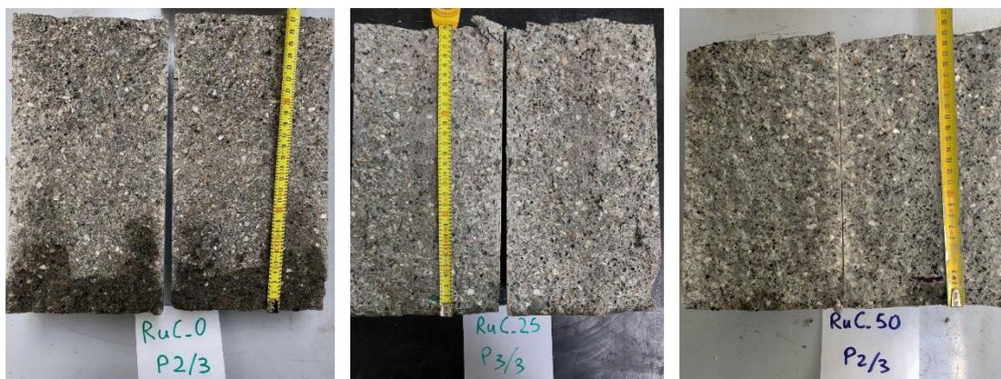
Fig. 60 – Water penetration measurement after permeability test
