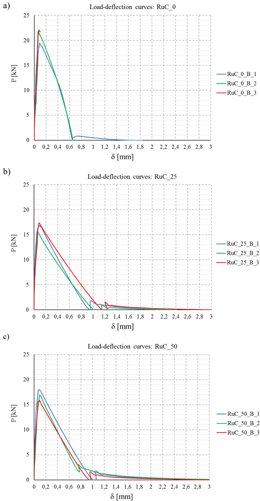
**Fig. 56** – Load-deflection curves for a) normal concrete RuC\_0, b) rubberized concrete with 6% replacement RuC\_25, c) rubberized concrete with 12% replacement RuC\_50
