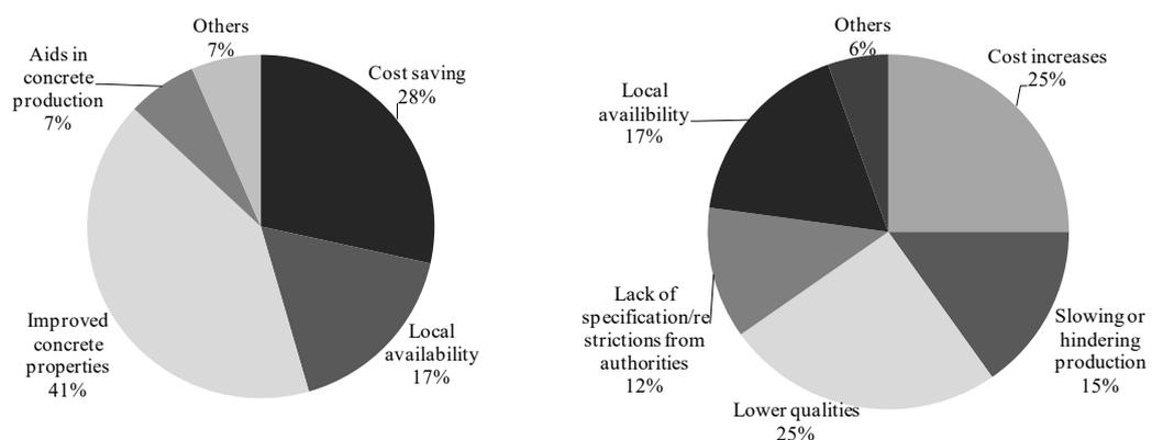
**Fig. 4** - Benefits and barriers of using waste material as partial replacement of cement (Jin and Chen, 2013)
