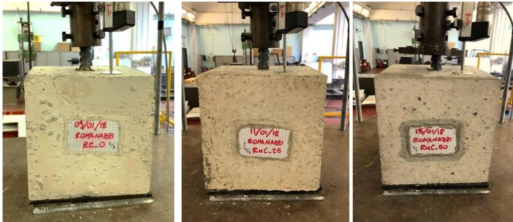
Fig. 59 – Specimen of the three concrete mixtures after pull-out failure
