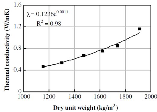
**Fig. 23** – Relationship between thermal conductivity and dry unit weight (Benazzouk *et al.*, 2008)
