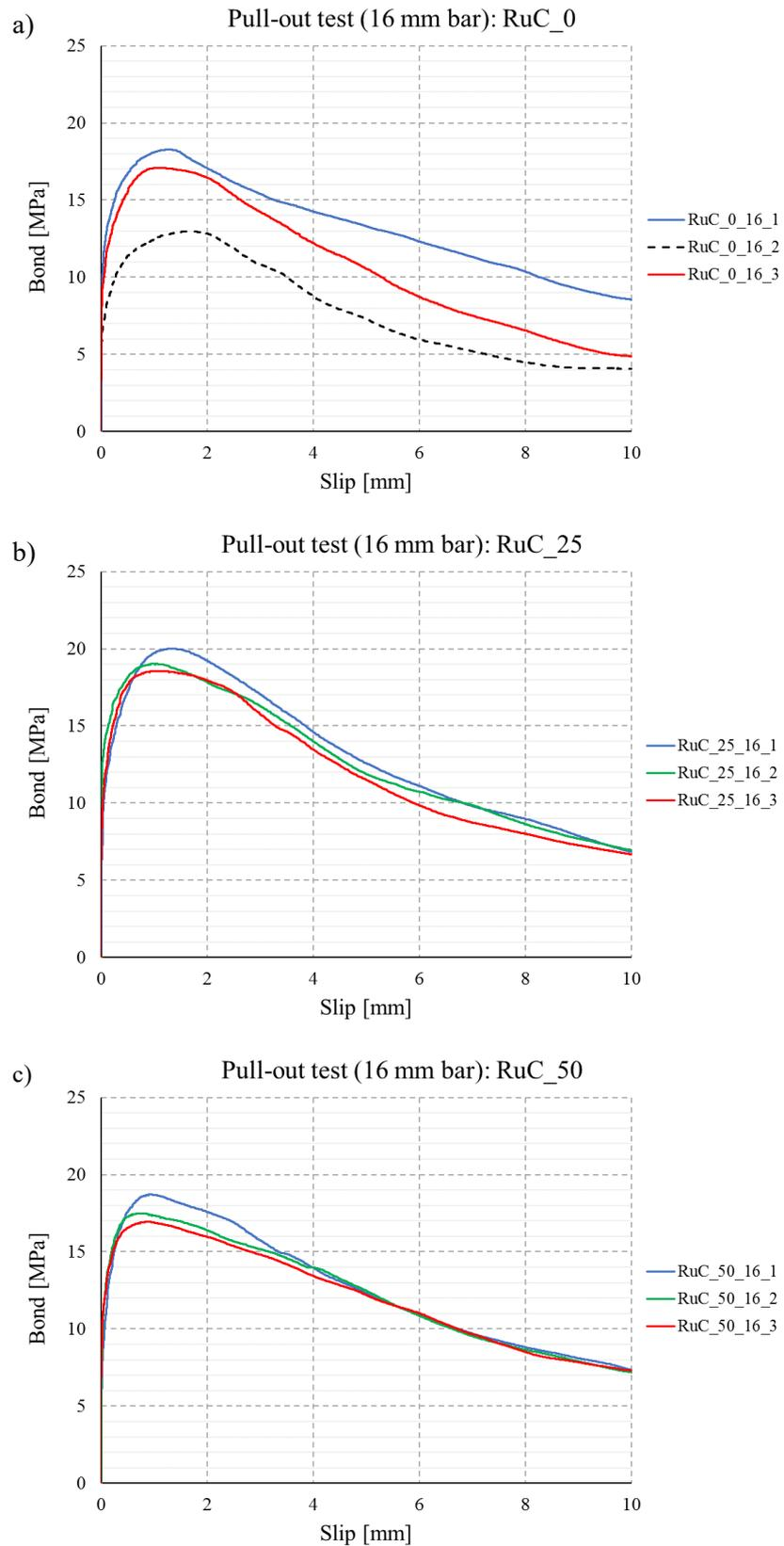
**Fig. 58** – Bond-slip behavior for specimen with 16 mm embedded deformed bar: a) normal concrete RuC\_0, b) rubberized concrete with 6% replacement RuC\_25, c) rubberized concrete with 12% replacement RuC\_50
