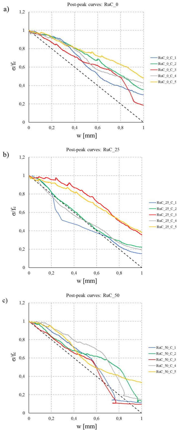
**Fig. 50** – Post-peak curves: a) control concrete mixture RuC\_0, b) rubberized concrete with 6% replacement RuC\_25, c) rubberized concrete with 12% replacement RuC\_50
