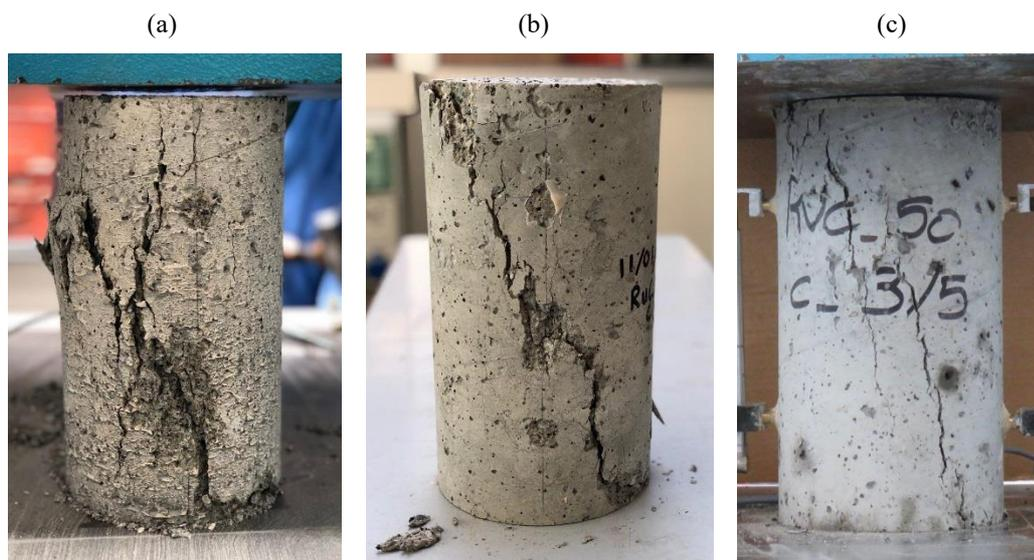
**Fig. 51** – Some of tested specimens after failure in compression: a) RuC\_0, b) RuC\_25, c) RuC\_50
