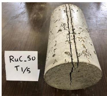
**Fig. 54** – Concrete RuC\_50 specimen after splitting tensile test
