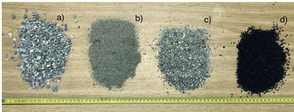
**Fig. 25** – Aggregates used in rubberized concrete: a) gravel b) fine sand c) river sand d) rubber
