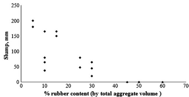
**Fig. 15** – Effect of aggregate replacement ratio on slump of rubber concrete (Najim and Hall, 2010)
