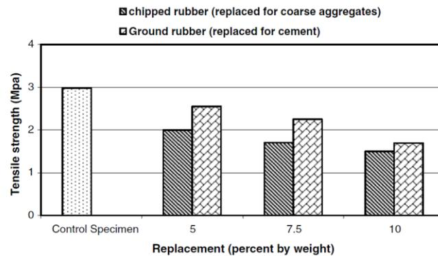
**Fig. 19** – Results of tensile strength test (Ganjian, Khorami and Maghsoudi, 2009)
