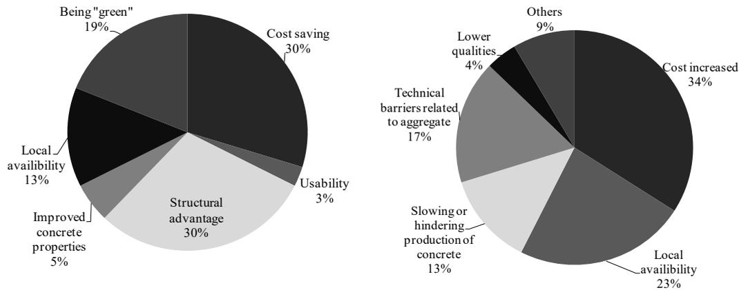
**Fig. 5** - Benefits and barriers of using waste material as alternative aggregates in concrete (Jin and Chen, 2013)
