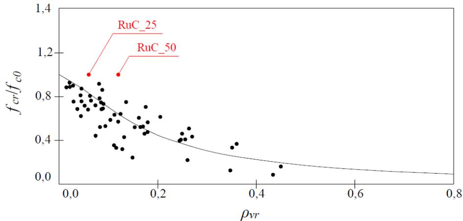
**Fig. 61** – Compressive strength degradation curve defined by Bompa *et al.* (2017) as a function of volumetric rubber ratio in case of fine aggregates replacement compared with compressive strength results obtained in this study
