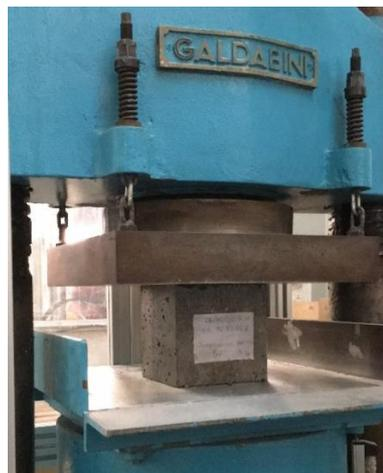
**Fig. 32** – Compression strength test on cubic sample obtained from trial mix
