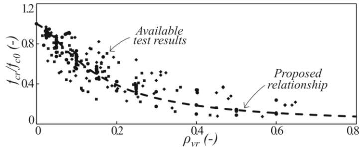
**Fig. 18** – Compressive strength as a function of volumetric rubber ratio  $\rho_{vr}$  (Elghazouli *et al.*, 2018)
