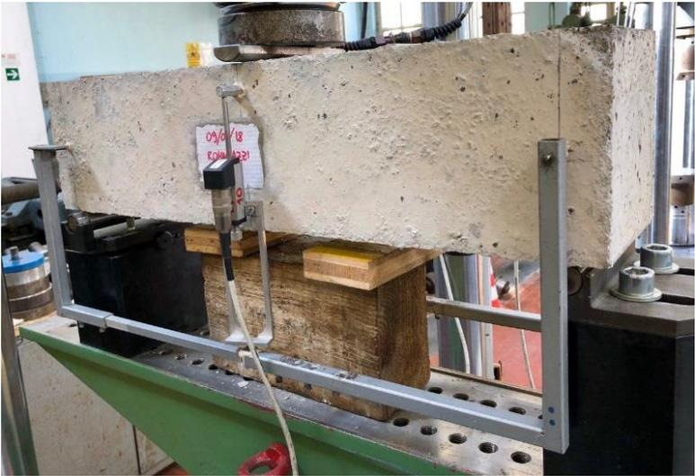
Fig. 45 – Three points bending testing arrangement
