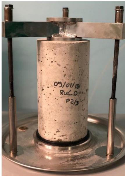
Fig. 46 – Permeability test
