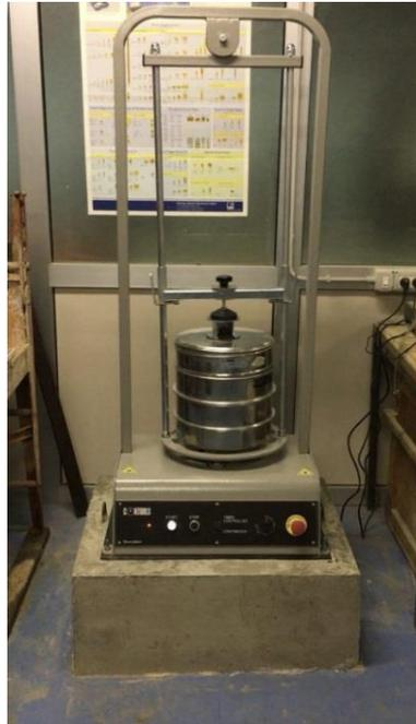
**Fig. 33** – Electromechanical sieve shaker
