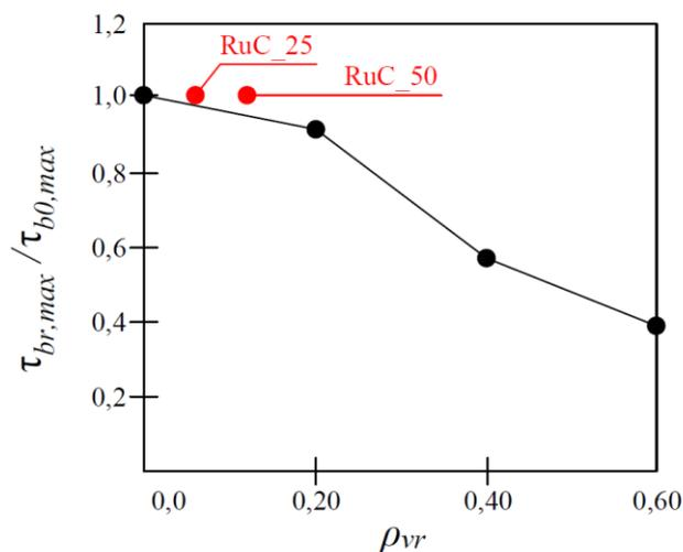
**Fig. 63** – Maximum bond stress degradation according to Bompa and Elghazouli (2017) (black markers) and results achieved in this work (red markers)
