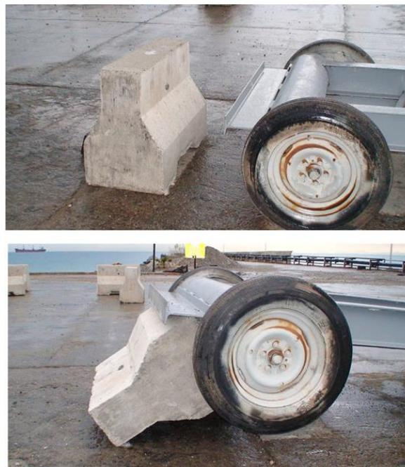
**Fig. 24** – A typical New Jersey barriers used in dynamic impact tests before and after impact (Atahan and Sevim, 2008)
