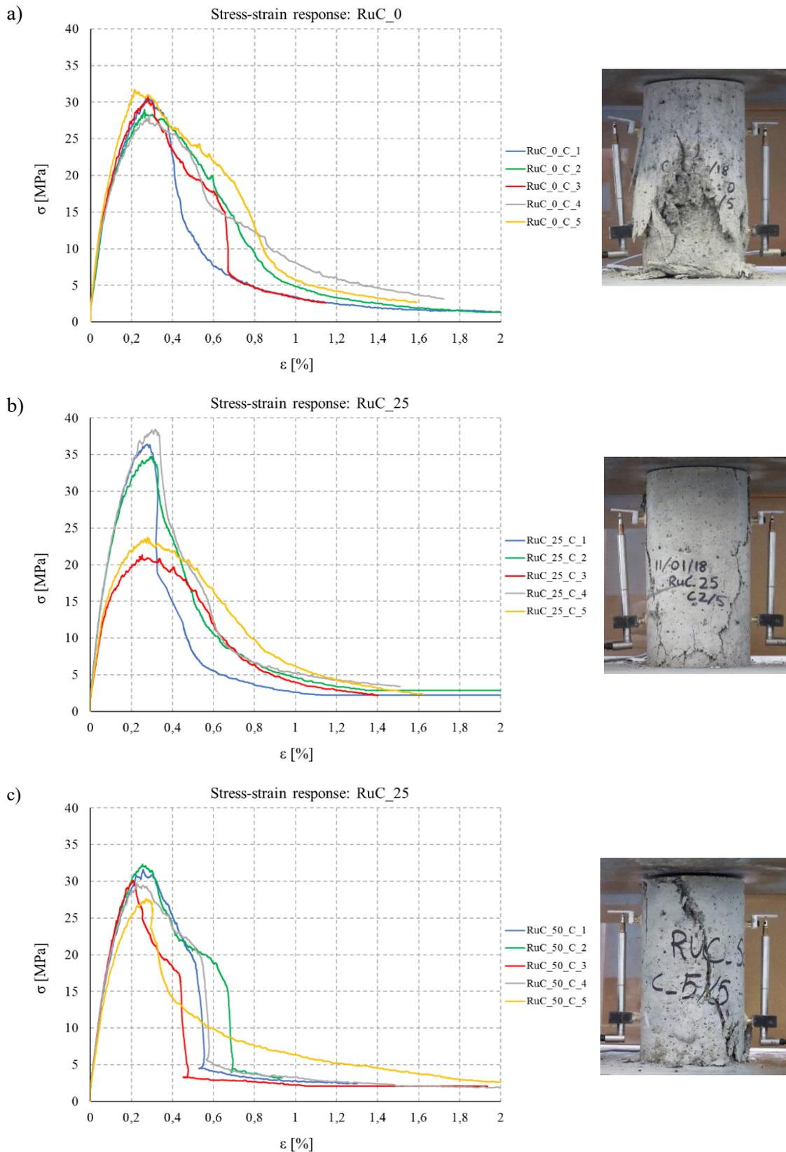
**Fig. 48** – Stress-strain relationship and specimen after failure for a) normal concrete RuC\_0, b) rubberized concrete with 6% replacement RuC\_25, c) rubberized concrete with 12% replacement RuC\_50
