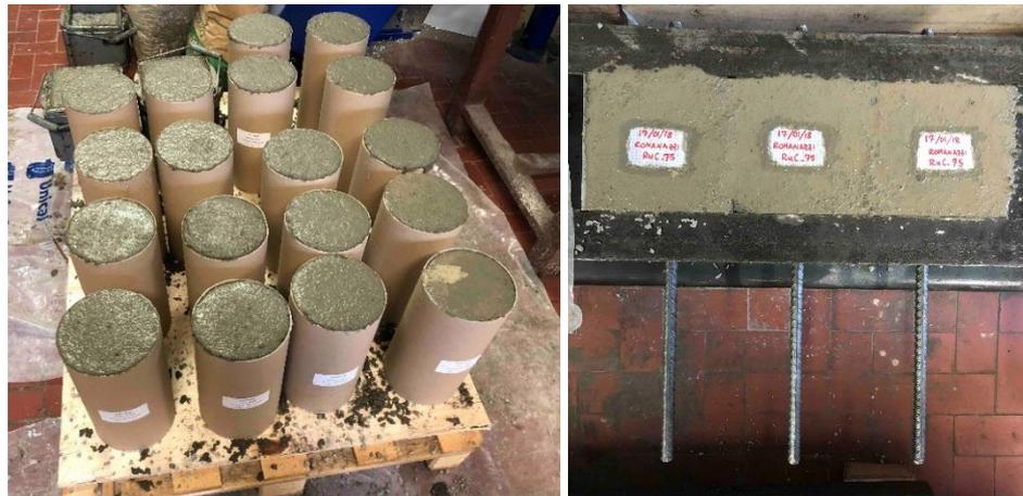
**Fig. 37** – Cylindrical specimens and pull-out test specimens just after concrete casting
