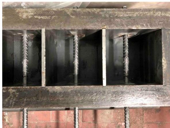
**Fig. 35** – Formworks for pull-out test cubic specimens
