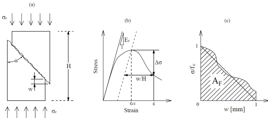
**Fig. 49** – The post-peak behavior of concrete cylinders under compression: a) kinematic variables involved during failure, b) idealized stress-strain relationship, c) Post-peak response in terms of relative stress vs. inelastic shortening  $w$
