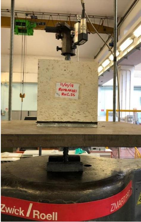
Fig. 47 – Pull-out test configuration
