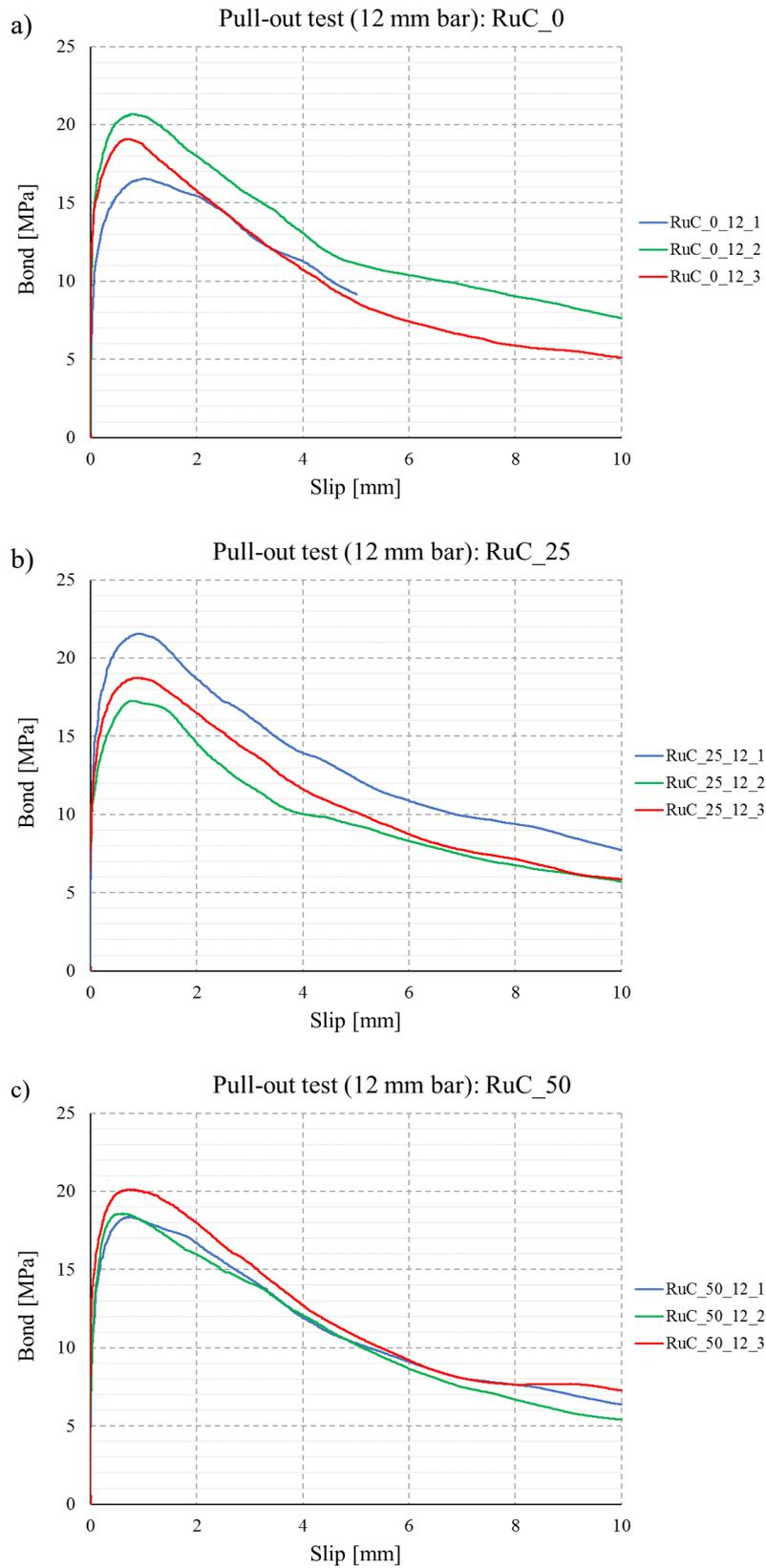
**Fig. 57** – Bond-slip behavior for specimen with 12 mm embedded deformed bar: a) normal concrete RuC\_0, b) rubberized concrete with 6% replacement RuC\_25, c) rubberized concrete with 12% replacement RuC\_50
