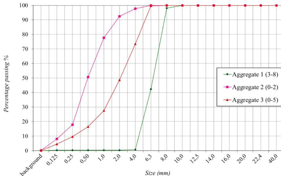
Fig. 26 – Sieve analysis for Aggregate 1, Aggregate 2 and Aggregate 3
