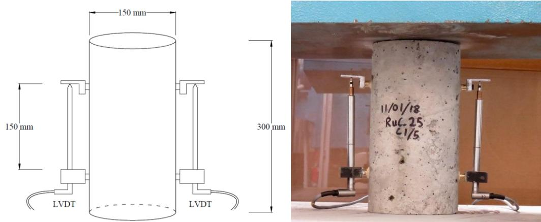
**Fig. 42** – Compressive strength test configuration
