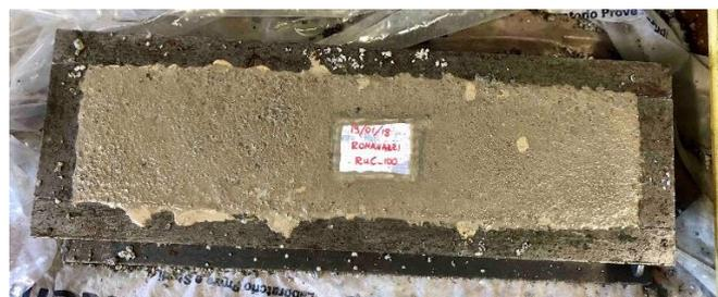
**Fig. 40** – Beam just after rubberized concrete casting
