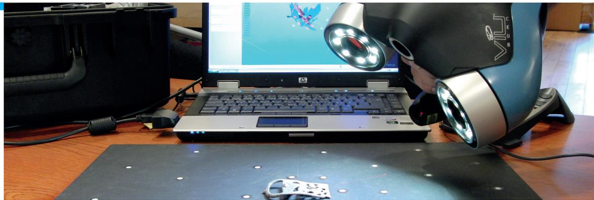
Scansione 3D manuale con VIU Scan, scanner non-contact a Structured Light Triangulation
