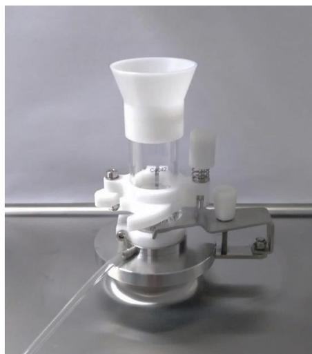
**Figure 2.36:** Example of vessel with aeration base connected to the aeration unit.
