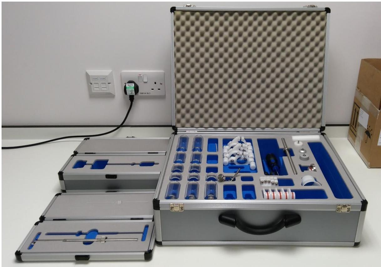
**Figure 2.24:** FT4 Powder Rheometer accessories.
