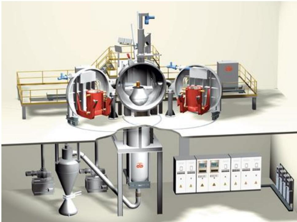
**Figure 1.18:** Schematics of a VIGA system. [12]
