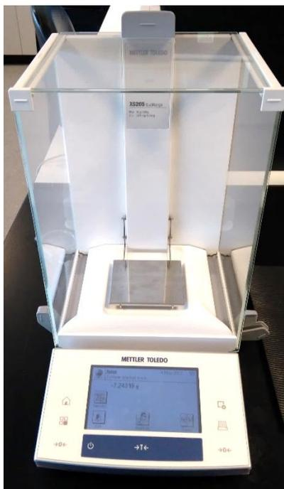
**Figure 2.6:** XS205 analytical balance.
