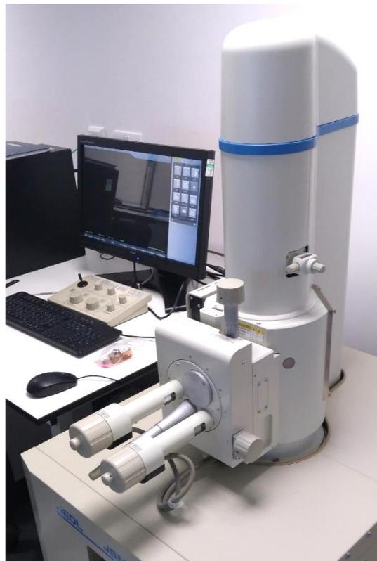
**Figure 2.1:** JSM-6010PLUS/LA electron microscope.
