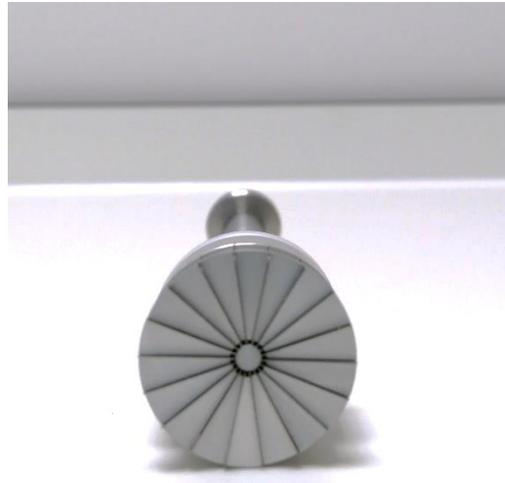
**Figure 2.32:** Shear cell head compression face.
