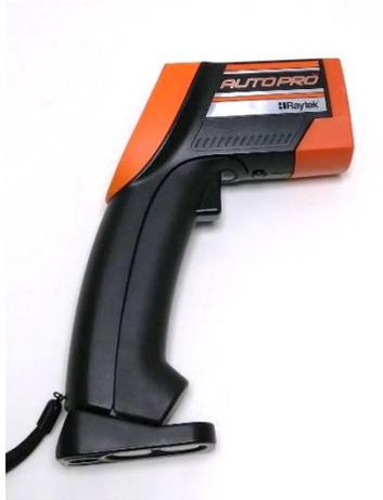
**Figure 2.15:** Infrared thermometer.
