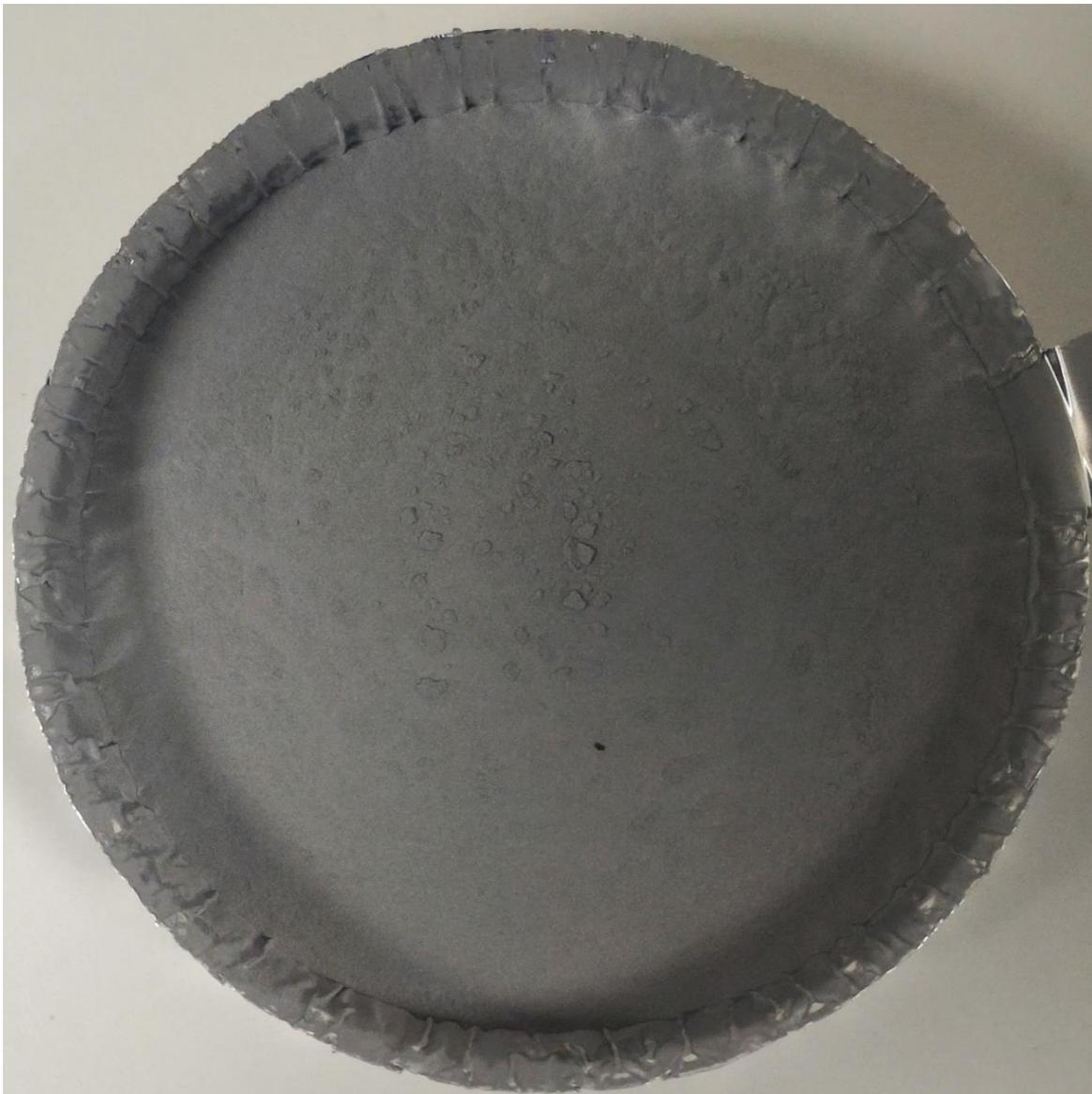
**Figure 4.8:** Agglomeration on V 15-6053S sample surface after the moisture content test.
