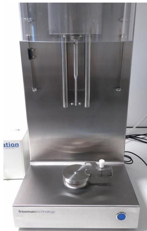
**Figure 2.26:** 23.5 mm Blade inserted in the machine.
