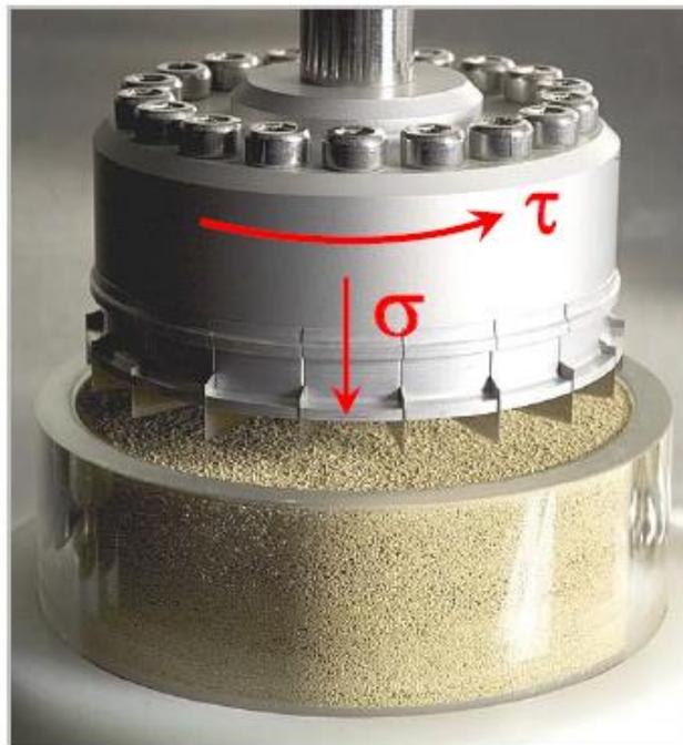
**Figure 2.57:** Shear head and applied stresses (Courtesy of Freeman Technology). [44]
