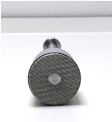
**Figure 2.28:** Vented piston compression face.
