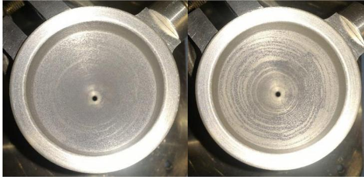
**Figure 3.34:** Powder residue of L UK3359 in the Hall funnel.
