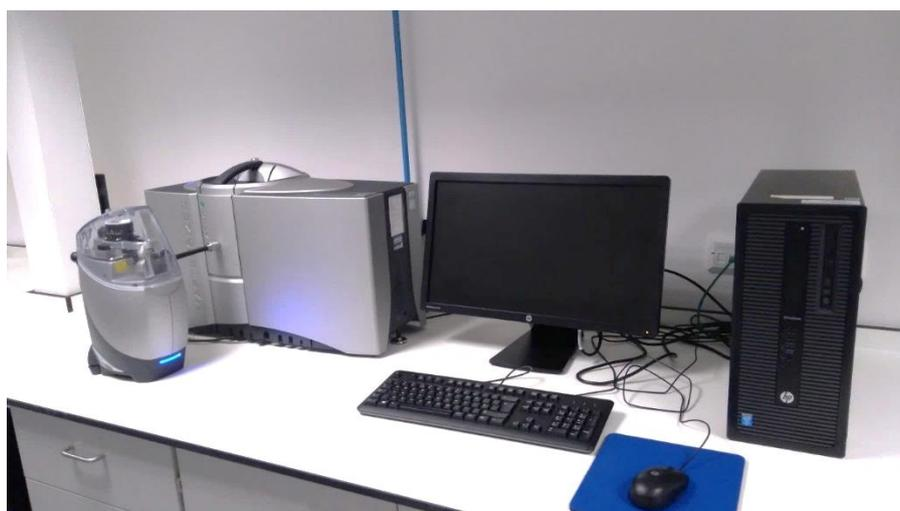
**Figure 2.10:** Mastersizer 3000 and Aero S unit.
