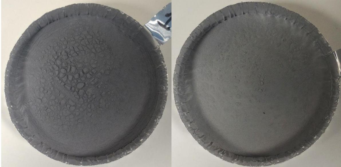
**Figure 4.9:** Agglomeration comparison between V 14-5034S (AlSi10Mg, left) and V 15-6053S (A205, right).
