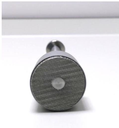
**Figure 2.28:** Vented piston compression face.
