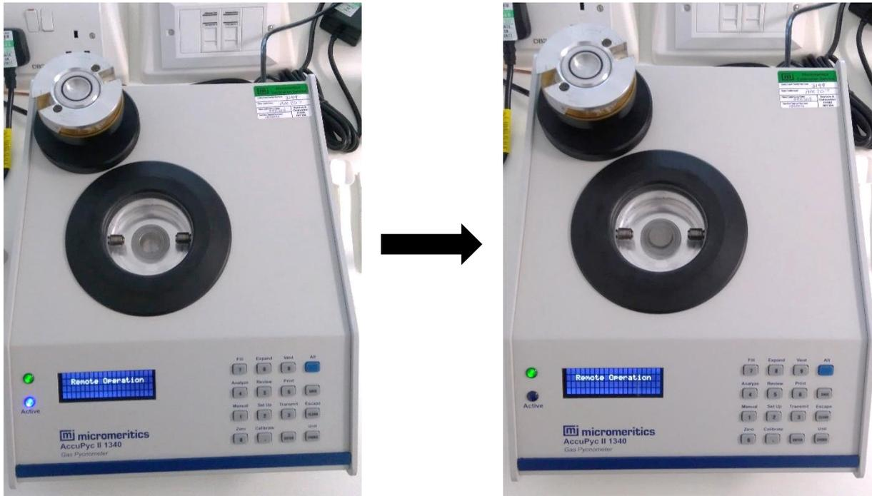
**Figure 2.8:** Pycnometer before (left) and after (right) the chamber has been slotted.
