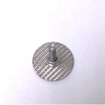
**Figure 2.29:** Metallic mesh, part of the vented piston.
