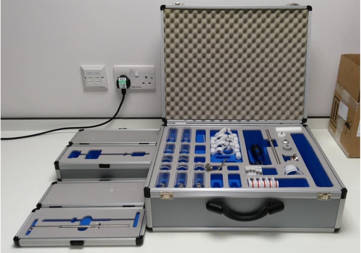
**Figure 2.24:** FT4 Powder Rheometer accessories.
