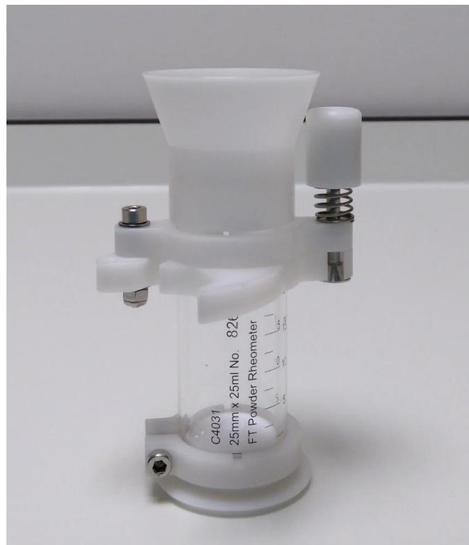
**Figure 2.33:** One of the several vessels that are used during an FT4 test.
