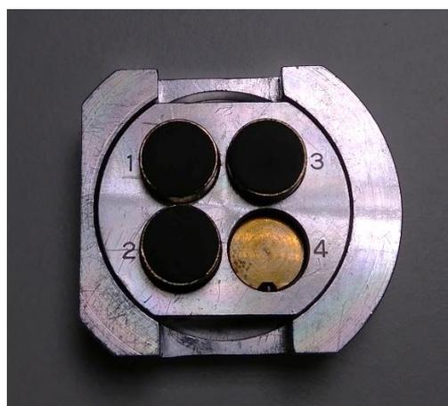
**Figure 2.3:** Sample holder with 3 brass cylinders and relative powder slotted in.
