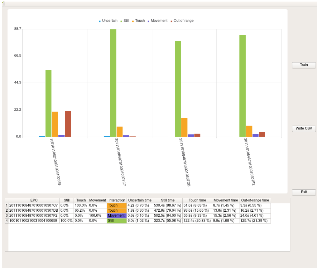
Figure 15.13: The user interface. blue is the “uncertain” response, green is “still”, orange is “touch” and violet is “movement” and brown is “out of range”
