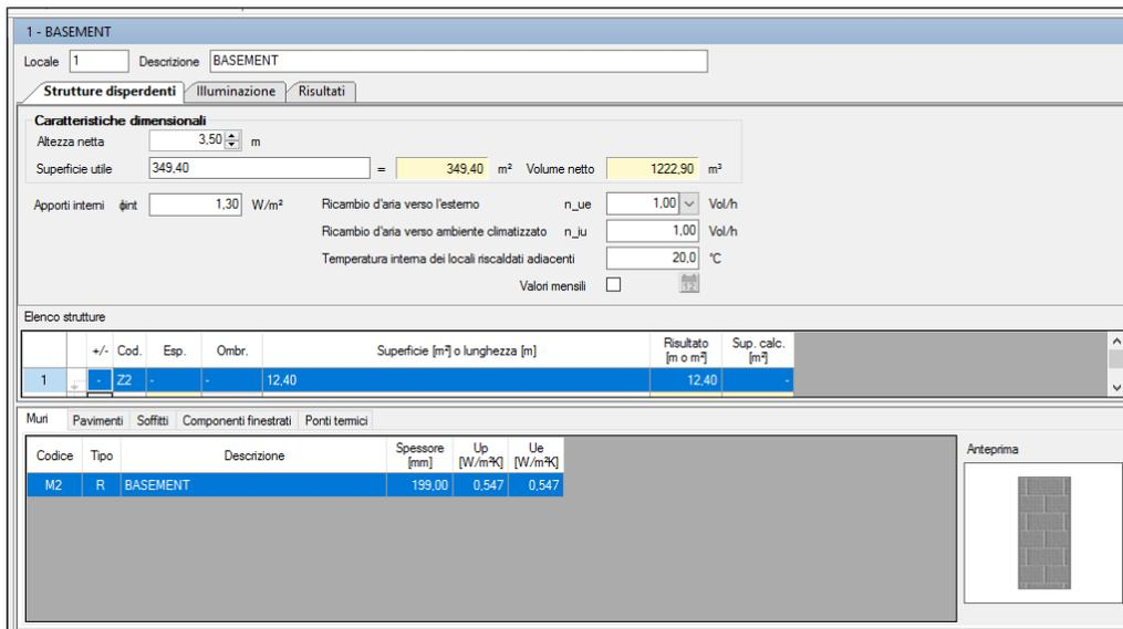
6.61 – Basement as an unconditioned room and its results (down).
