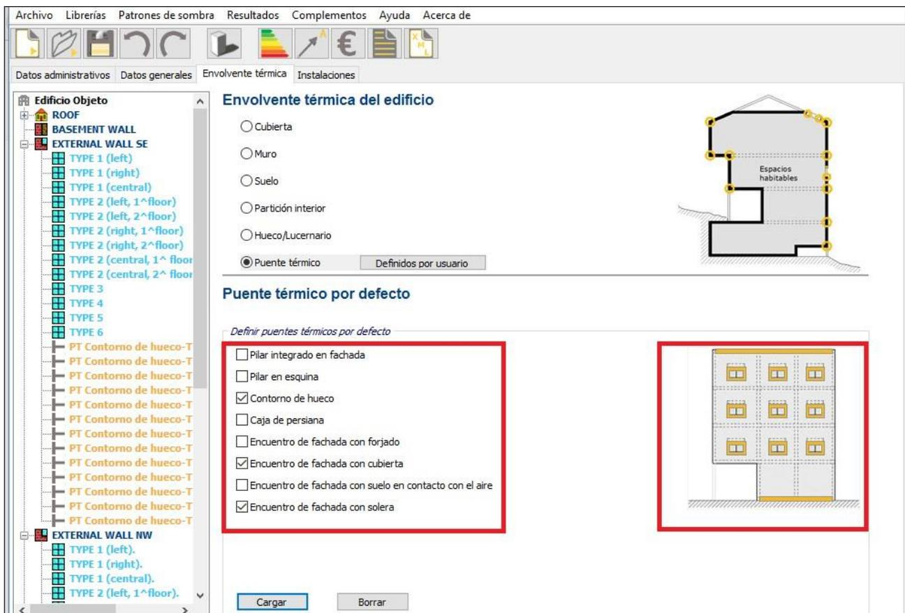
Figure 6.41 – Thermal bridge that still remain in the façade
