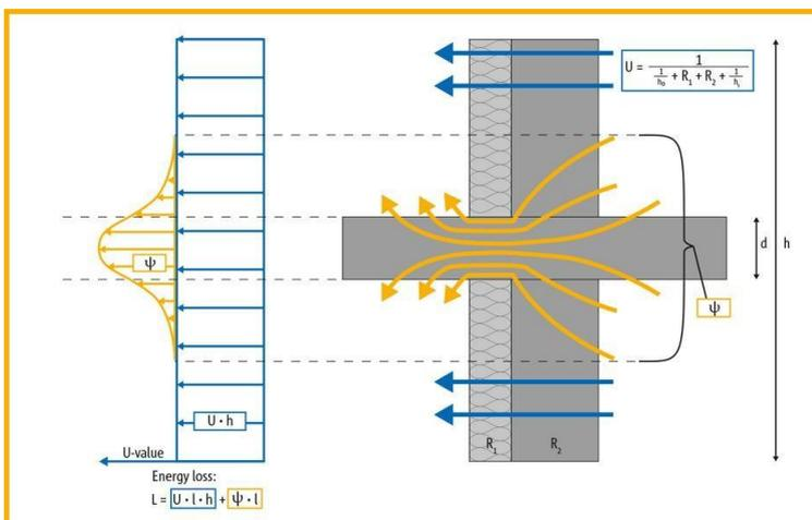
Figure 3.22 – En example of Thermal bridge
