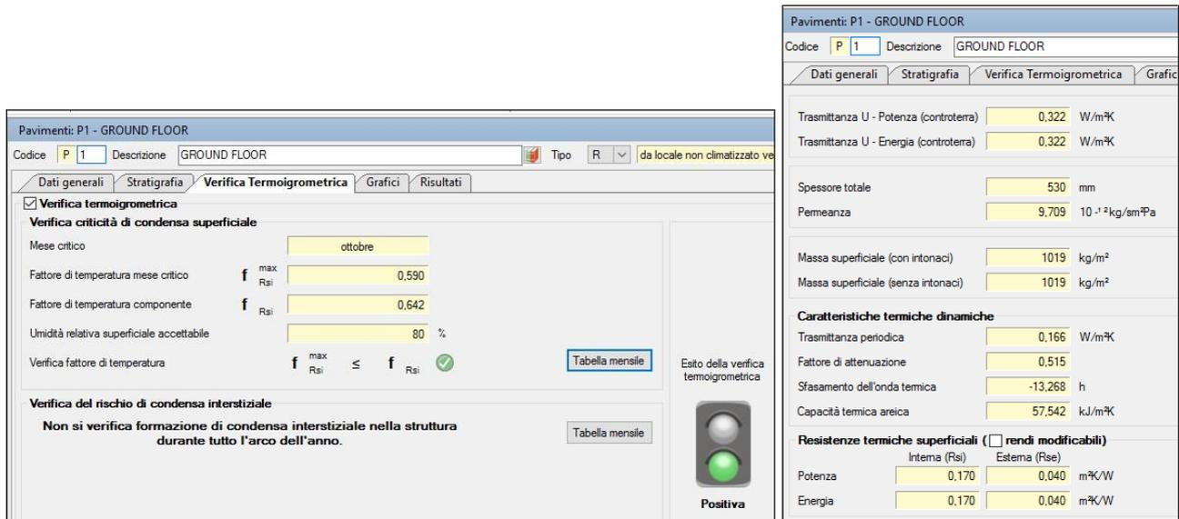
6.56 – Hygrothermal verification (left) and Transmittance value (right)
