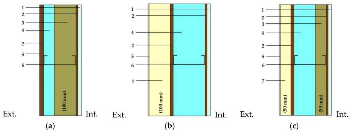
Figure 3.24 – (a) cold frame construction; (b) warm frame construction; (c) hybrid frame construction.
