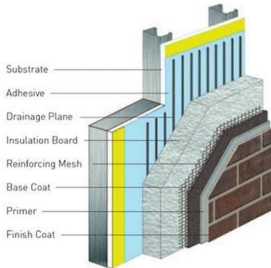
Figure 3.25 – Façade with Exterior Insulation
