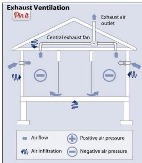
Exhaust ventilation systems are most applicable in cold climates. In climates with warm, humid summers, depressurization can draw moist air into building wall cavities, where it may condense and cause moisture damage.
