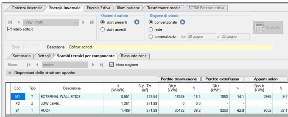
6.69 – Thermal exchange of opaque element
