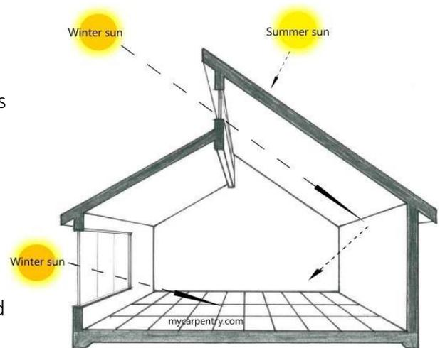
Figure 3.2 – Direct gain passive solar Energy.
