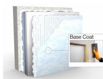
Polymer modified dry-mix mortar is applied to secure the glassfiber mesh. The mortar makes for a composite base that is both secure and flexible.
