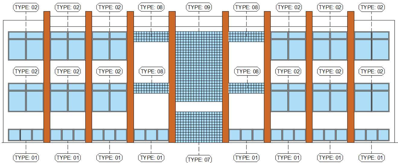
Figure 6.14 – Scheme of type of windows. North-West Façade
