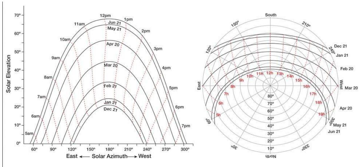
Figure 3.18 - Solar Chart (cylindrical diagram on left and polar diagram on right)
