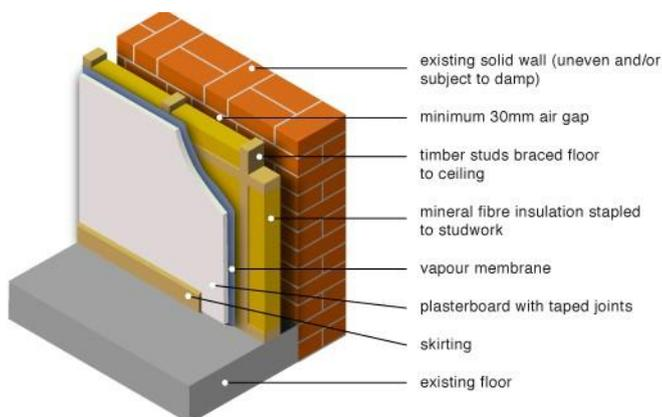
Figure 3.26 – Façade with Internal Insulation
