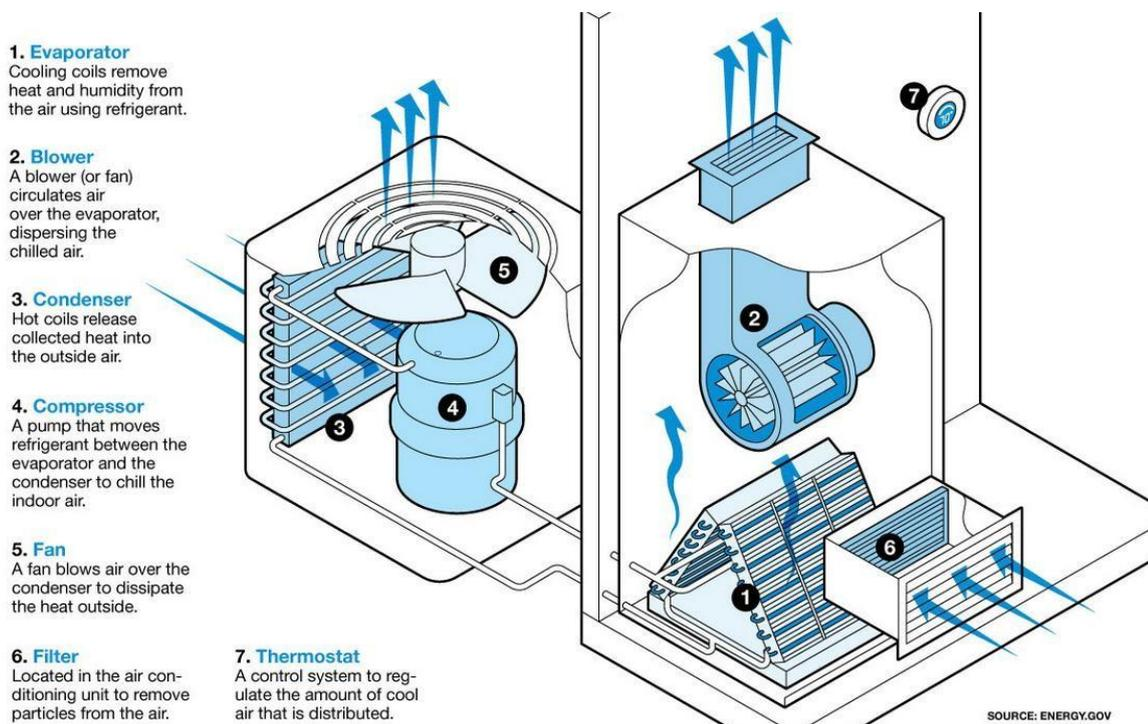
Figure 4.8 – Illustration of how an air conditioner work.
