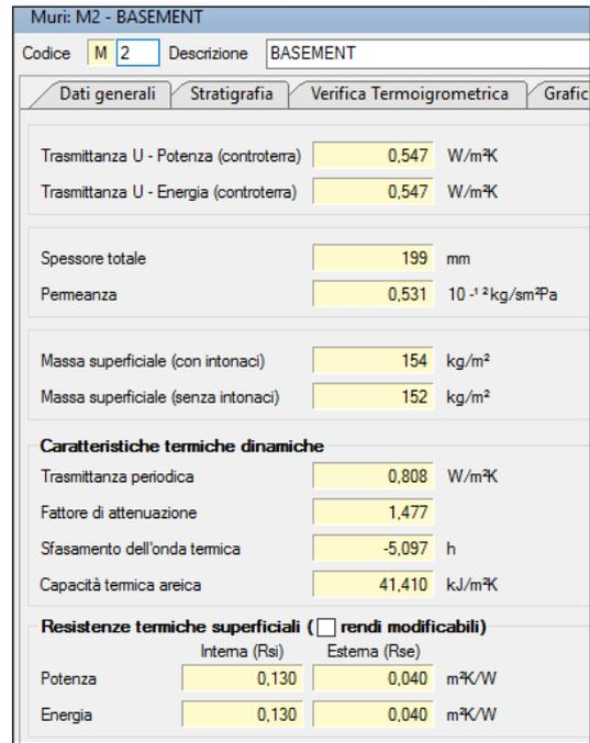
6.54 – Hygrothermal verification (left) and Transmittance value (right)
