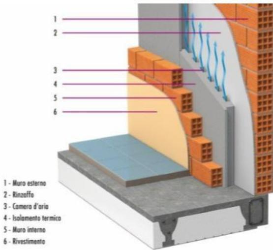
Figure 3.27 – Façade with Middle Insulation
