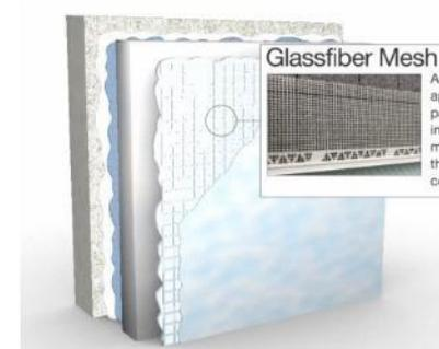
The glassfiber mash is applied to the insulation panel to reinforce its impact resistance. The mesh is embedded in the base coat.
