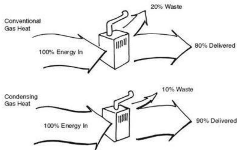
The efficiency of a fossil-fuel furnace or boiler is a measure of the amount of useful heat produced per unit of input energy (fuel). Figure 4.3
