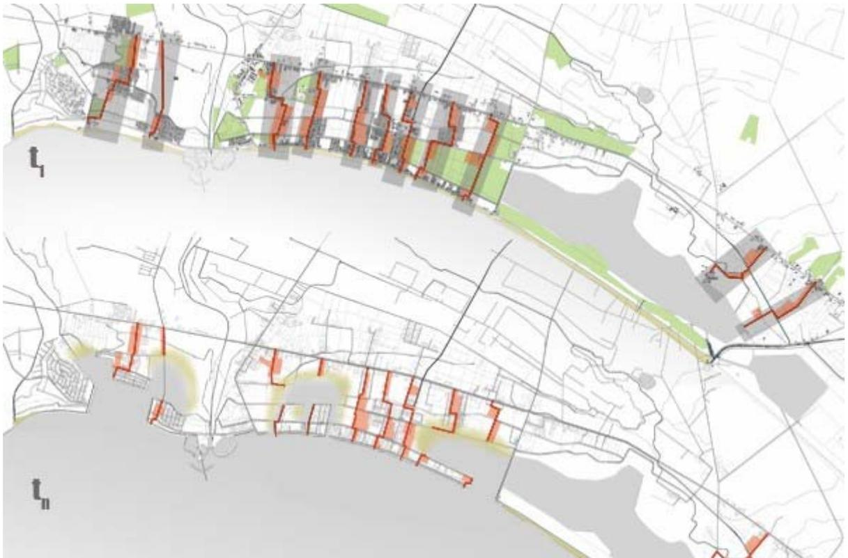
Fig.1: Transformation phases:  $t_1$  - the transformation is oriented according to directrices which are transversal to the coastline;  $t_n$  - complete erosion of the coastline and flooding of the agricultural area with the consequent birth of new beaches among agricultural fields and urban blocks
