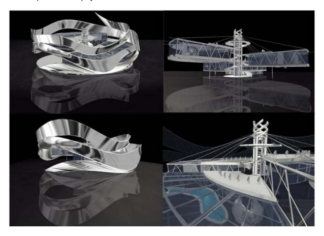
The construction is suspended above the ground by means of kevlar cables covered in carbon fiber and the exterior is made of a web of carbon profiles in carbon that support an "intelligent" camouflaged covering that changes according to the environment: transparent photovoltaic panels that project digital images and information, ETFE panels, bamboo and raw earth panels, frames with climbing plants, panels of tree bark and Hylite panels.
