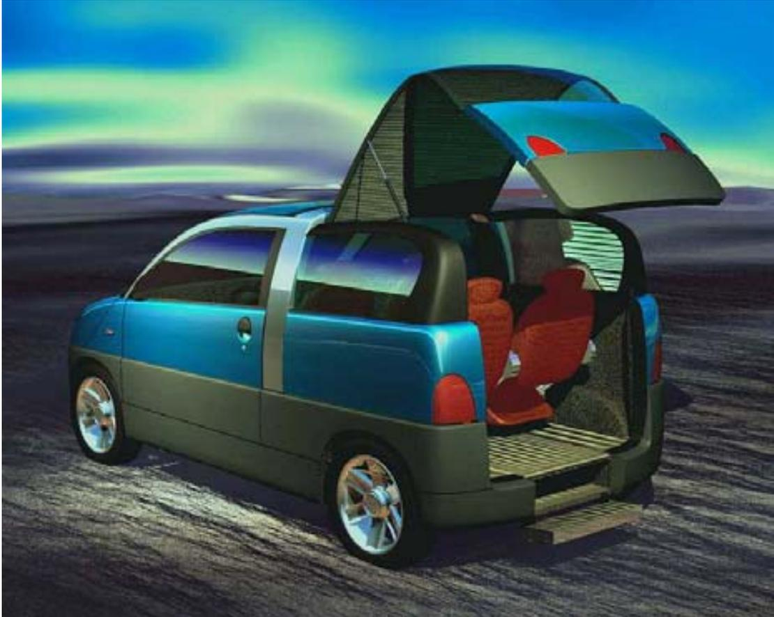
So the interiors are modular, seats are removable and the floor is level, under the floor there is a long space (about 3,80m x 0,60m) that allows you to carry a lot of objects.
