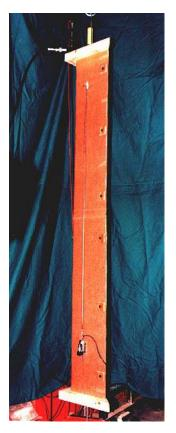
On pieces built on real scale, has been carried out on pillars compression tests on bending beams during which have been recorded the loads weight yielding and the main deformations.
