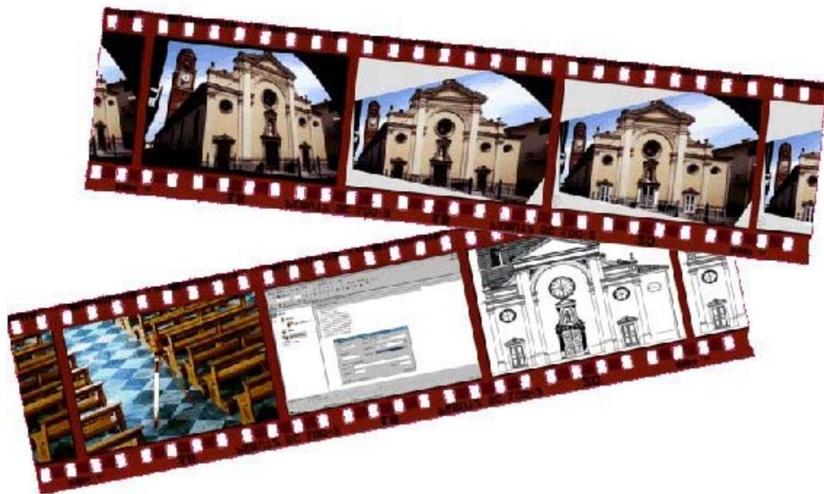
Some phases of the building survey, were done with "Fotogramma" (a software of photographic correction applied in the operations regarding the front of the building), and with interfaced total station with the computer during the phases of survey inside the church.
